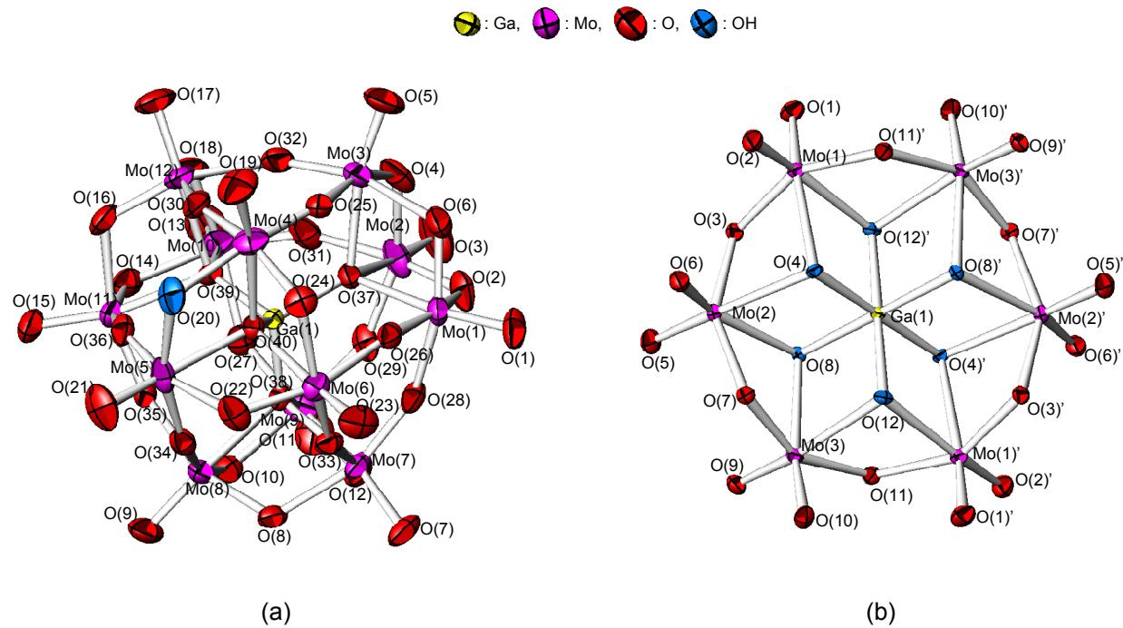
Figure S1. Structures of (a)  $[(\text{GaO}_4)\text{Mo}_{12}\text{O}_{35}(\text{OH})]^{4-}$ ; (b)  $[\text{Ga}(\text{OH})_6\text{Mo}_6\text{O}_{18}]^{3-}$ .
