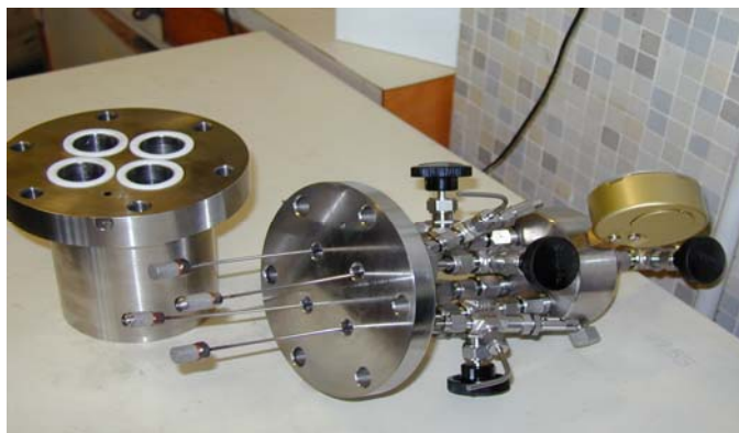
Figure S3. 4XC autoclave equipped with a system for the continuous withdrawal of gaseous or liquid samples.
