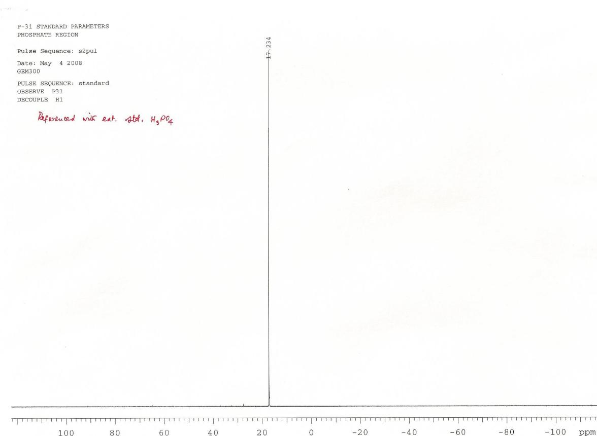
**Figure S2.** The  $^{31}P\{^1H\}$  NMR spectrum of compound **1** recorded in  $C_6D_6$  at 25 °C.
