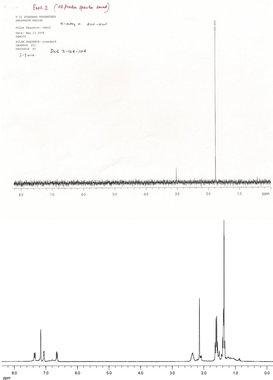
**Figure S3.** The addition of  $B_2\text{cat}_2$  and complex  $(\text{PNP})\text{Ni(O}^t\text{Bu)} (\mathbf{1})$  monitored by  $^{31}\text{P}\{\text{H}\}$  (top) and  $^1\text{H}$  (bottom) NMR in  $C_6\text{D}_6$  at 25 °C. The dominant resonance corresponds to **1** and the minor resonance at ~30 ppm is the intermediate.
