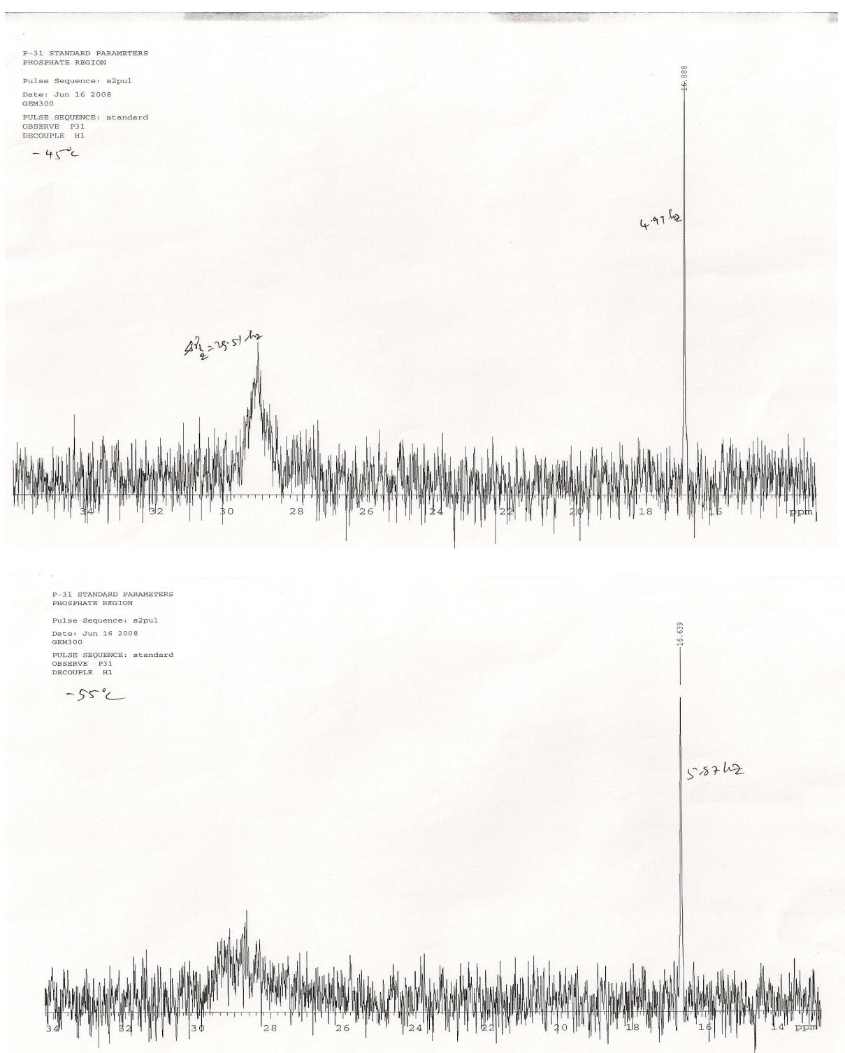
**Figure S7.** The reaction of  $\text{B}_2\text{cat}_2$  and complex  $(\text{PNP})\text{Ni}(\text{O}^t\text{Bu})$  (**1**) monitored by  $^{31}\text{P}\{^1\text{H}\}$  NMR in  $\text{C}_6\text{D}_6$  at  $-45^\circ\text{C}$  (**top**) and at  $-55^\circ\text{C}$  (**bottom**). The broad peak at  $\sim 30$  ppm corresponds to the intermediate and has broadened at lower temperature compared to the room temperature recording.
