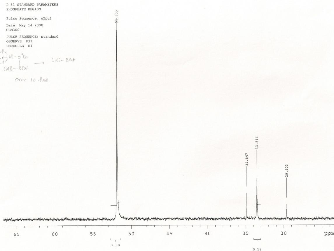
**Figure S6.** The reaction of  $\text{B}_2\text{cat}_2$  and complex  $(\text{PNP})\text{Ni}(\text{O}^t\text{Bu})$  (**1**) monitored by  $^{31}\text{P}\{^1\text{H}\}$  NMR in  $\text{C}_6\text{D}_6$  at  $25^\circ\text{C}$ . After 10 h, the intermediate has converted mostly to the product **3**, which is at  $\sim 52$  ppm. However, there are unidentified minor side products at 33 and 35 ppm.
