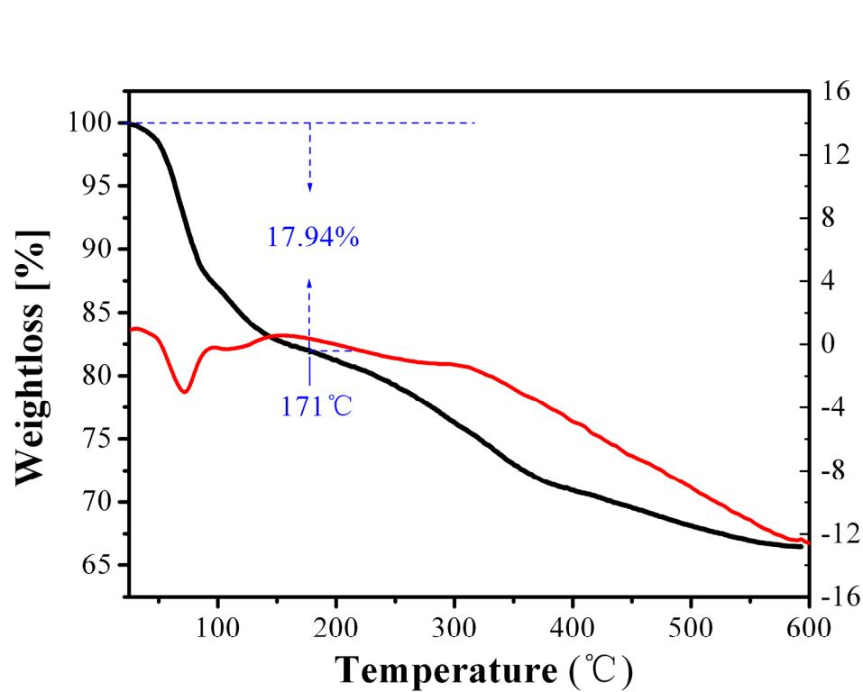
**Figure S13.** The TG curve of **1** exhibits two weight loss stages in the temperature ranges 20-600°C. The first weight loss is 17.95% in the temperature range 20-171°C, corresponding to the release of all the NH<sub>4</sub><sup>+</sup> ions, lattice and coordinated water molecules in **1** (18.05%). And after 171°C, polyoxoanion **1** would be decomposed.
