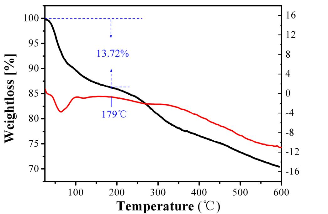
**Figure S14.** The TG curve of **2** exhibits two weight loss stages in the temperature ranges 20-600°C. The first weight loss is 13.72% in the temperature range 20-179°C, corresponding to the release of all the NH<sub>4</sub><sup>+</sup> ions and lattice water molecules in **2** (13.87%). And after 179°C, polyoxoanion **2** would be decomposed.
