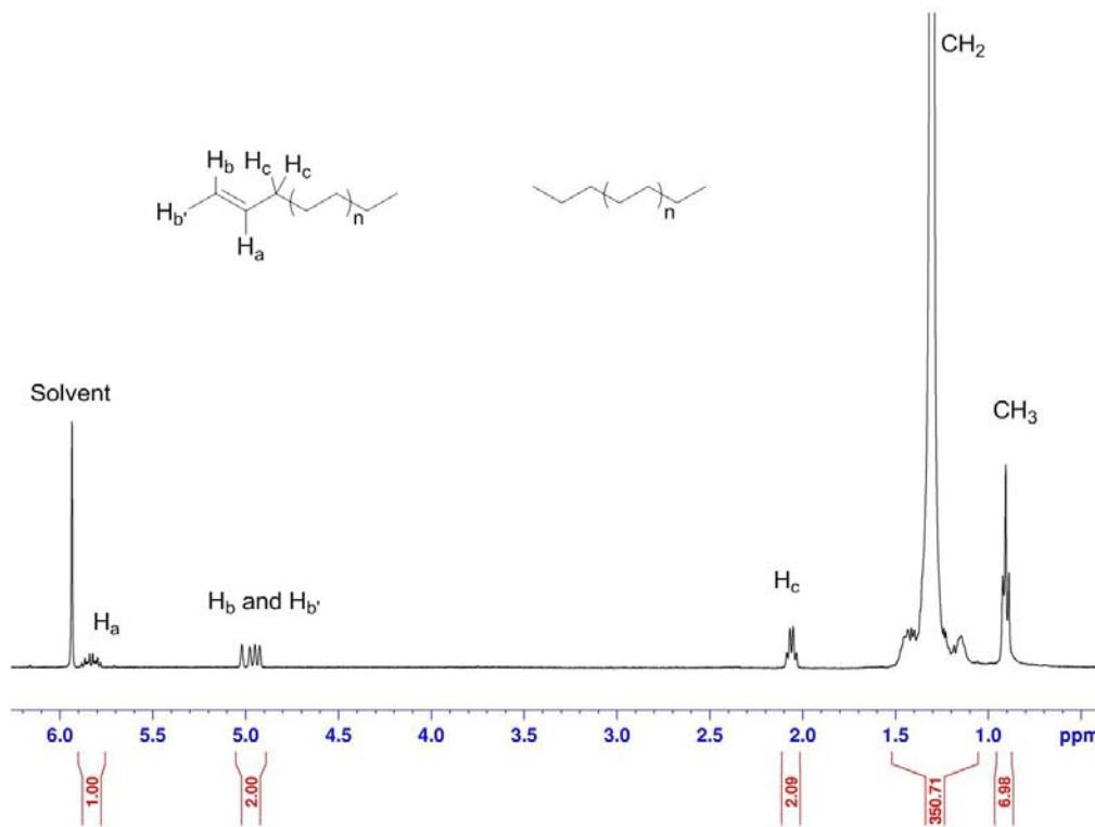
**Fig. S17** <sup>1</sup>H NMR spectrum of polyethylene obtained by using **2b** and Et<sub>3</sub>Al (listed in Table 2, entry 8).
