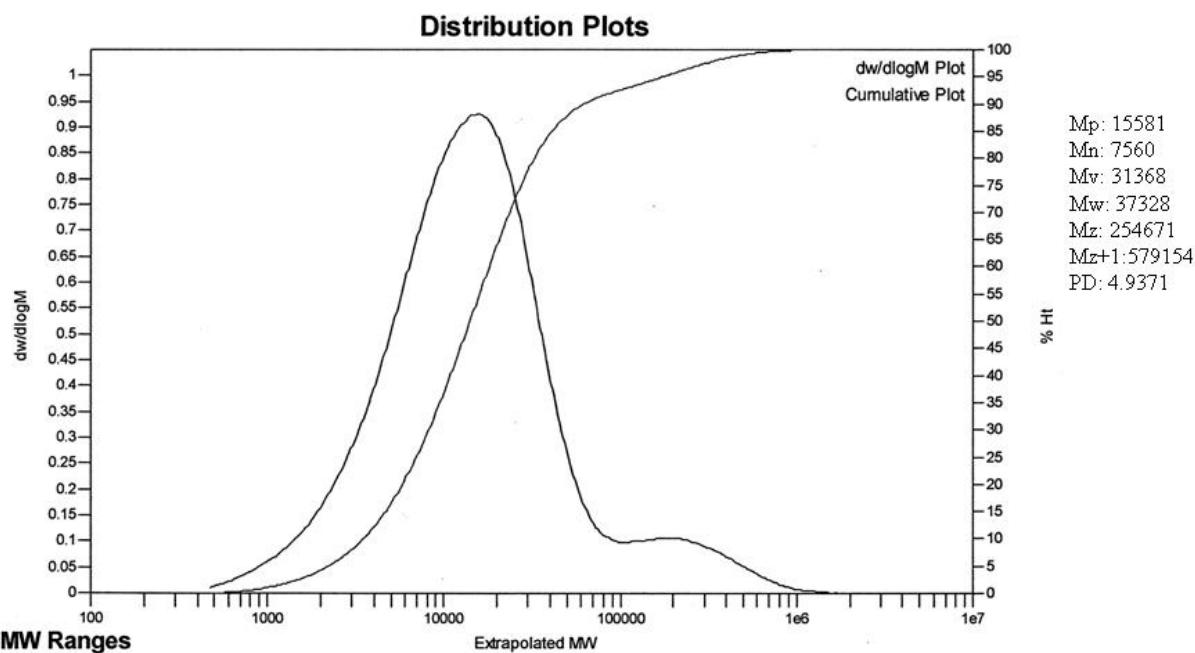
**Fig. S27** GPC trace of the polyethylene (listed in Table 2, entry 3).
