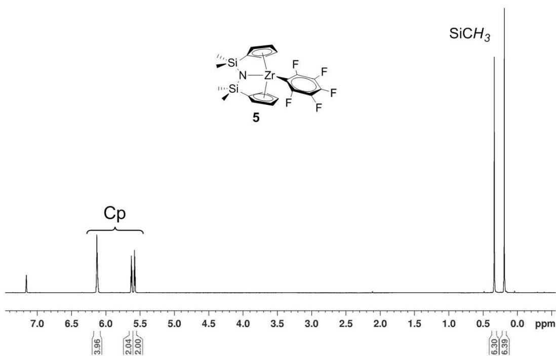
Fig. S6 <sup>1</sup>H NMR spectrum of **5** ((400 MHz, C<sub>6</sub>D<sub>6</sub>, 298 K).
