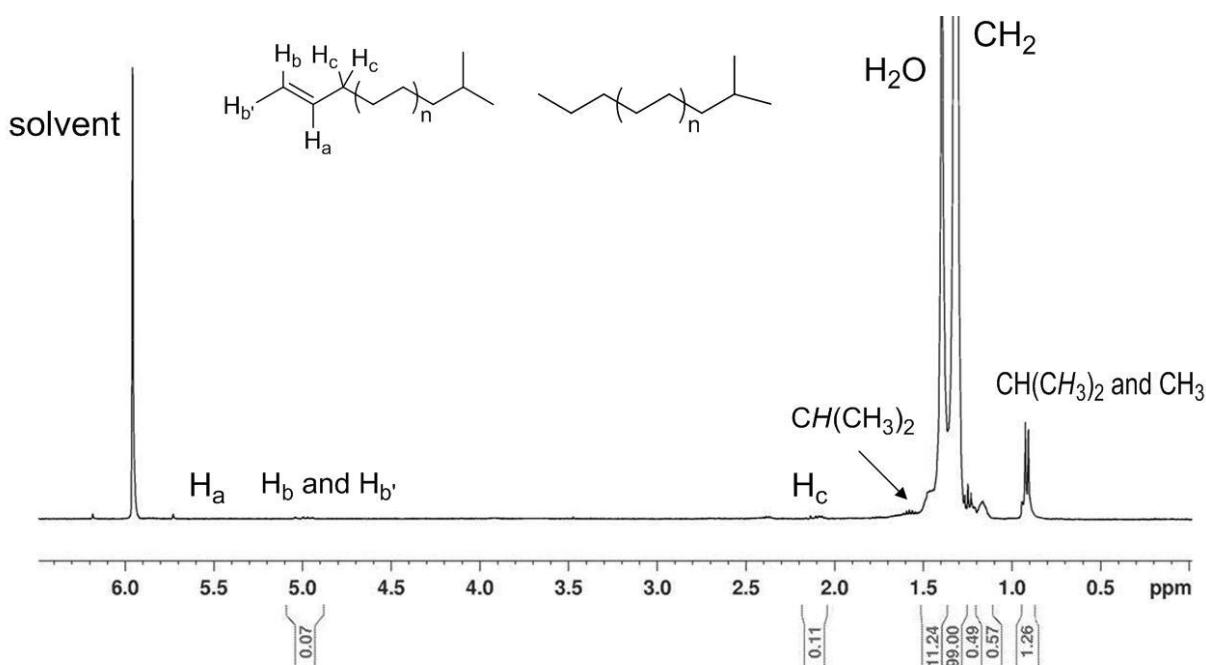
**Fig. S12** <sup>1</sup>H NMR spectrum of polyethylene obtained by using **2a** and (i-Bu)<sub>3</sub>Al (listed in Table 2, entry 4).
