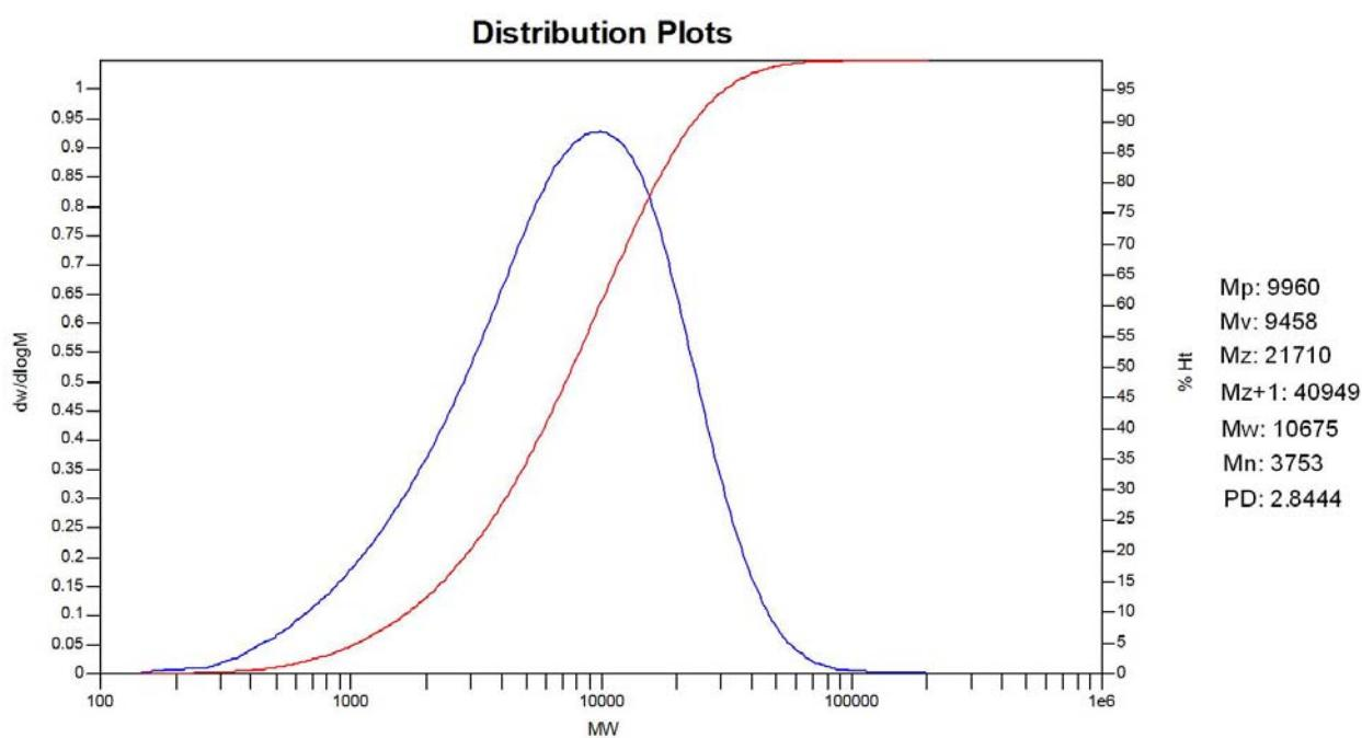
**Fig. S33.** GPC trace of the polyethylene (listed in Table 2, entry 9).
