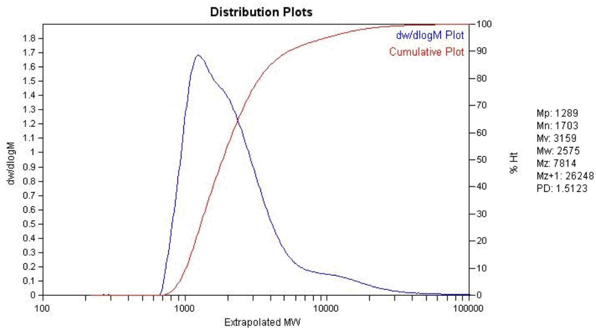
**Fig. S36** GPC trace of the copolymer of ethylene with 1-octene using **1** and MAO.
