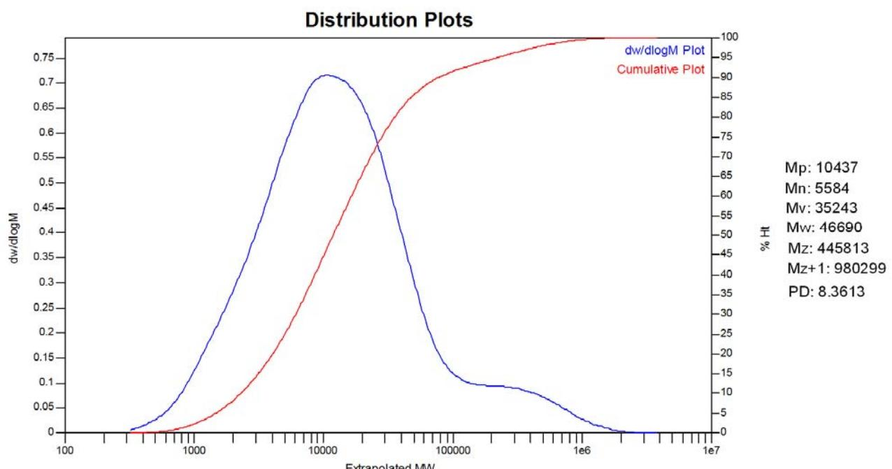
**Fig. S26** GPC trace of the polyethylene (listed in Table 2, entry 2).
