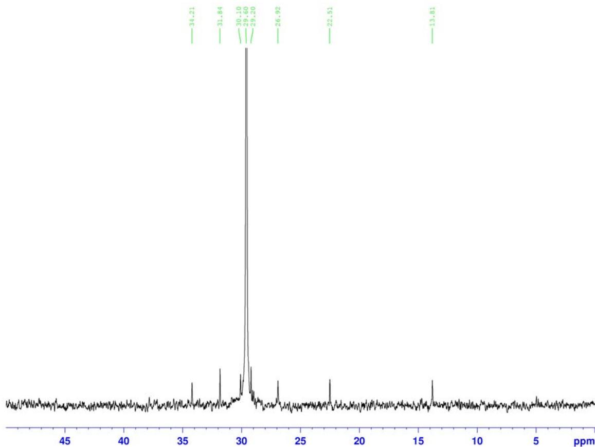
**Fig. S16** <sup>13</sup>C NMR spectrum of polyethylene obtained by using **2b** and Et<sub>3</sub>Al (listed in Table 2, entry 7).
