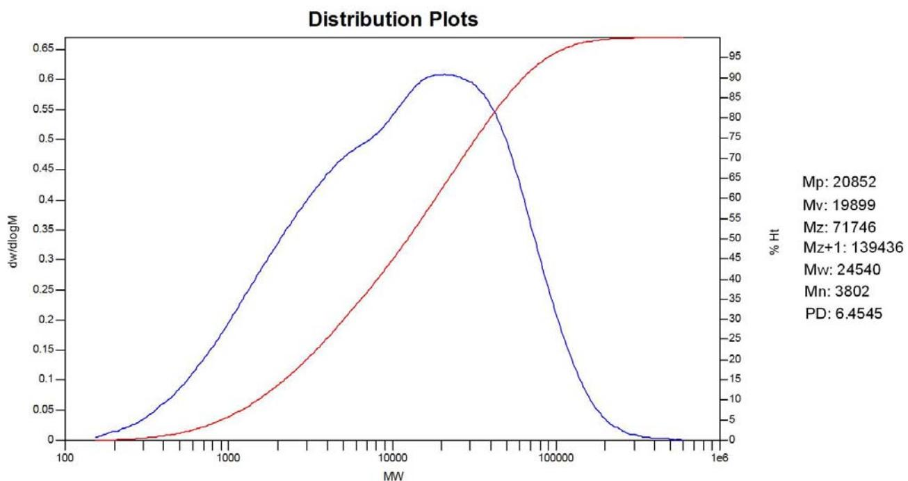
**Fig. S37** GPC trace of the copolymer of ethylene with 1-octene using **2b** and Et<sub>3</sub>Al.
