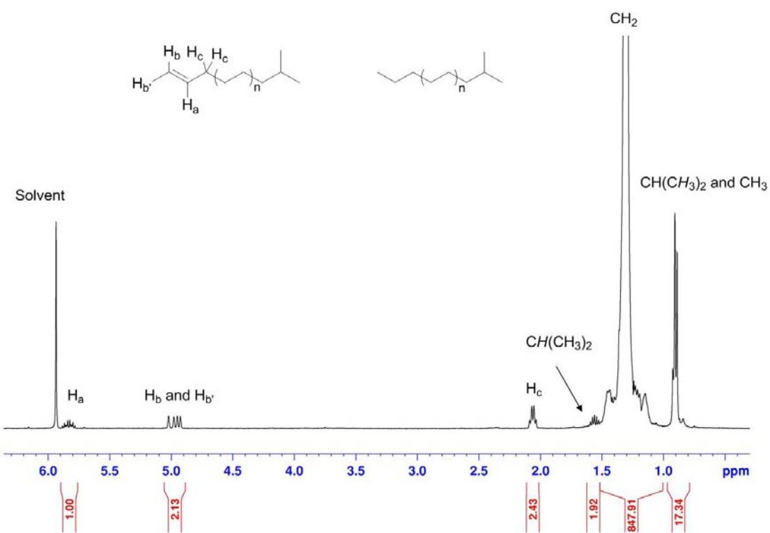
**Fig. S13** <sup>1</sup>H NMR spectrum of polyethylene obtained by using **2b** and (i-Bu)<sub>3</sub>Al (listed in Table 2, entry 5).
