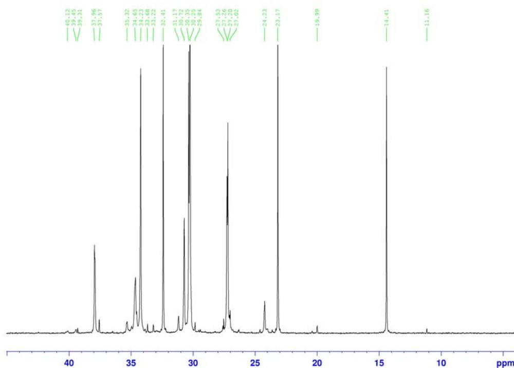
**Fig. S24**  $^{13}\text{C}$  NMR spectrum of the copolymer of ethylene with 1-octene using **2b** and Et<sub>3</sub>Al (100 MHz, benzene-*d*<sub>6</sub>, 298 K).
