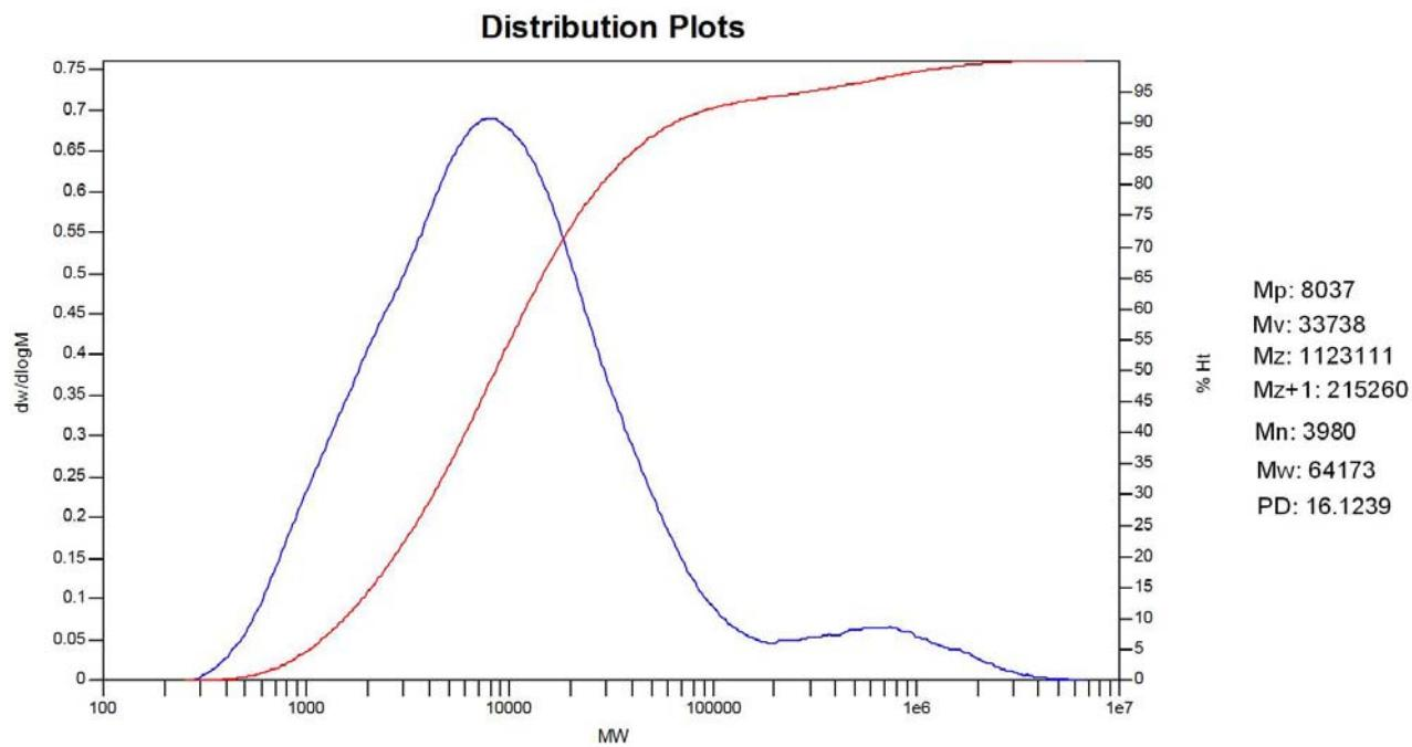
**Fig. S32.** GPC trace of the polyethylene (listed in Table 2, entry 8).
