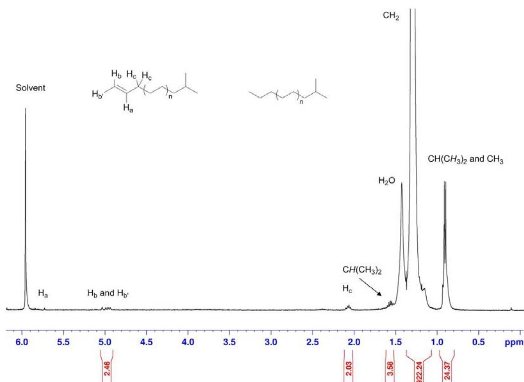
**Fig. S10** <sup>1</sup>H NMR spectrum of polyethylene obtained by using **3a** and (i-Bu)<sub>3</sub>Al (listed in Table 2, entry 2).
