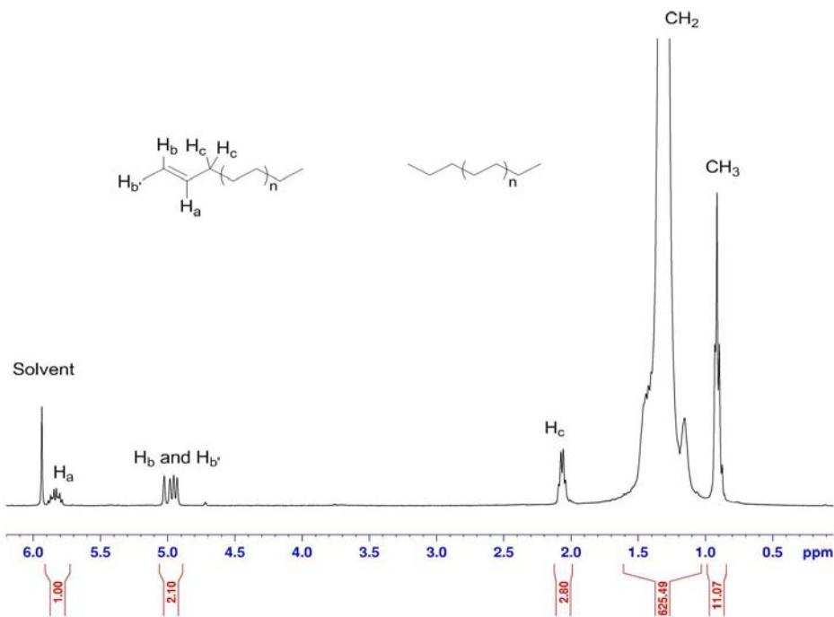
**Fig. S15** <sup>1</sup>H NMR spectrum of polyethylene obtained by using **2b** and Et<sub>3</sub>Al (listed in Table 2, entry 7).
