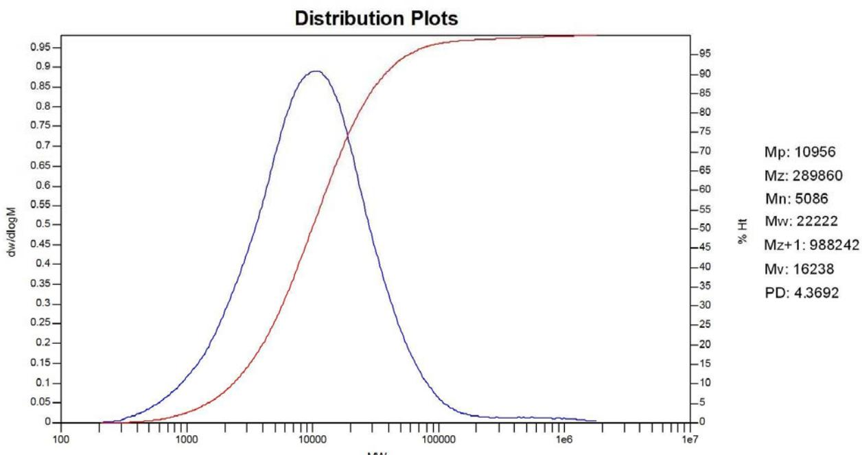
**Fig. S29** GPC trace of the polyethylene (listed in Table 2, entry 5).
