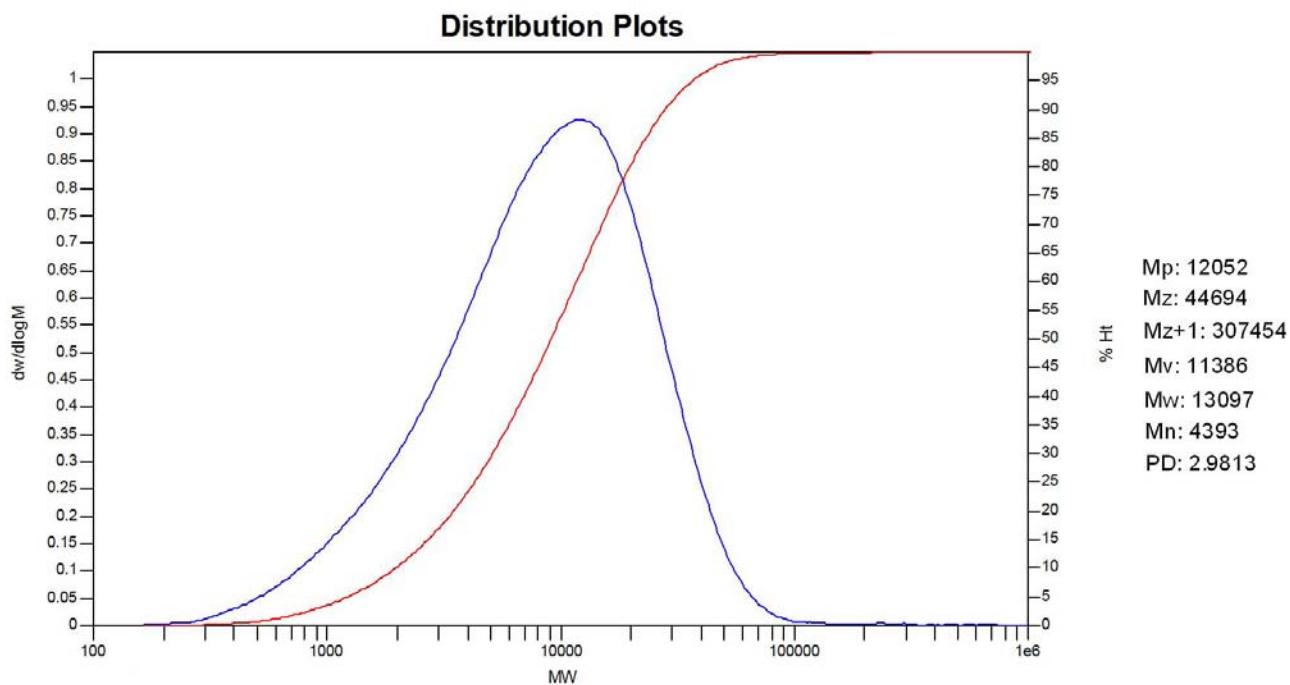
**Fig. S31** GPC trace of the polyethylene (listed in Table 2, entry 7).
