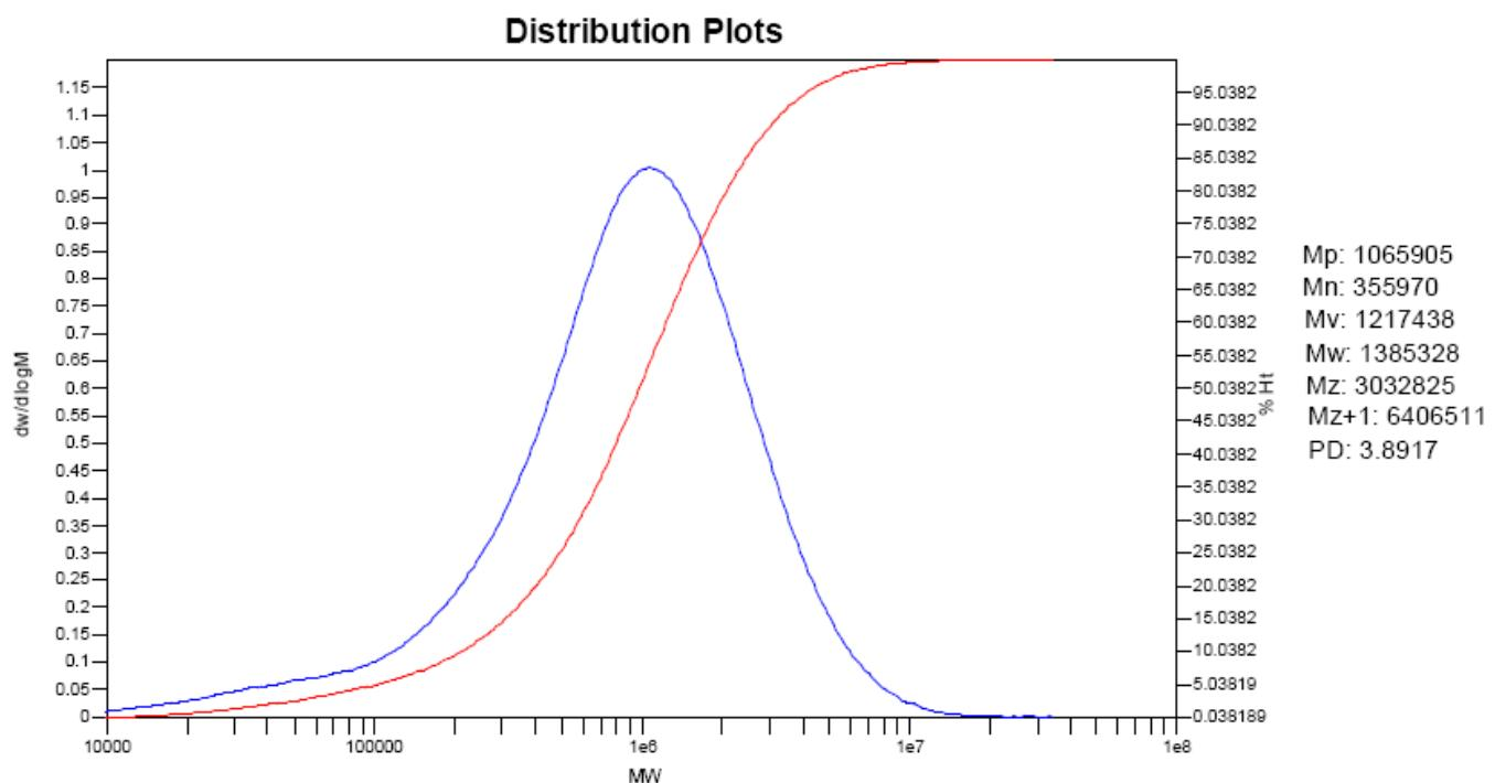
**Fig. S34** GPC trace of the polyethylene (listed in Table 2, entry 10).
