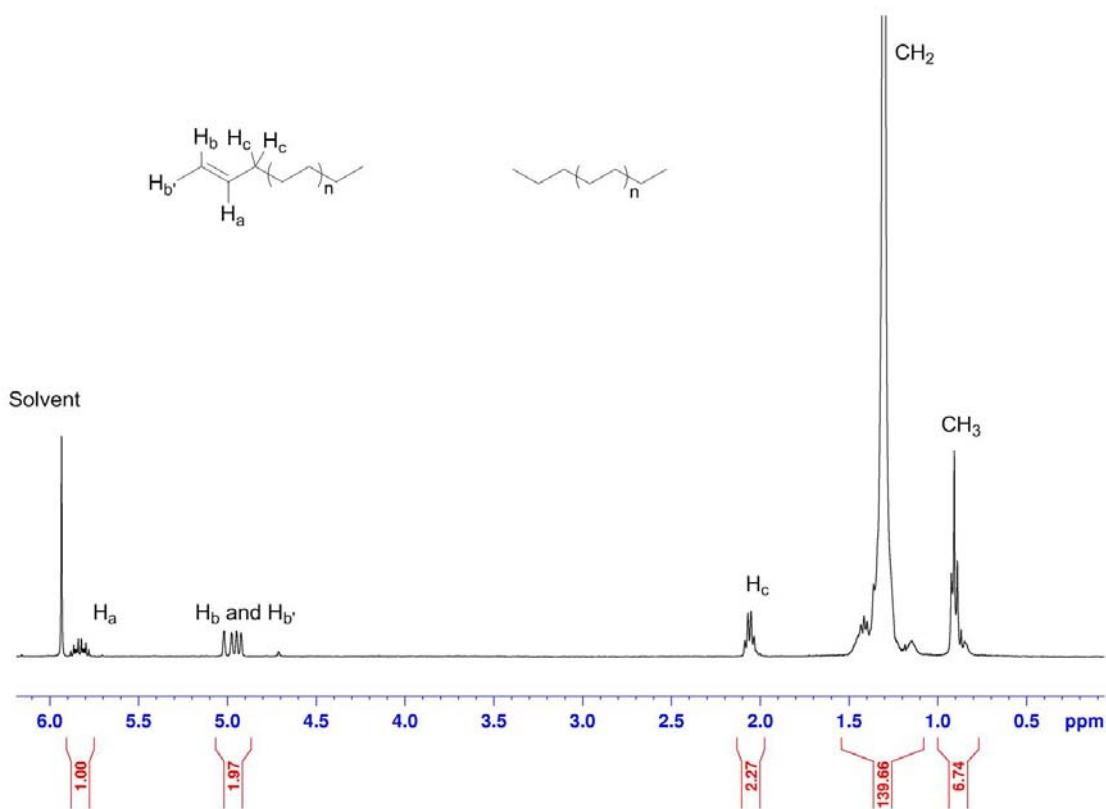
**Fig. S14** <sup>1</sup>H NMR spectrum of polyethylene obtained by using **2b** and Me<sub>3</sub>Al (listed in Table 2, entry 6).
