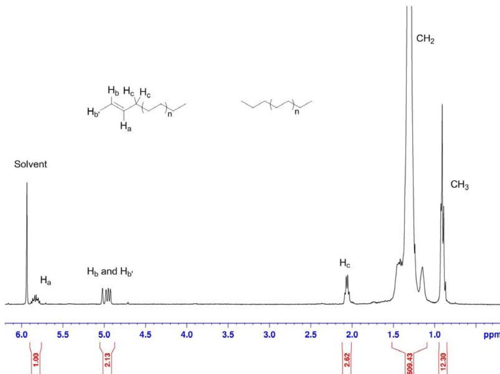
**Fig. S18** <sup>1</sup>H NMR spectrum of polyethylene obtained by using **2b** and Et<sub>3</sub>Al (listed in Table 2, entry 9).
