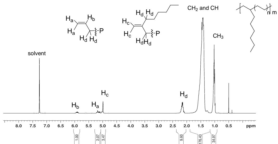
**Fig. S21**  $^1\text{H}$  NMR spectrum of the copolymer of ethylene with 1-octene using **1** and MAO (400 MHz, benzene- $d_6$ , 298 K)
