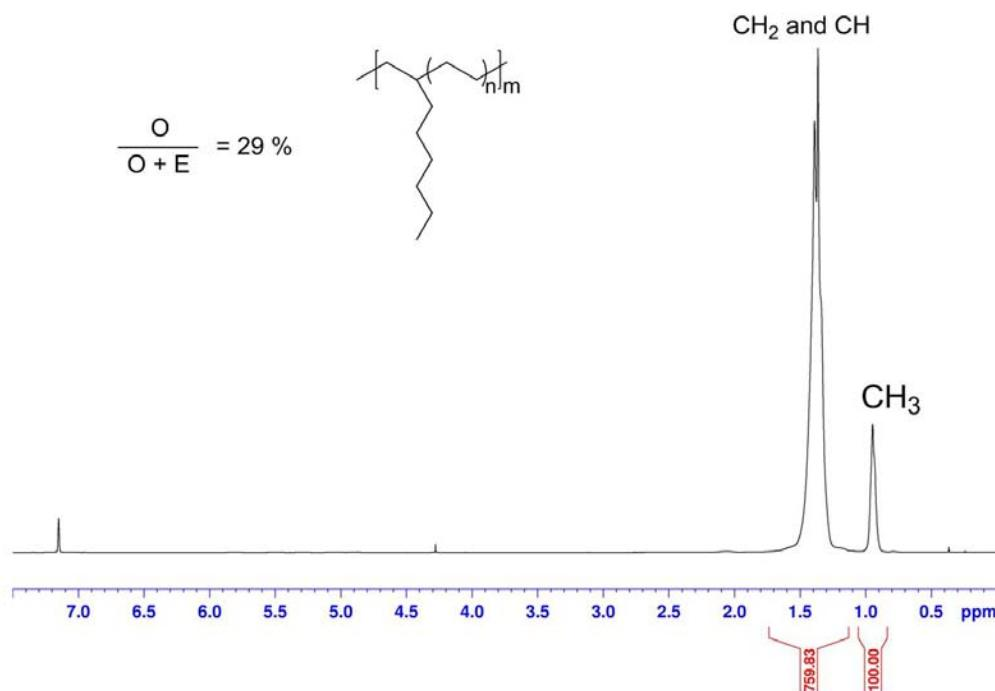
**Fig. S23**  $^1\text{H}$  NMR spectrum of the copolymer of ethylene with 1-octene using **2b** and Et<sub>3</sub>Al (100 MHz, benzene-*d*<sub>6</sub>, 298 K).
