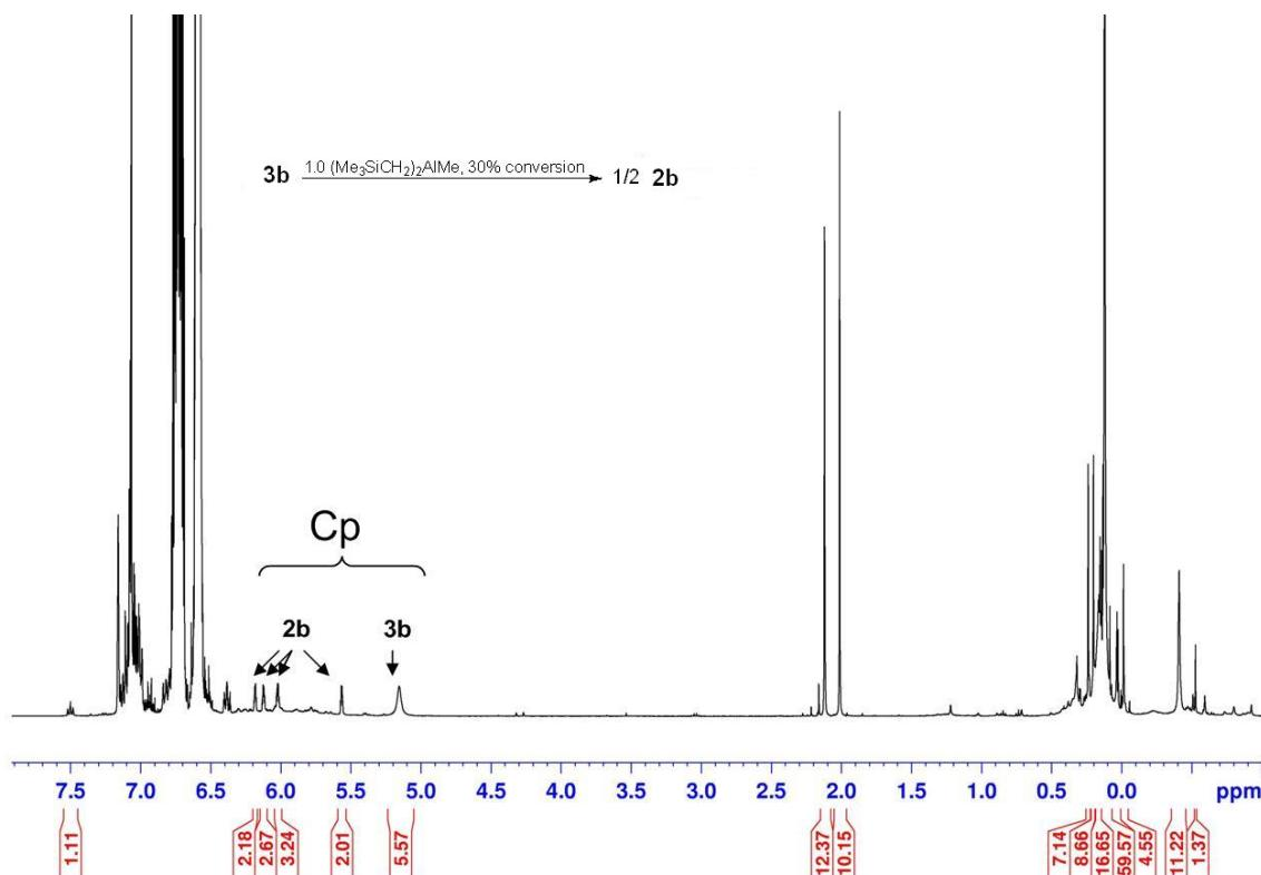
Fig. S7 <sup>1</sup>H NMR monitoring of the reaction of **3b** with 1 equiv of (Me<sub>3</sub>SiCH<sub>2</sub>)<sub>2</sub>AlMe in situ, about 30% conversion rate to **2b** was obtained ((400 MHz, C<sub>6</sub>D<sub>6</sub>/1,2-C<sub>6</sub>H<sub>4</sub>F<sub>2</sub>, 298 K).
