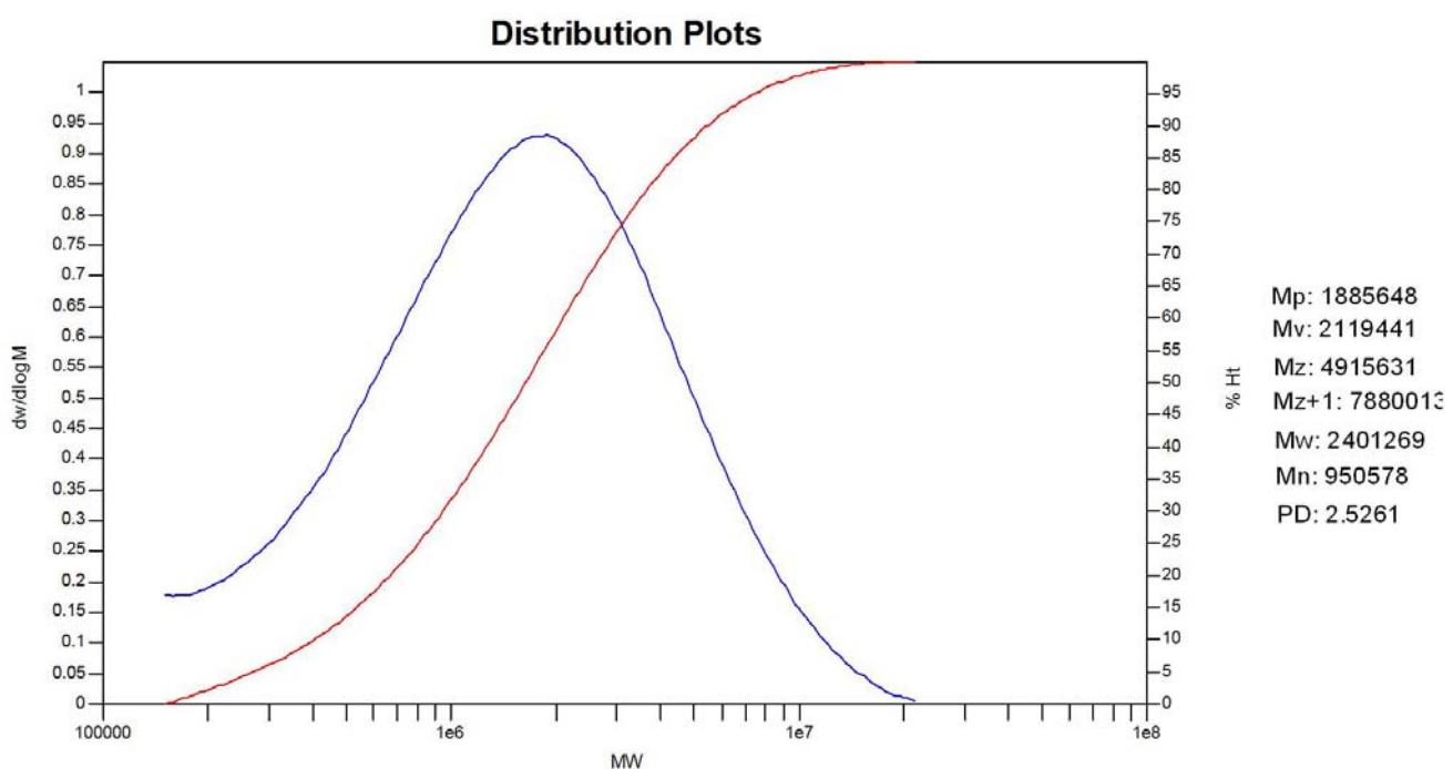
**Fig. S35** GPC trace of the polyethylene (listed in Table 2, entry 11).
