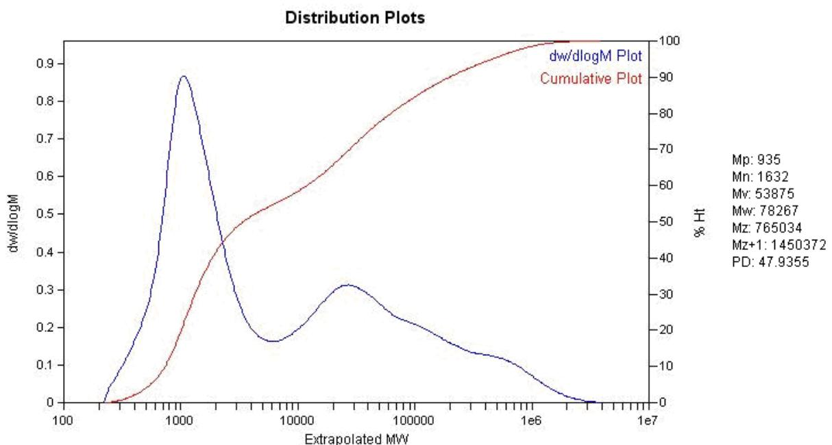
**Fig. S25** GPC trace of the polyethylene (Table 2, entry 1).
