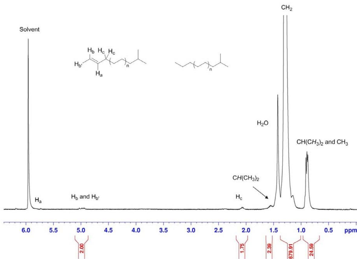
**Fig. S11** <sup>1</sup>H NMR spectrum of polyethylene obtained by using **3b** and (i-Bu)<sub>3</sub>Al (listed in Table 2, entry 2).
