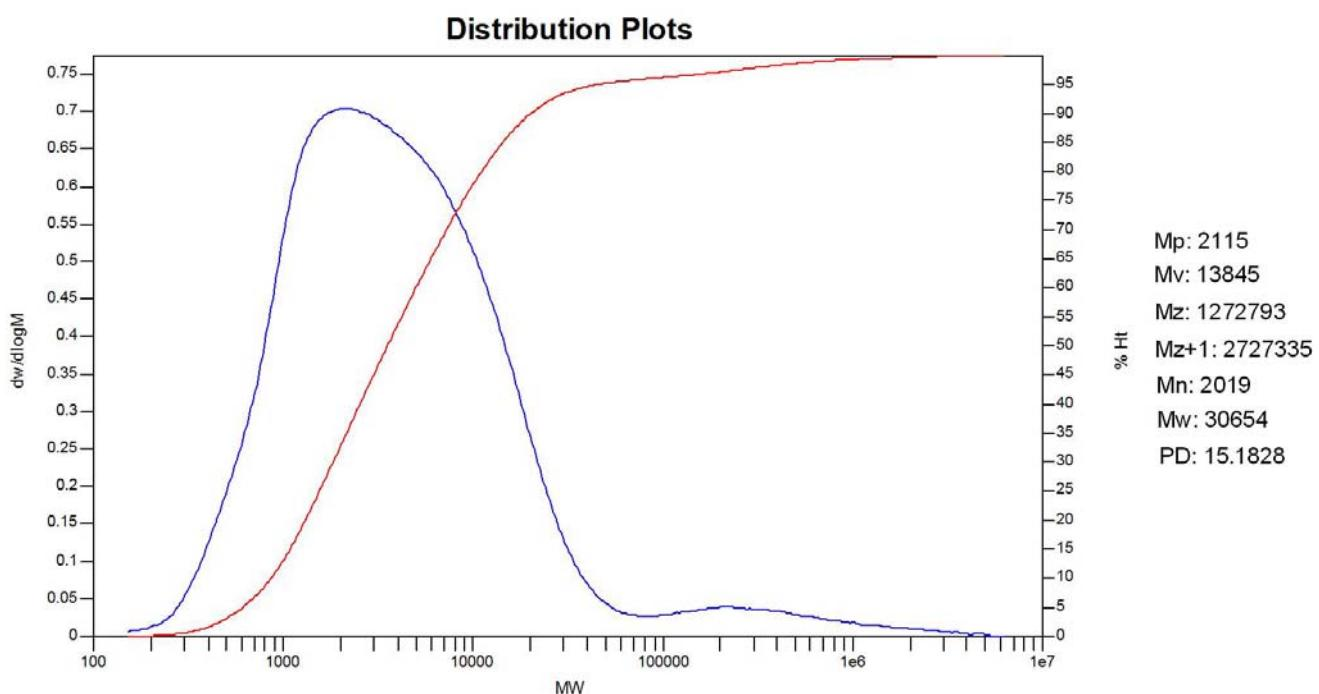
**Fig. S30.** GPC trace of the polyethylene (listed in Table 2, entry 6).
