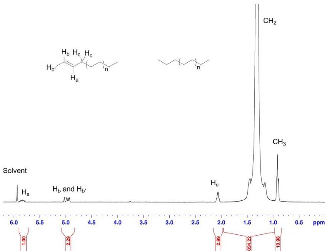
**Fig. S20** <sup>1</sup>H NMR spectrum of polyethylene obtained by using **2b** and Me<sub>3</sub>Al (listed in Table 2, entry 11).
