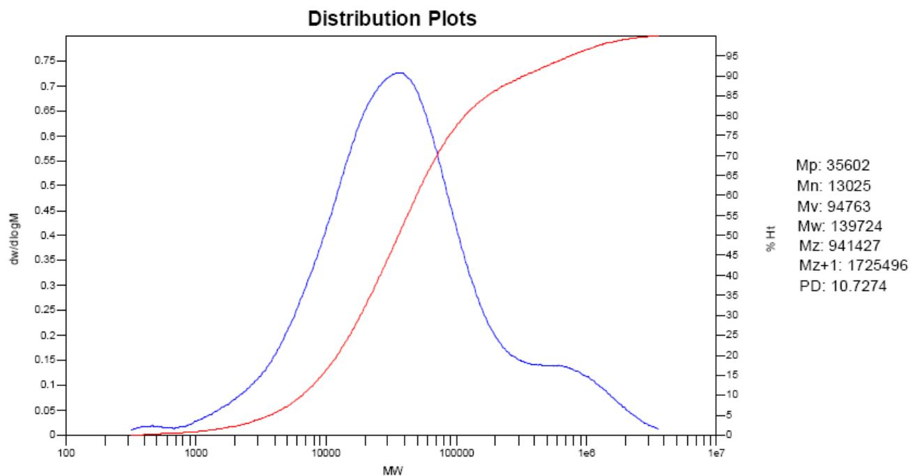
**Fig. S28** GPC trace of the polyethylene (listed in Table 2, entry 4).
