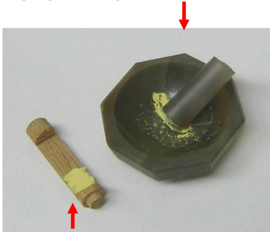
An insert (oak wood) that was placed into the cuvette holder for solid state fluorescence measurements. Oak wood was chosen because of its own low light reflectivity and good adhesion to the tape.
