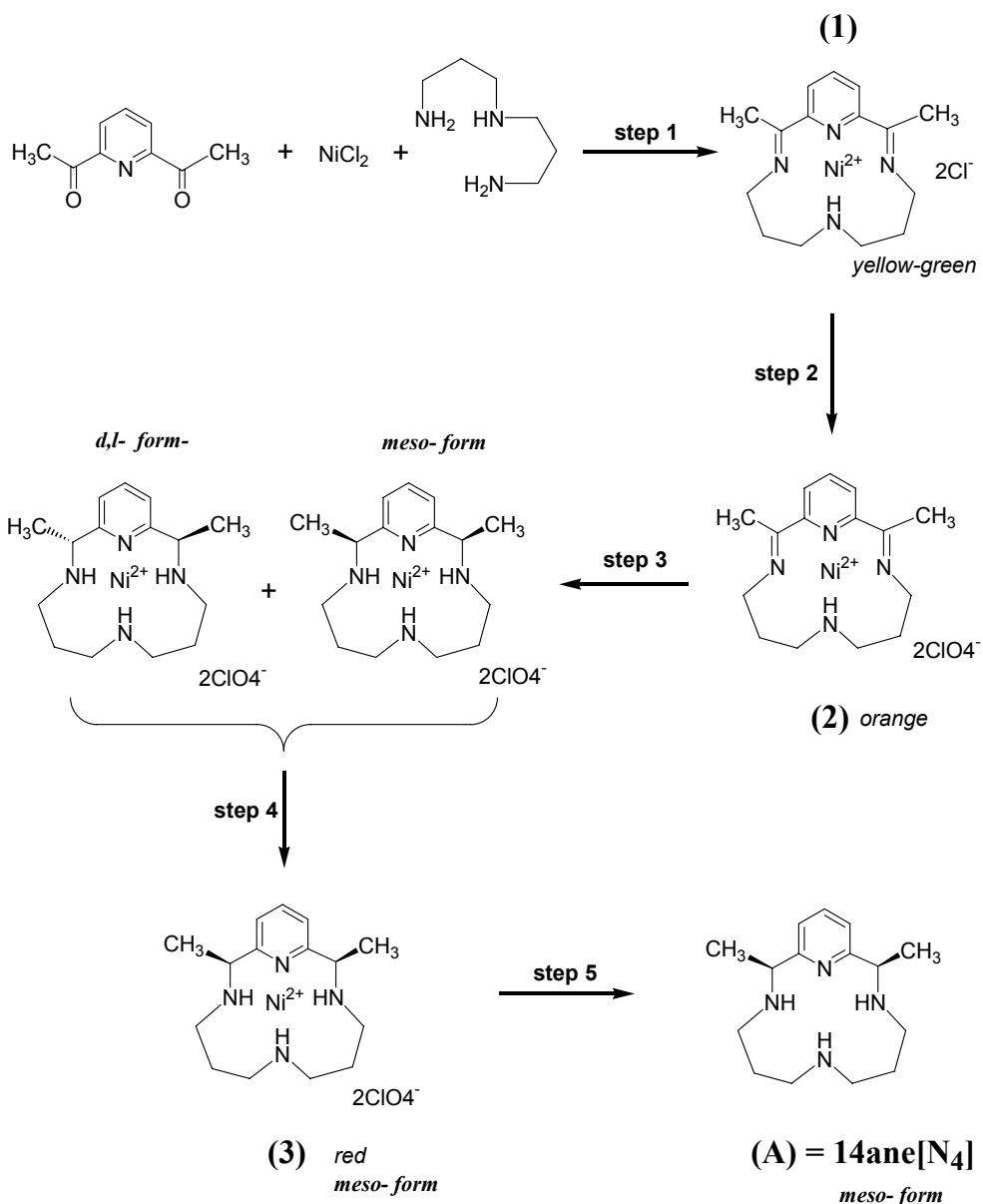
Step 1: Template condensation. Step 2: Ligand exchange reaction. Step 3: Reduction of the ligand in complex **3**. Step 4: Separation of the two reduced isomeric Ni(II) macrocyclic complexes by multistep crystallization. Step 5: Demetallation reaction.
