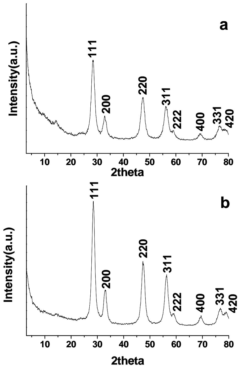
Figure S4. XRD patterns of (a) ceria nanofibers , (b) ceria 3D-macroporous foam.
