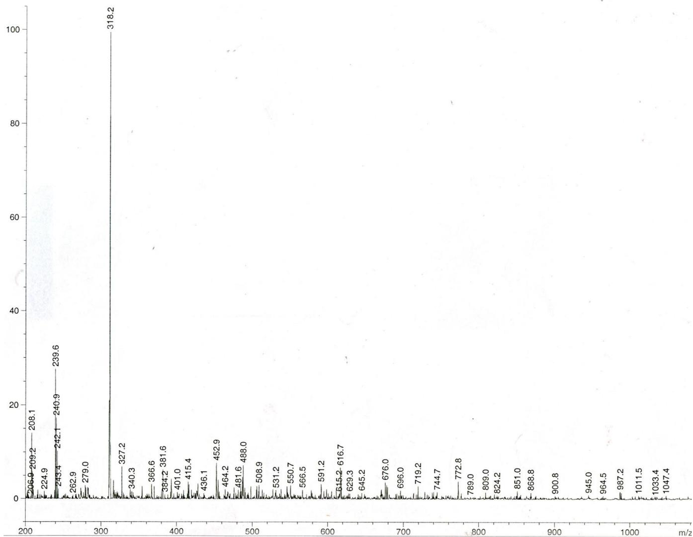
**Fig. S2** Mass spectrum of complex **2** in aqueous DMF (1:1 v/v) showing the parent ion peak at 318.20 m/z.
