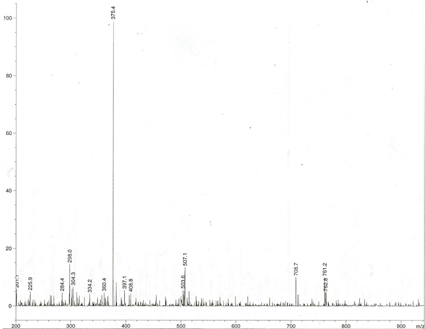
**Fig. S3** Mass spectrum of complex **3** in aqueous DMF (1:1 v/v) showing the parent ion peak at 375.47 m/z.
