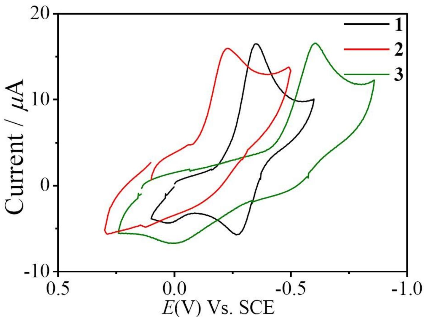
**Fig. S11** Cyclic voltammetric responses for the complexes **1** (black), **2** (red), **3** (green) in DMF using TBAP (0.1 M) as the supporting electrolyte with a scan rate of  $50 \text{ mV s}^{-1}$ .
