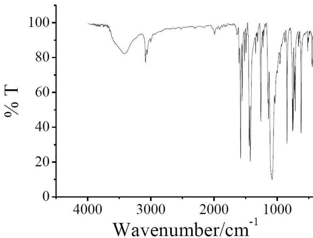
**Fig. S4** IR spectrum of complex **1** in solid KBr matrix.
