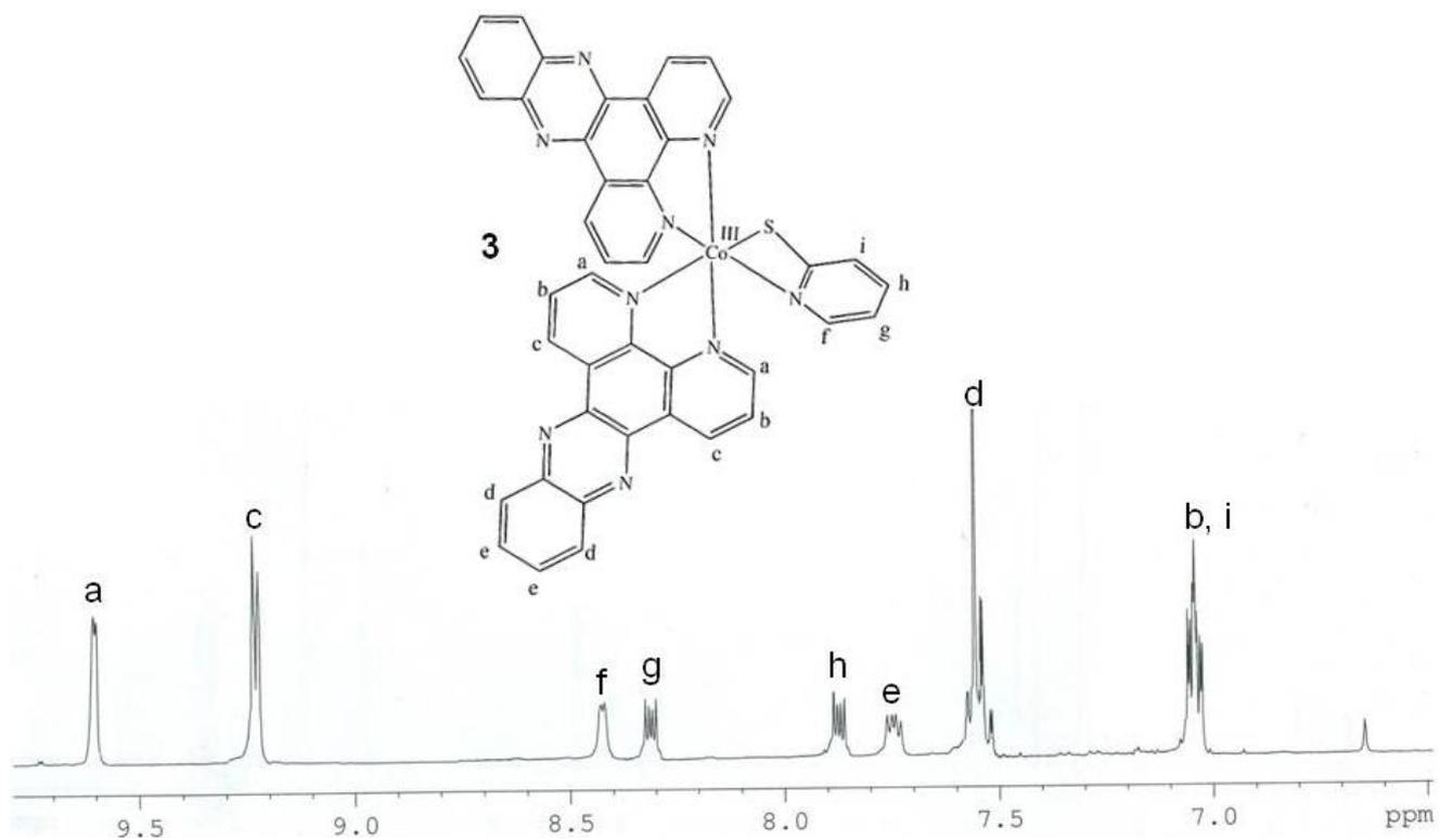
**Fig. S9** NMR spectrum of complex **3** in DMSO-d<sub>6</sub> showing the peak assignments.
