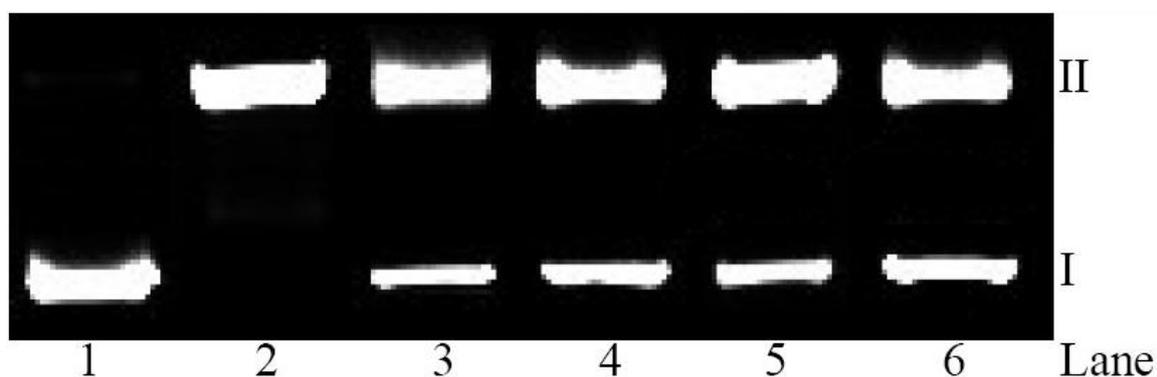
**Fig. S16** Cleavage of SC pUC19 DNA (0.2  $\mu$ g, 30  $\mu$ M) by the complex **3** (20  $\mu$ M, 2 h) in the presence of various additives on photo-irradiation at 647.1 nm under argon atmosphere in 50 mM Tris-HCl/NaCl buffer (pH, 7.2) for 1 h incubation time [ $\text{NaN}_3$ , 200  $\mu$ M; catalase, 4 units; DMSO, 4  $\mu$ L]. Form I and II are supercoiled and nicked circular forms of DNA, respectively.
