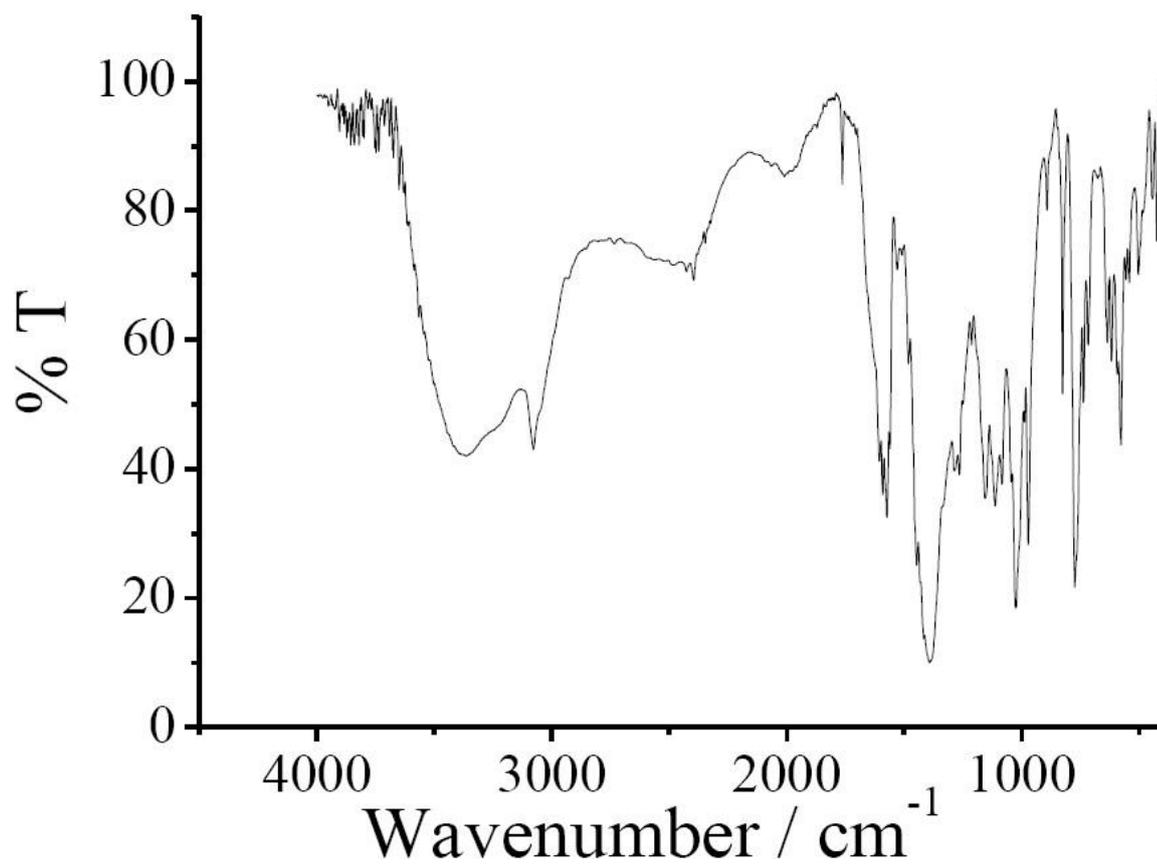
**Fig. S5** IR spectrum of complex **2** in solid KBr matrix.
