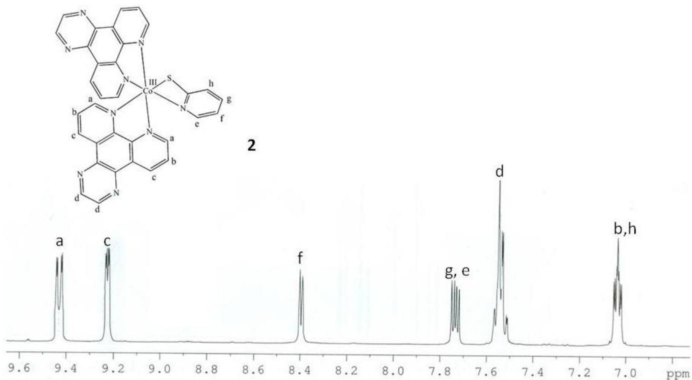
**Fig. S8** NMR spectrum of complex **2** in DMSO-d<sub>6</sub> showing the peak assignments.
