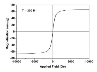
Fig. S1 Magnetization-applied magnetic field of oleic acid stabilized  $Fe_3O_4$  particles at 300 K.
