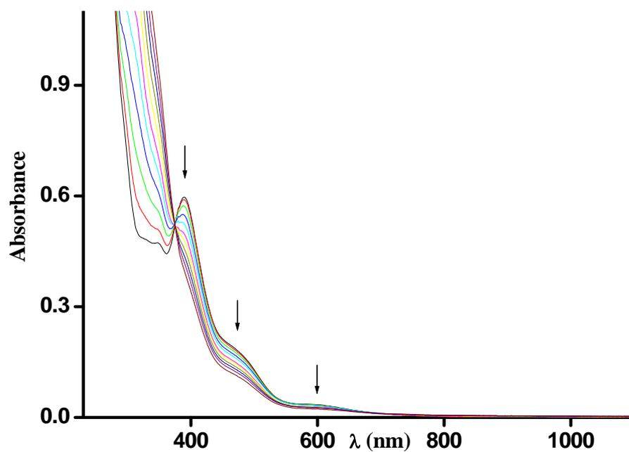
**Figure S8** Spectrochemical titration of [Cu<sup>II</sup>L] in CH<sub>2</sub>Cl<sub>2</sub> with 0-1 equivalent of Tris(4-bromophenyl) ammonium hexachloro antimonate. Arrows indicate spectral changes upon addition of oxidizer.  $T = 298\text{ K}$ ,  $l = 1.000\text{ cm}$ , [Cu<sup>II</sup>L] = 0.05 mM.
