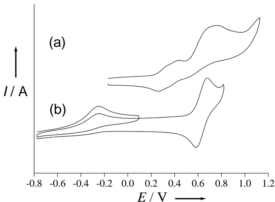
**Figure S4** CV curves of  $CH_2Cl_2$  solutions (+ 0.1 M TBAP) of the complexes (a)  $[Ni^{II}L]$ , (b)  $[Co^{II}L]$  in the presence of 0.05 M pyridine. Concentrations are 0.75 mM, and the potentials are referenced vs.  $Fc^+/Fc$ . Scan rate:  $0.1 V \cdot s^{-1}$ ,  $T = 298 K$
