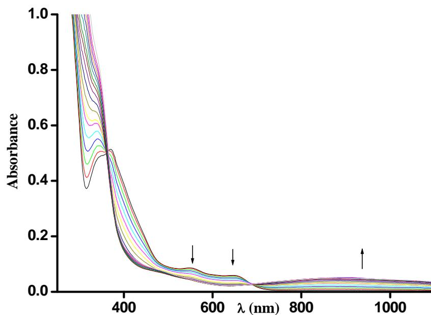
**Figure S6** Spectrochemical titration of  $[\text{Co}^{\text{II}}(\text{L})]$  with 0-2 equivalents of Tris(4-bromophenyl) ammonium hexachloro antimonate. Arrows indicate spectral changes upon addition of oxidizer.  $T = 298 \text{ K}$ ,  $l = 1.000 \text{ cm}$ ,  $[\text{Co}^{\text{II}}\text{L}] = 0.05 \text{ mM}$ .
