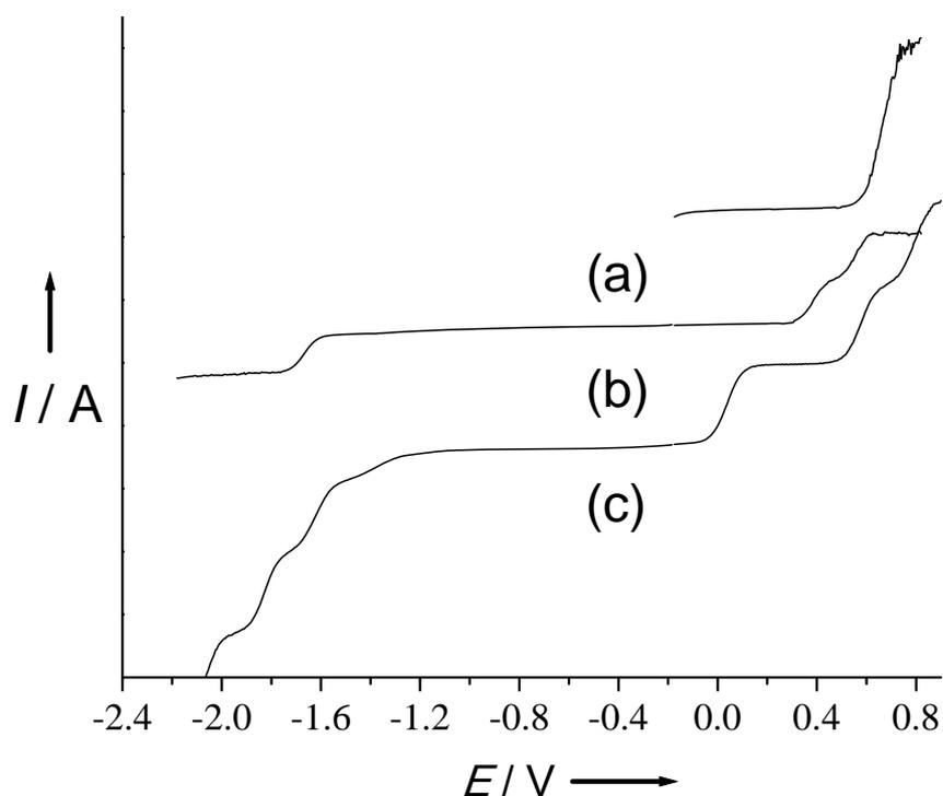
**Figure S5** RDE curves of  $CH_2Cl_2$  solutions (+ 0.1 M TBAP) of the complexes (a)  $[Zn^{II}L]$ , (b)  $[Cu^{II}L]$ , (c)  $[Co^{II}L]$ .  $T = 298 K$ . Concentrations are 0.75 mM except for  $[Cu^{II}L]$  (0.5 mM), and the potentials are referenced vs.  $Fc^+/Fc$ . Scan rate:  $0.01 V \cdot s^{-1}$  (500 rpm),  $T = 298 K$ .
