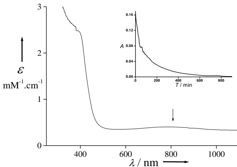
**Figure S1** Electronic spectra of the electrogenerated  $[\text{Zn}^{\text{II}}(\text{L}^{\bullet})]^{2+}$  in  $\text{CH}_2\text{Cl}_2$  (0.01 M TBAP). The insert represents the decay pattern at  $T = 298$  K.  $l = 1.000$  cm.
