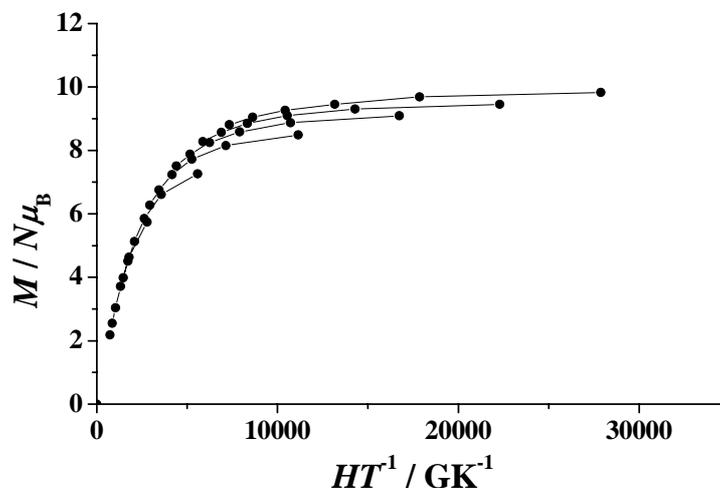
**Fig. S6** Plots of the reduced magnetization,  $M/N\mu_B$ , vs  $HT^{-1}$  for complex **1** in the field range 0-5 T. Data were measured for 1 K increments between 1.8 and 6.8 K.
