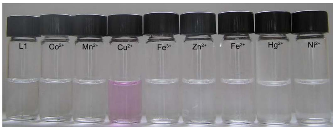
**Fig.S2** (a) Photos of color changes of **L1** (20  $\mu\text{M}$ ) upon addition of 40  $\mu\text{M}$  different metal ions in water/  $\text{CH}_3\text{CN}$  (1:1 v/v) solutions.
