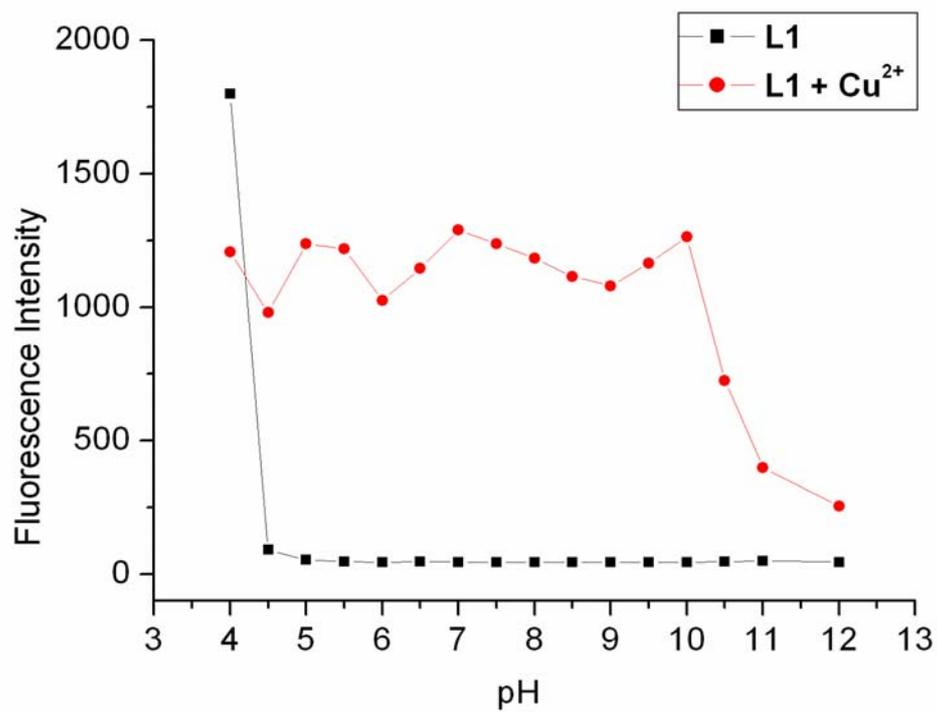
**Fig. S6** Fluorescence spectra of **1** (20  $\mu\text{M}$ ) with the addition of  $\text{Cu}^{2+}$  (30  $\mu\text{M}$ ) in water/ $\text{CH}_3\text{CN}$  (1:1 v/v) at various pH values (Ex. 495 nm; Em. 552 nm).
