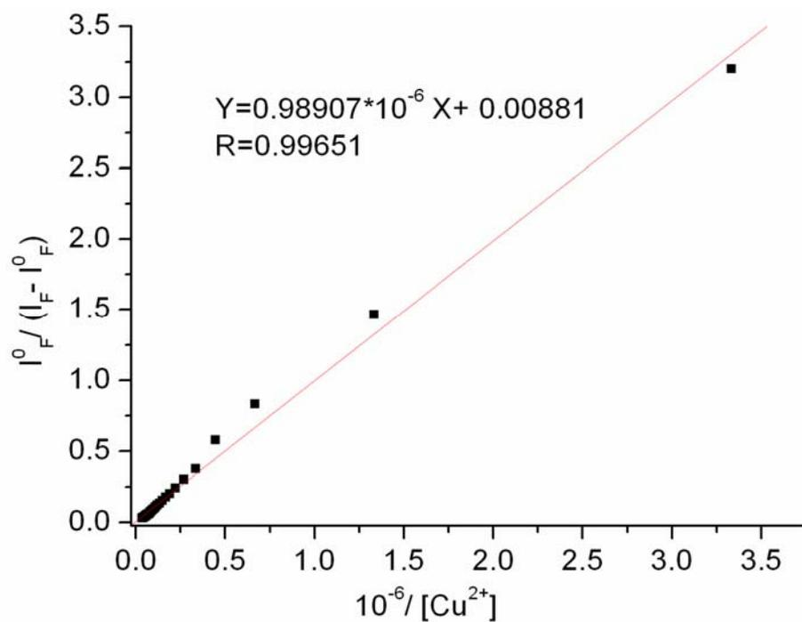
**Fig. S3** Fitting of Fluorescence titration curve of **L1** in water/  $\text{CH}_3\text{CN}$  (1:1 v/v) solution.
