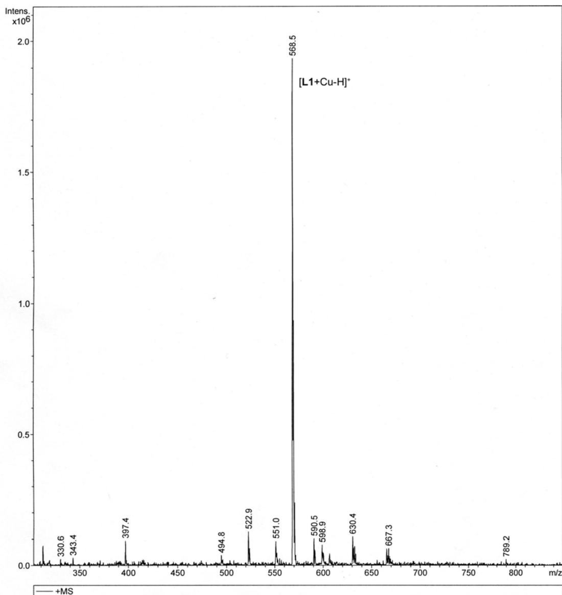
**Fig.S11** ESI mass spectrum of 20  $\mu\text{M}$  **L1** in the presence of 1.2 equiv of  $\text{Cu}^{2+}$  in water/  $\text{CH}_3\text{CN}$  (1:1 v/v) solution, indicating the formation of  $[\text{L1} + \text{Cu}^{2+} - \text{H}]^+$ .
