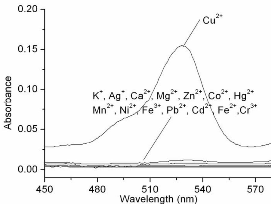
**Fig. S1** Changes in the absorption spectra of L1 (20 μM) in the presence of different metal ions (40 μM) in water/ CH<sub>3</sub>CN (1:1 v/ v).
