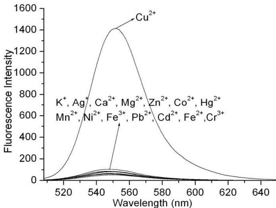
**Fig. S4** Fluorescence spectra of **L1** (20 μM) upon the addition of various metal ions (20 μM for Cu<sup>2+</sup>; 40 μM for all other cations) in water/ CH<sub>3</sub>CN (1:1 v/v) solution.
