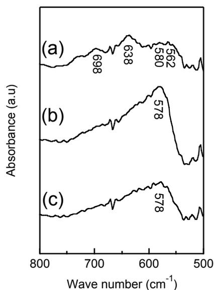
**Figure S1.** FT-IR spectrum of (a)  $\gamma$ -Fe<sub>2</sub>O<sub>3</sub>, (b) Fe<sub>3</sub>O<sub>4</sub>, and (c) synthesized Fe<sub>3</sub>O<sub>4</sub> nanoparticle cluster with a diameter of 200 nm
