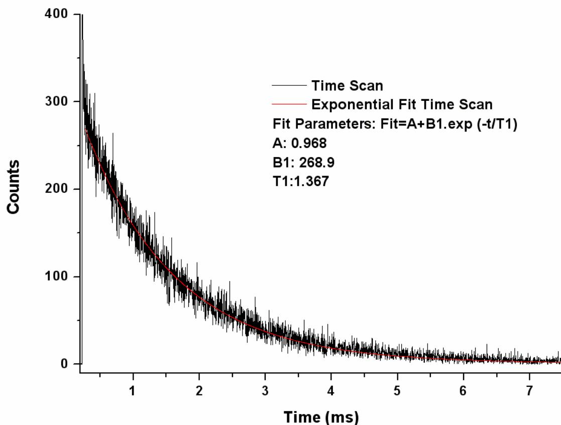
**Fig. S2** The room-temperature solid-state phosphorescence lifetime of Eu (III) complex of ligand **H<sub>3</sub>L**.
