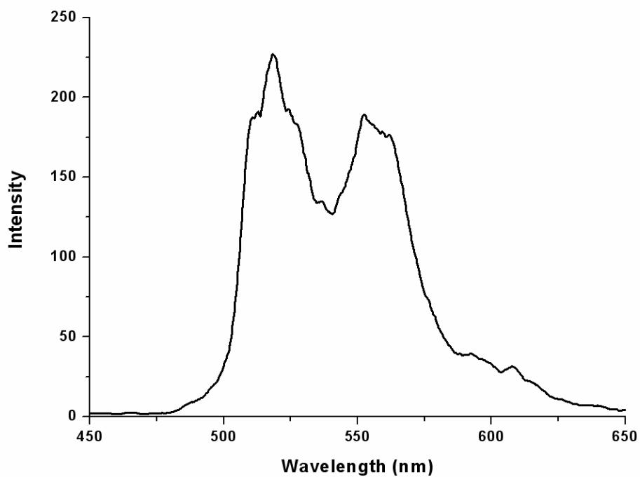
**Fig. S4** Phosphorescence spectrum of Gd(III) complex of ligand **H<sub>3</sub>L** excited at 358 nm at 77K.
