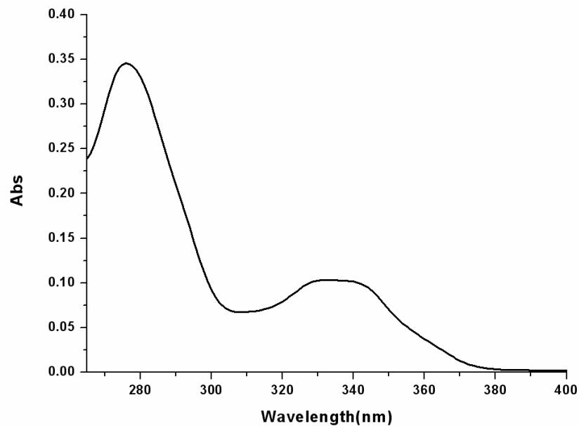
**Fig. S3** Absorption spectra of  $\mathbf{H}_3\mathbf{L}$  in DMF solution ( $2.5 \times 10^{-5}$  M).
