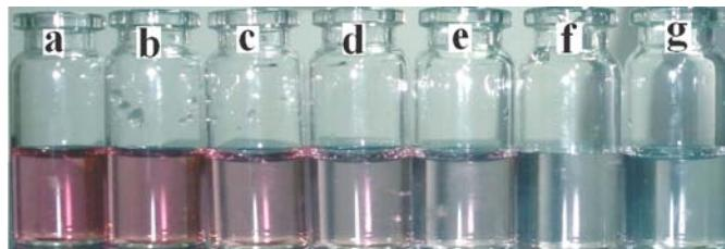
Fig. SI4 the photographs of Safranine T dyes irradiated by the mimicking sunlight in the presence of Sn-doped TiO<sub>2</sub> for different durations: (a) 0, (b) 15, (c) 30, (d) 45, (e) 60, (f) 75 and (g) 90 min.
