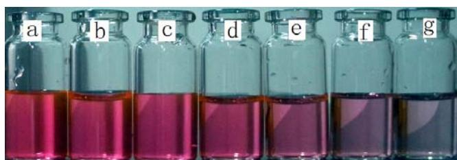
Fig. SI3 the photographs of Pyronine B dyes irradiated by the mimicking sunlight in the presence of Sn-doped TiO<sub>2</sub> for different durations: (a) 0, (b) 15, (c) 30, (d) 45, (e) 60, (f) 75 and (g) 90 min.
