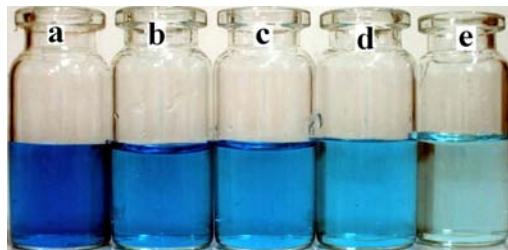
Fig. SI5 the photographs of Methylene Blue dyes irradiated by 254 UV light in the presence of Sn-doped TiO<sub>2</sub> for different durations: (a) 0, (b) 15, (c) 30, (d) 45 and (e) 60 min.
