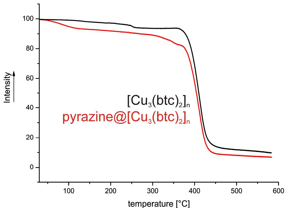
**Figure S4.** TG data of unloaded  $[Cu_3(btc)_2]_n$  material (40 deposition cycles) deposited on flexible polymer surface (black line) und of the same material after loading with pyrazine (red line).
