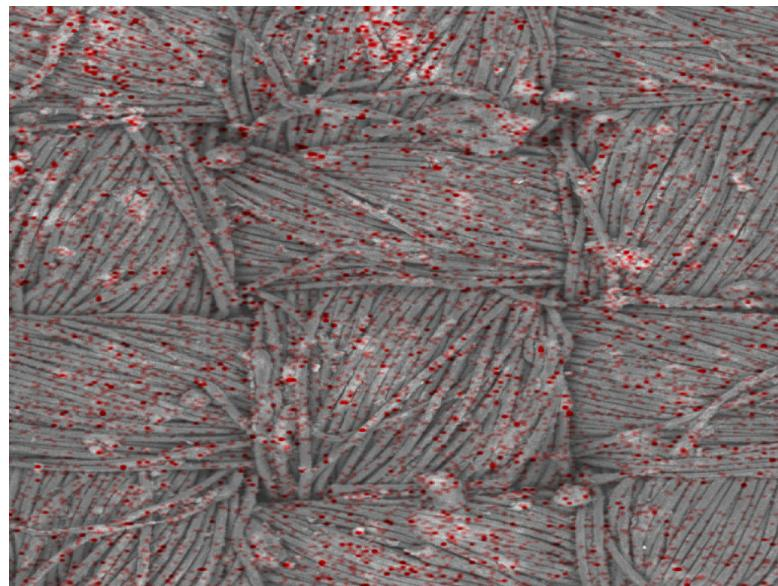
**Figure S2.** EDX Cu mapping image of a synthetic polymer substrate after applying 40 deposition cycles of  $[\text{Cu}_3(\text{btc})_3]_n$ . The areas where copper was detected are imaged in red.
