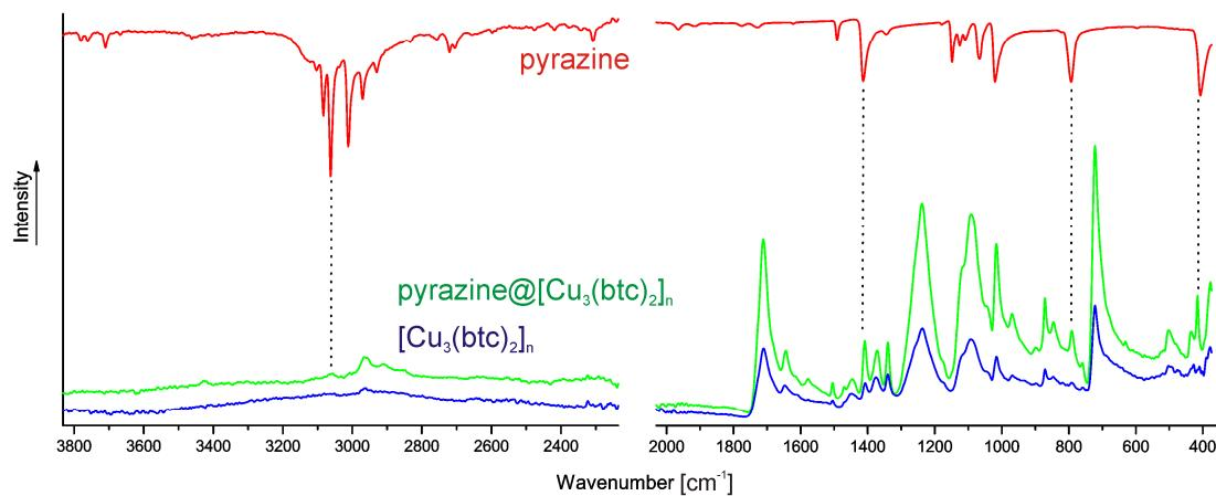
**Figure S3.** FT-IR spectra of a  $[\text{Cu}_3(\text{btc})_2]_n$  material (40 deposition cycles) deposited on flexible polymer surface before loading experiment with pyrazine (blue) and after the loaded experiment (green). The reference FT-IR spectrum of pyrazine is presented in red.
