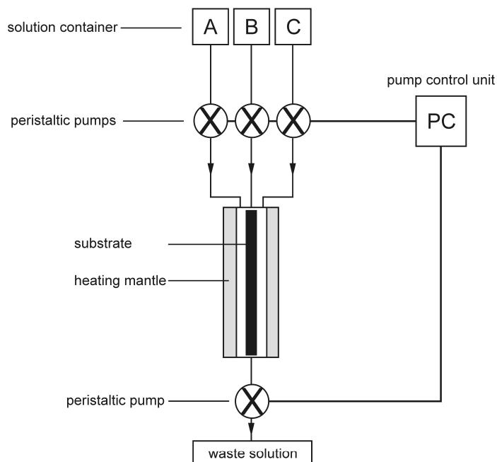
**Figure S1.** Scheme of “Step-by-step” growth apparatus.
