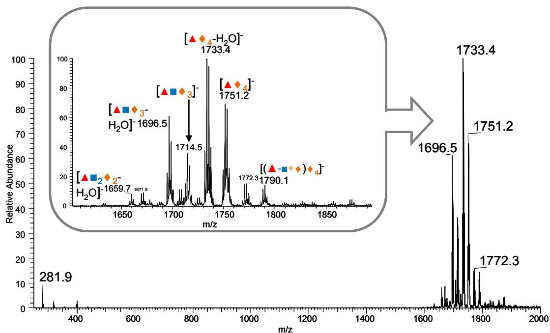
**Figure S1.** Negative ion electrospray mass spectrum for complex **1**. Insert depicts the molecular ion region and assignments.
