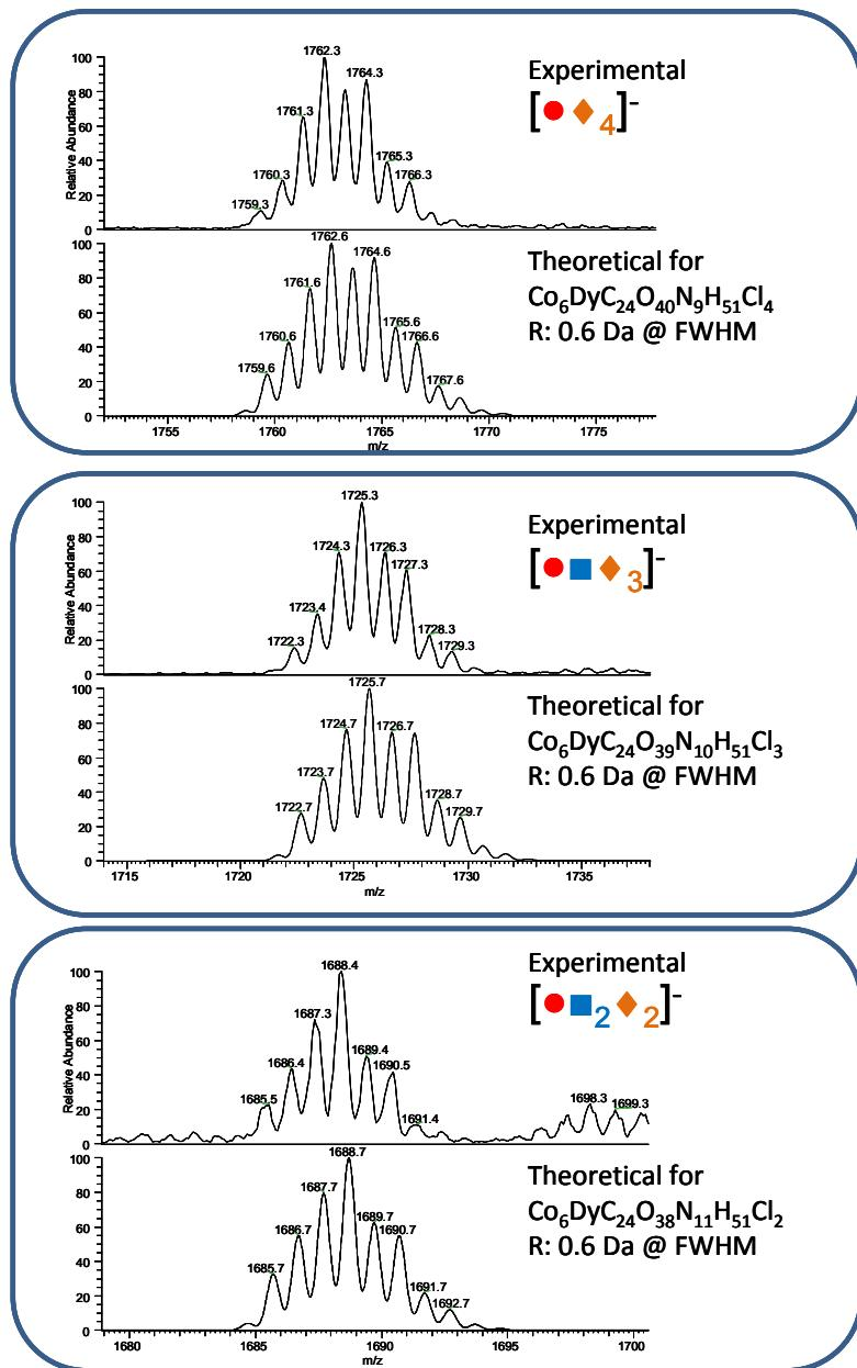
**Figure S3.** Comparison of experimental and theoretical isotopic patterns observed and determined for complex **2** under negative ion mass spectrometric conditions.
