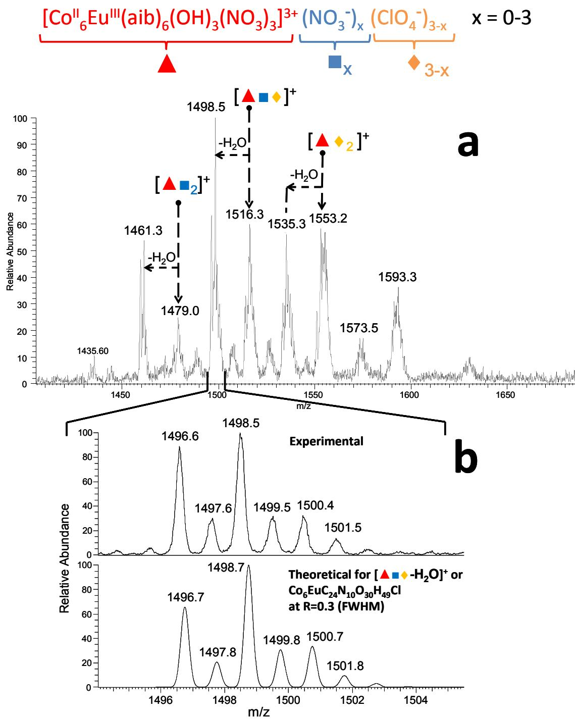
**Figure S4.** Positive ion electrospray mass spectrum for complex **1** (a). Comparison of experimental and theoretical isotopic pattern for  $[\text{Co}_6\text{Eu}_{24}\text{N}_{10}\text{O}_{30}\text{H}_{49}\text{Cl}-\text{H}_2\text{O}]^+$  (b).
