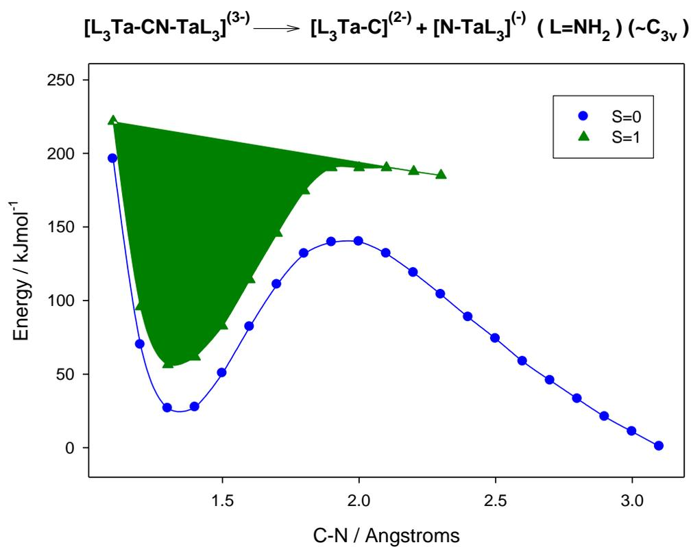
**Figure S1.** Potential energy scans for the dissociation of the dinuclear species into carbide and nitride products, in the Nb and Ta  $[L_3M-CN-ML_3]$  ( $L=[NH_2]$ ) systems.
