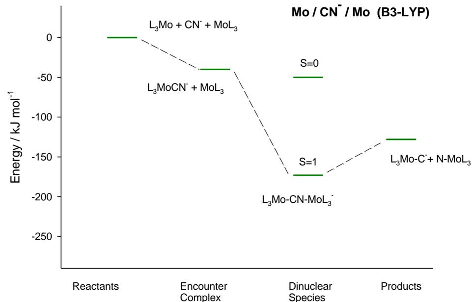
**Figure S2.** Reaction energy profiles for Mo [L<sub>3</sub>M-CN-ML<sub>3</sub>] (L=[NH<sub>2</sub>]) systems.
