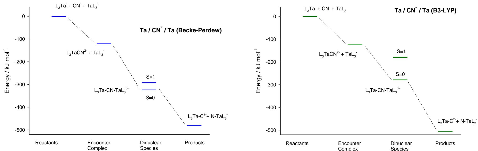
**Figure S3.** Reaction energy profiles for Ta [L<sub>3</sub>M-CN-ML<sub>3</sub>] (L=[NH<sub>2</sub>]) systems.
