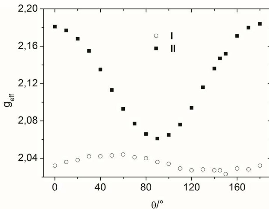
**Figure S4:** Angular dependence of  $g_{\text{eff}}$  for the two signals at W-band at 293 K (top) and 40 K (bottom). The rotation was performed around the direction perpendicular to the (11-1) face;  $\theta = 0^\circ$  corresponds to magnetic field making an angle of  $20^\circ$  with the intersection of the (011) and (11-1) faces.
