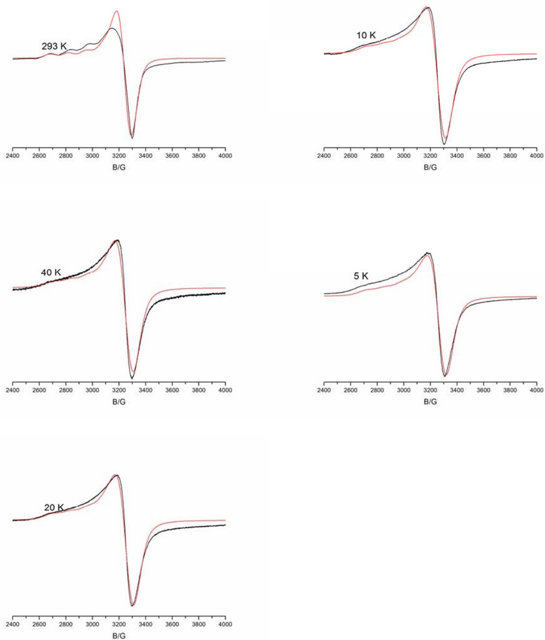
**Figure S2:** Powder X- Band EPR spectrum of  $[\text{Cu}(\text{hfac})_2(\text{N}_3\text{TEMPO})]_n$  recorded at 293, 40, 20, 10 and 5K (black lines) with the best simulation curves (red lines).
