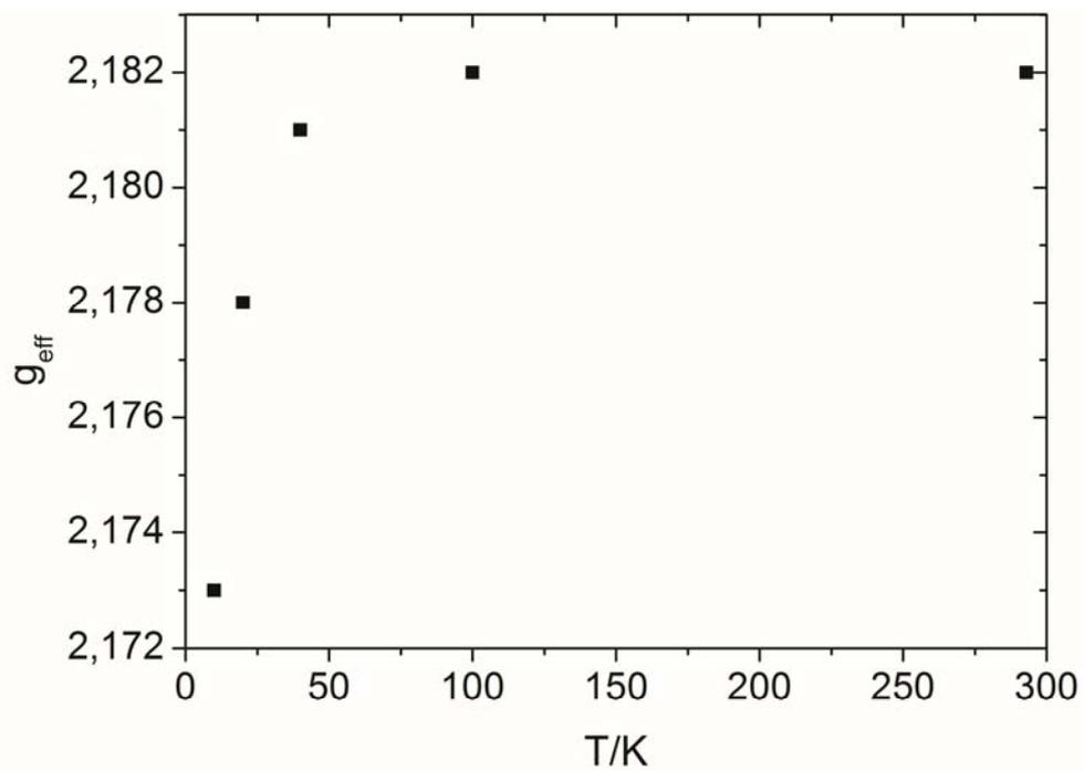
**Figure S7:** Temperature dependence of observed  $g$  values for **I** (top) and **II** (bottom) at W-band at  $\theta = 0^\circ$ .
