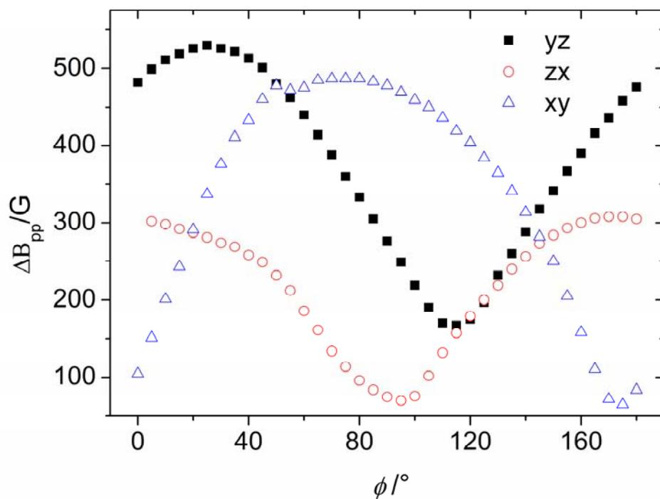
**Figure S3:** Room temperature angular dependence of the peak-to-peak linewidths for **II** at X-band in the three orthogonal laboratory axes.
