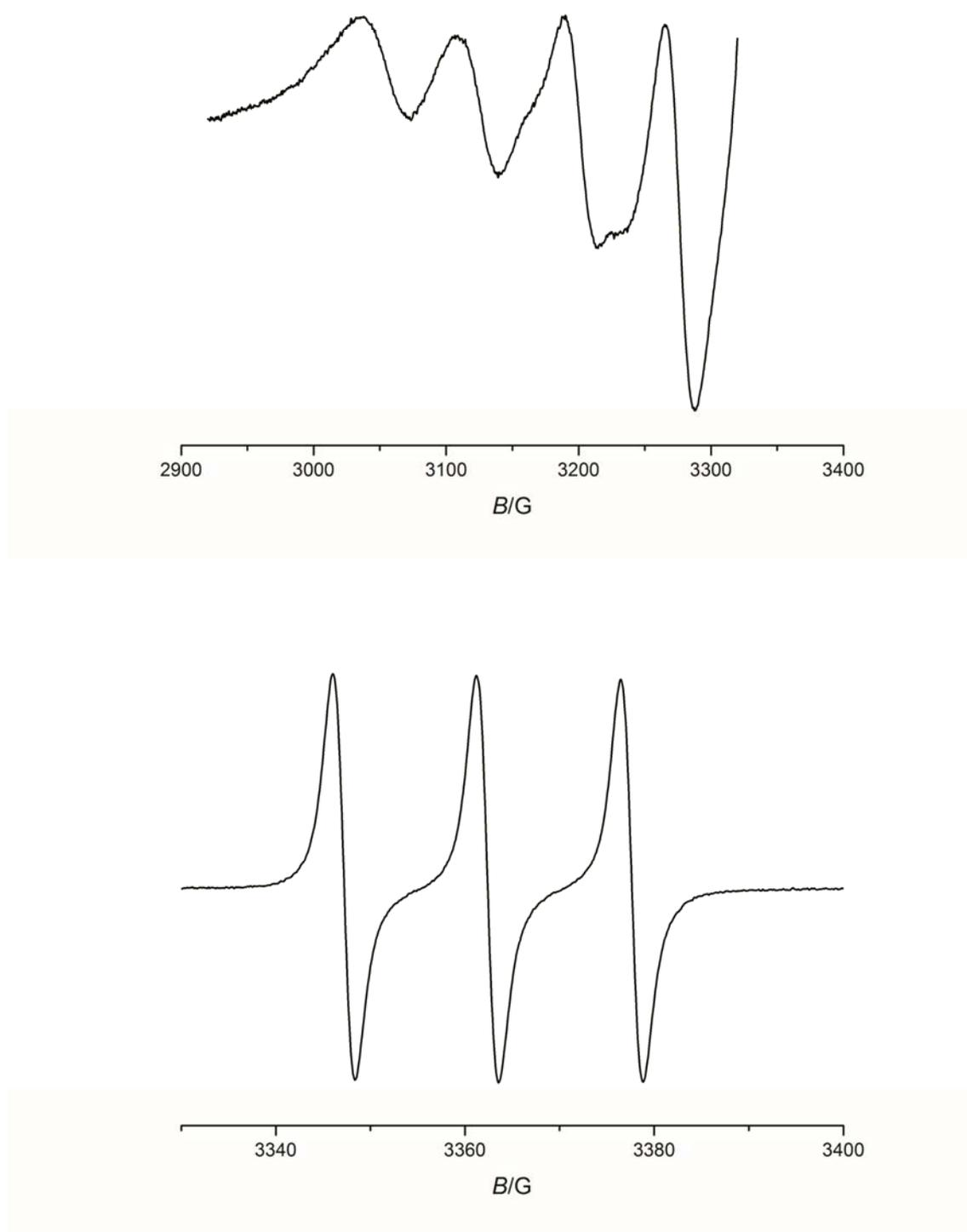
**Figure S1:** EPR spectra of  $[\text{Cu}(\text{hfac})_2(\text{N}_3\text{TEMPO})]_n$  in *n*-heptane solution. Zoom in the  $[\text{Cu}(\text{hfac})_2]$  signal (top) and the nitroxide radical signal (bottom).
