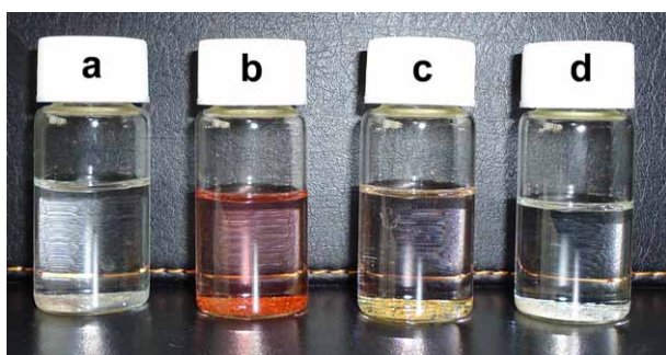
Fig. S6 Adsorption and delivery photographs bulk samples of 1 in dichloromethane solution at room temperature: (a) samples before adsorption; (b) samples immersed in the solution of I 2 for 24h; (c) samples releasing I 2 in fresh dichloromethane for 48h; (d) samples releasing I 2 in fresh dichloromethane for 72h.
