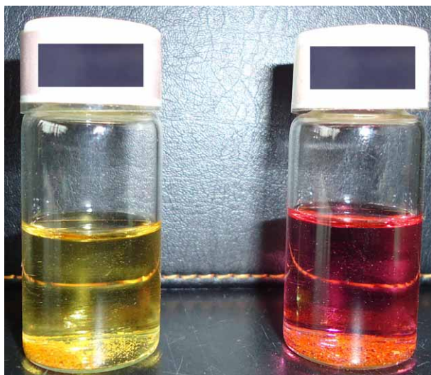
Fig. S8 the color of methanol (left) and dichloromethane (right) used for immersing 1c and the color change of moist potassium iodide-starch test paper (top).
