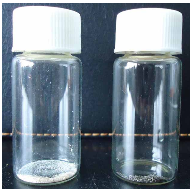
Fig. S5 Photographs showing the color change of bulk samples of 1 before and after I 2 adsorption in the air at room temperature.
