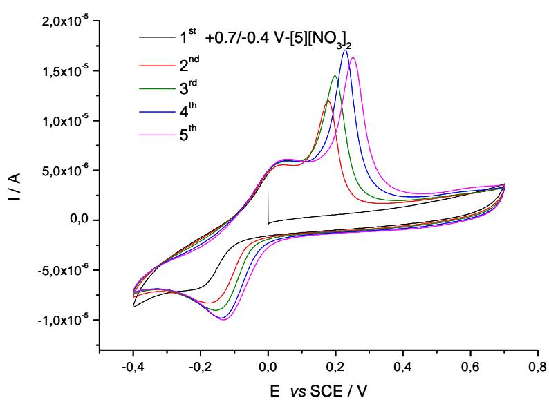
**Fig. 1S** CVs of  $[5][\text{NO}_3]_2$  in the potential range +0.7/-0.4 V showing 1 to 5 successive scans.
