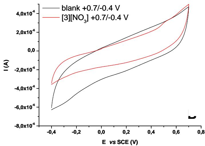
**Fig. 2S** CVs of  $[3][\text{NO}_3]$  and blank; scan rate  $100 \text{ mV s}^{-1}$ .
