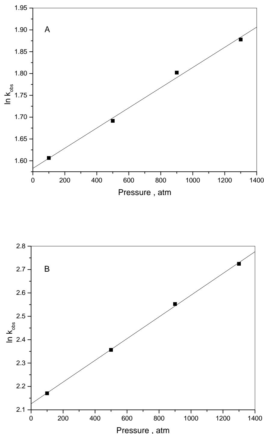
Figure S3. Plot of  $\ln(k_{\text{obs}})$  versus pressure for the second degradation step of imipramine.
