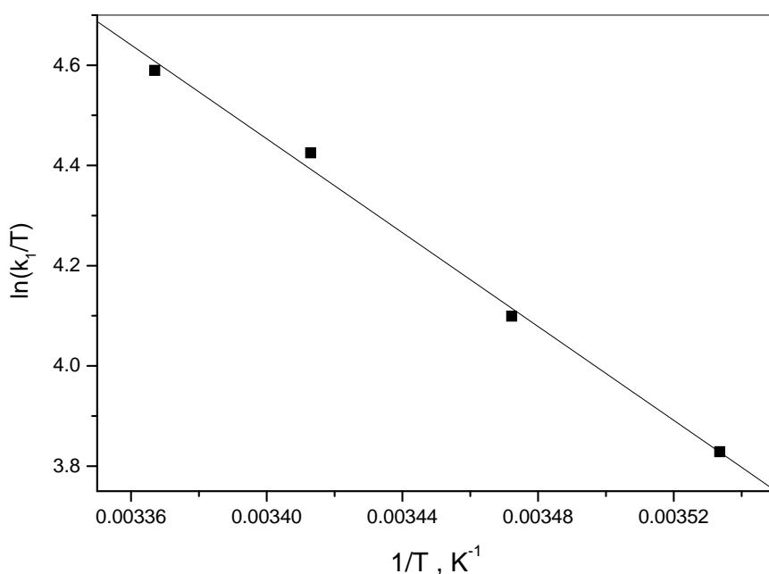
Figure S2. Eyring plot of  $\ln(k_1/T)$  versus  $1/T$  for the electron-transfer reaction between desipramine and cerium(IV). Experimental conditions:  $[Ce^{IV}] = 5 \times 10^{-5} M$ ,  $[TCA] = (0.5 - 3) \times 10^{-3} M$ ,  $[H_2SO_4] = 1.0 M$ ,  $[H^+] = 1.2 M$ ,  $I = 1.4 M$  ( $H^+$ ,  $HSO_4^-$ ,  $SO_4^{2-}$ ),  $T = 283 - 298 K$ ,  $\lambda = 630 nm$ .
