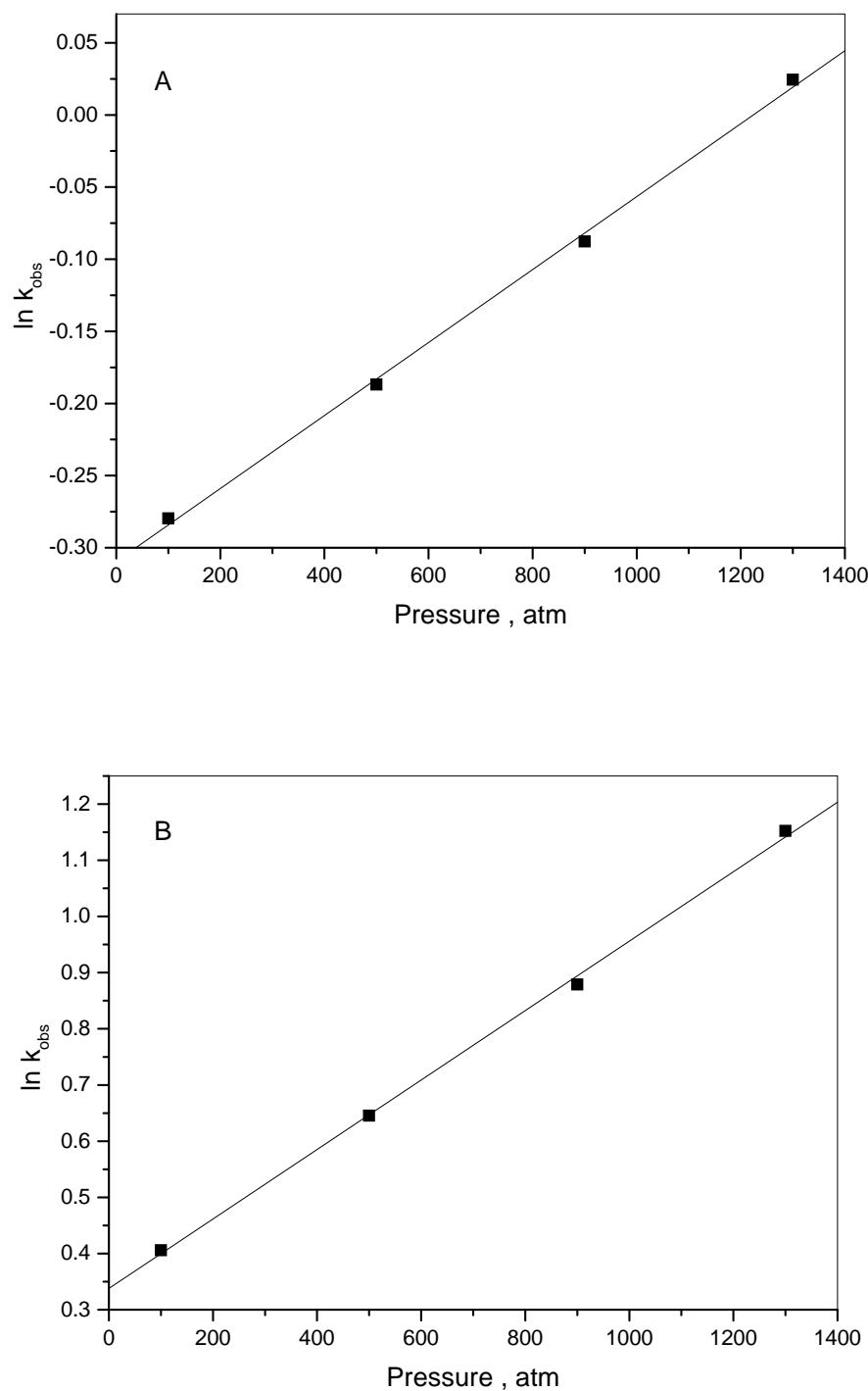
Figure S4. Plot of  $\ln(k_{\text{obs}})$  versus pressure for the third degradation step of imipramine.
