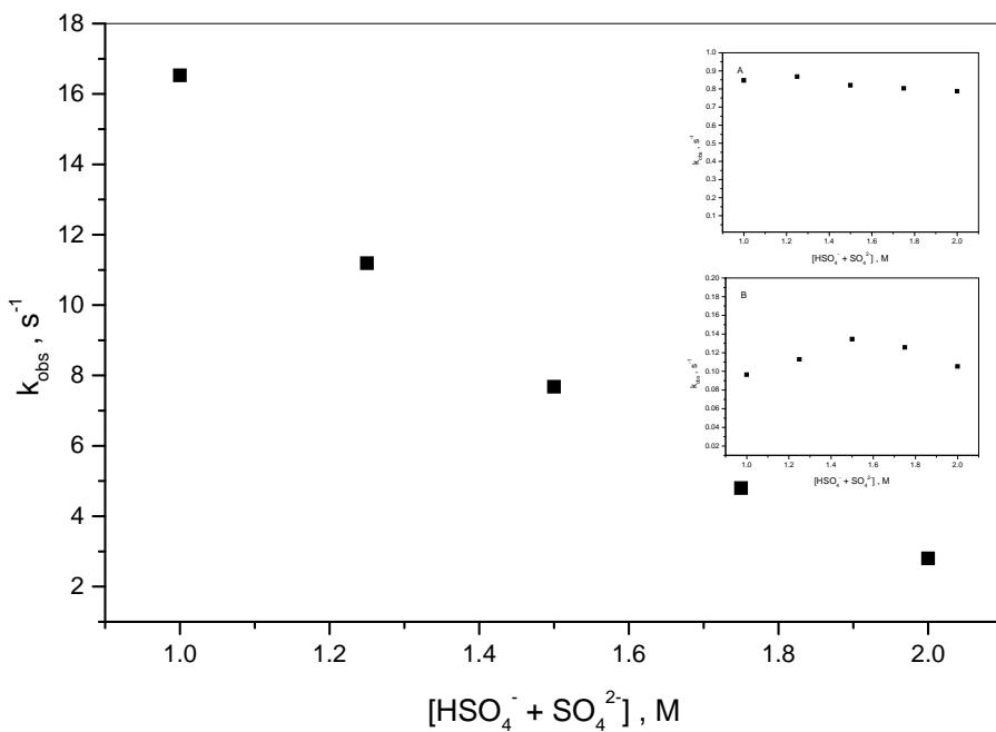
Figure S1. Plot of  $k_{\text{obs}}$  versus  $[\text{HSO}_4^- + \text{SO}_4^{2-}]$  for the electron-transfer reaction between imipramine and cerium(IV). Inset: (A): the second reaction step, (B): the third reaction step. Experimental conditions:  $[\text{Ce}^{\text{IV}}] = 5 \times 10^{-5} \text{ M}$ ,  $[\text{TCA}] = 1 \times 10^{-3} \text{ M}$ ,  $[\text{H}_2\text{SO}_4] = 1.0 \text{ M}$ ,  $[\text{Na}_2\text{SO}_4] = 0 - 1.0 \text{ M}$ ,  $I \neq \text{const}$ ,  $T = 288 \text{ K}$ .
