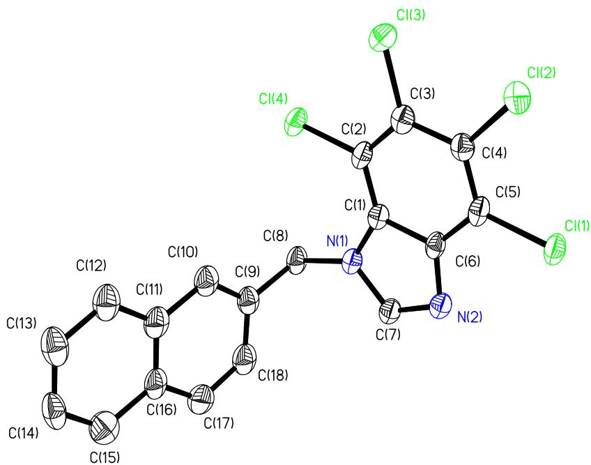
Asymmetric unit drawn with thermal ellipsoids at 50% probability.
