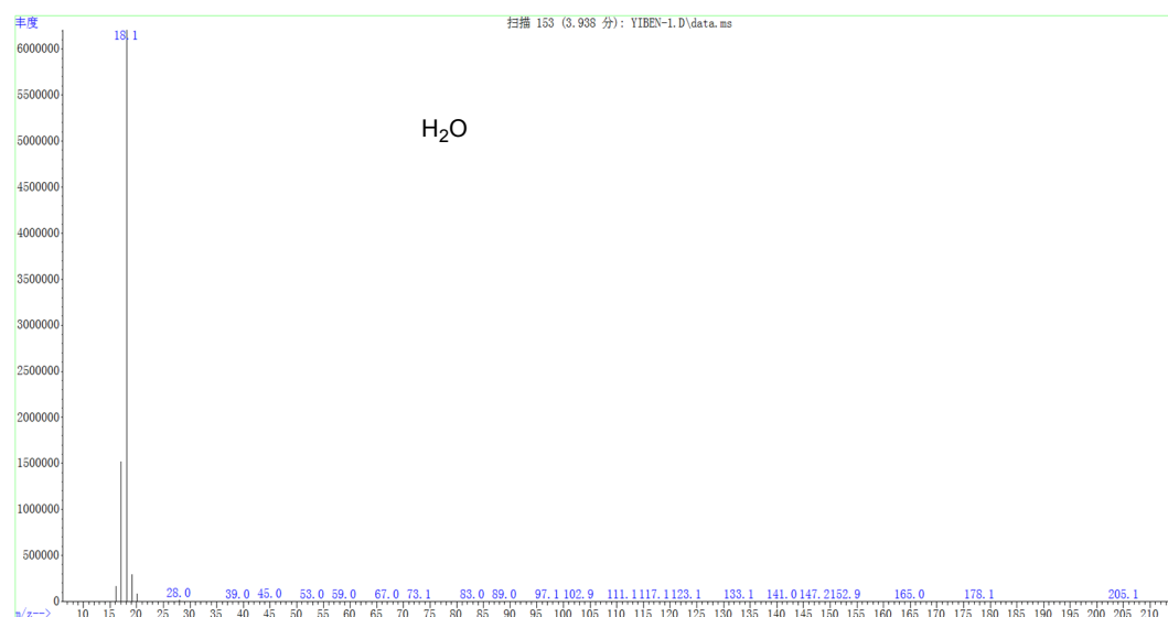
Fig. S10-1 MS graph of water in catalytic hydrogen abstraction from ethylbenzene with H 2 18 O 2 .
