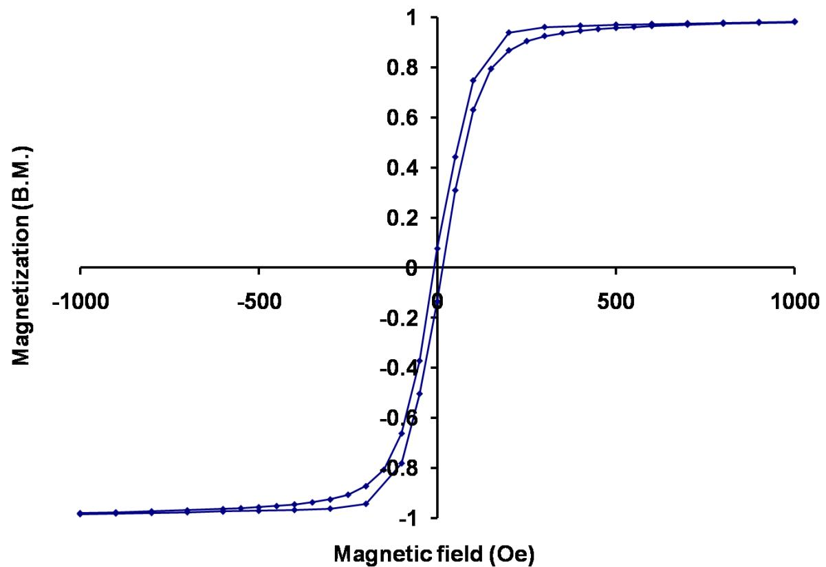
Figure S8. Hysteresis loop for 1 at 1.8 K.
