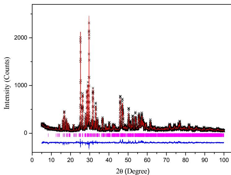
The calculated pattern (red solid line) is compared with observed data ( $\times$ ). The locations of reflections are indicated by the magenta vertical bars. The difference between the observed and calculated profiles is shown at the bottom (blue solid line).
