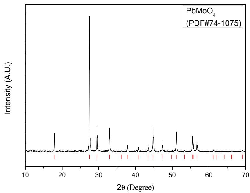
S5. Thermogravimetric analysis diagram for  $\text{PbWSeO}_6$  and XRD pattern for calcined product
