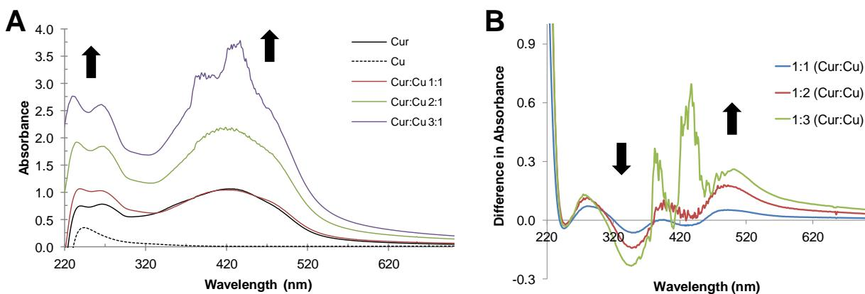
**Fig. S26** UV-vis spectra for A) curcumin in the presence of varying Cu<sup>+</sup> ratios in MOPS buffer (10 mM, pH 7.0) and B) difference spectra of A, subtracting out contributions from curcumin and Cu<sup>+</sup> only. A 1:1 ratio represents 29  $\mu\text{M}$  Cu<sup>+</sup> and curcumin, and higher ratios are obtained by increasing concentrations of curcumin with a fixed Cu<sup>+</sup> concentration (29  $\mu\text{M}$ ). Reaction times were 10 min in MOPS buffer (pH 7.0, 10 mM).
