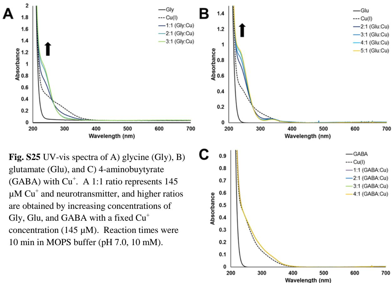
**Fig. S25** UV-vis spectra of A) glycine (Gly), B) glutamate (Glu), and C) 4-aminobutyrate (GABA) with Cu<sup>+</sup>. A 1:1 ratio represents 145  $\mu\text{M}$  Cu<sup>+</sup> and neurotransmitter, and higher ratios are obtained by increasing concentrations of Gly, Glu, and GABA with a fixed Cu<sup>+</sup> concentration (145  $\mu\text{M}$ ). Reaction times were 10 min in MOPS buffer (pH 7.0, 10 mM).
