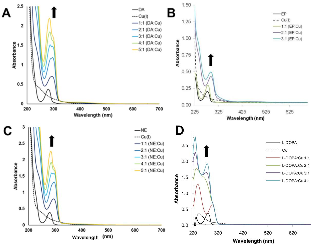
**Fig. S24** UV-vis spectra of A) dopamine (DA), B) epinephrine (EP), C) norepinephrine (NE), and L-DOPA with Cu<sup>+</sup>. A 1:1 ratio represents 145 μM Cu<sup>+</sup> and neurotransmitter, and higher ratios are obtained by increasing concentrations of DA, EP, NE, and L-DOPA with a fixed Cu<sup>+</sup> concentration (145 μM). Reaction times were 10 min in MOPS buffer (pH 7.0, 10 mM).
