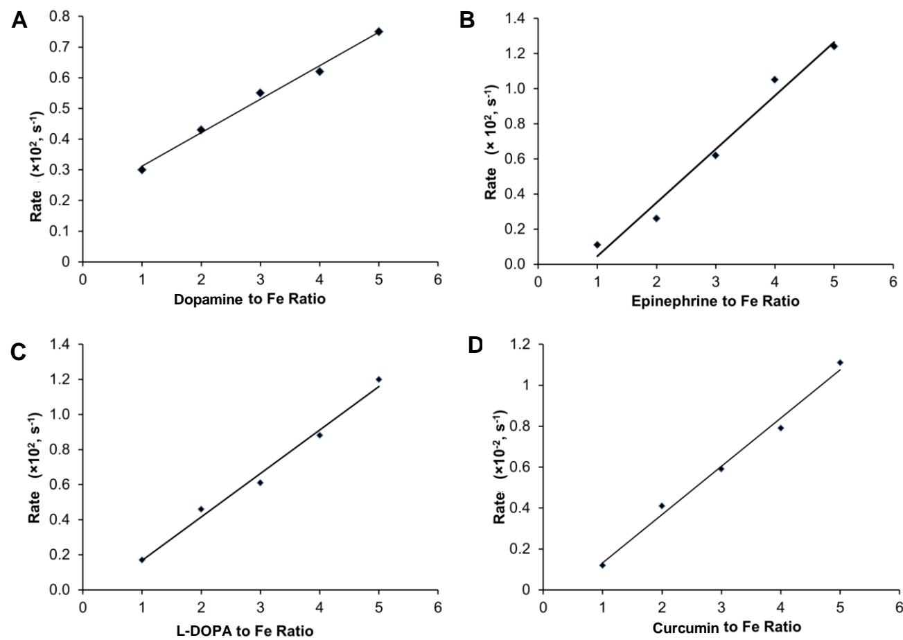
**Fig. S21** Graphs of  $\text{Fe}^{2+}$  oxidation rate vs. molar ratio of A) dopamine (DA), B) norepinephrine (NE), C) *l*-dihydroxyphenylalanine (L-DOPA), and D) curcumin with  $\text{Fe}^{2+}$ . Error bars are within marker size.
