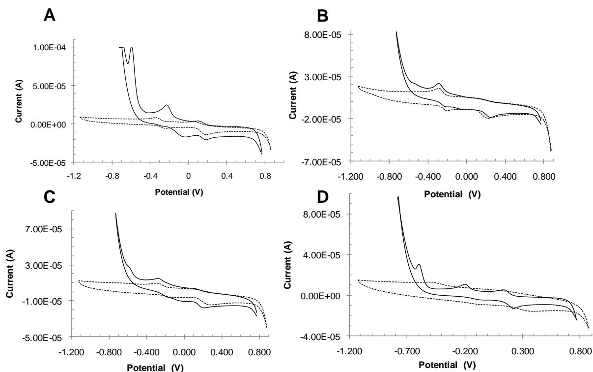
**Fig. S15** Cyclic voltammograms vs. NHE for A) dopamine, B) epinephrine, C) norepinephrine, and D) *l*-dihydroxyphenylalanine (L-DOPA; 380  $\mu\text{M}$ , dotted line) and 10 min after addition of  $\text{CuSO}_4$  (380  $\mu\text{M}$ ; solid line) in MOPS buffer (64 mM, pH 7.0) with  $\text{KNO}_3$  (64 mM) as a supporting electrolyte.
