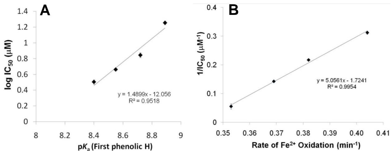
**Fig. S11** A) Graph of  $\log \text{IC}_{50}$  for catecholamine (DA, EP, NE, and L-DOPA) prevention of iron-mediated DNA damage vs.  $\text{p}K_a$  of the first phenolic H atom with the linear fit shown. B) Graph of  $1/\text{IC}_{50}$  vs. initial rate of  $\text{Fe}^{2+}$  oxidation in the presence of the four catecholamines with the linear fit shown.
