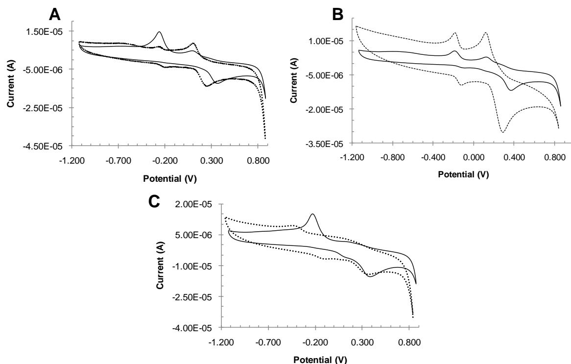
**Fig. S12** Cyclic voltammograms vs. NHE for A) dopamine, B) norepinephrine, and C) *l*-dihydroxyphenylalanine (L-DOPA; 380  $\mu$ M, dotted line) and 10 min after addition of FeSO<sub>4</sub> (380  $\mu$ M; solid line) in MES buffer (64 mM, pH 6.0) with KNO<sub>3</sub> (64 mM) as a supporting electrolyte.
