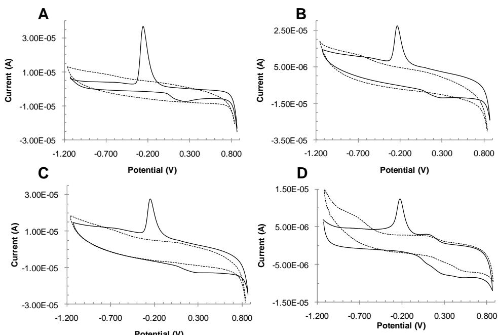
**Fig. S13** Cyclic voltammograms vs. NHE for A) glycine, B) glutamate, C) 4-aminobutyrate, and D) curcumin (380  $\mu$ M, dotted line) and 10 min after addition of FeSO<sub>4</sub> (380  $\mu$ M; solid line) in MES buffer (64 mM, pH 6.0) with KNO<sub>3</sub> (64 mM) as a supporting electrolyte.
