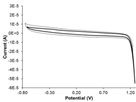
**Fig. S17** Cyclic voltammograms vs. NHE for tartrate (145  $\mu$ M) in MES buffer (64 mM, pH 6.0; dotted line) or MOPS buffer (64 mM, pH 7.2; solid line) with KNO<sub>3</sub> (64 mM) as a supporting electrolyte.
