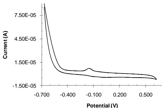
**Fig. S14** Cyclic voltammogram vs. NHE of  $\text{CuSO}_4$  (380  $\mu\text{M}$ ) in MOPS buffer (64 mM, pH 7.0) with  $\text{KNO}_3$  (64 mM) as a supporting electrolyte.
