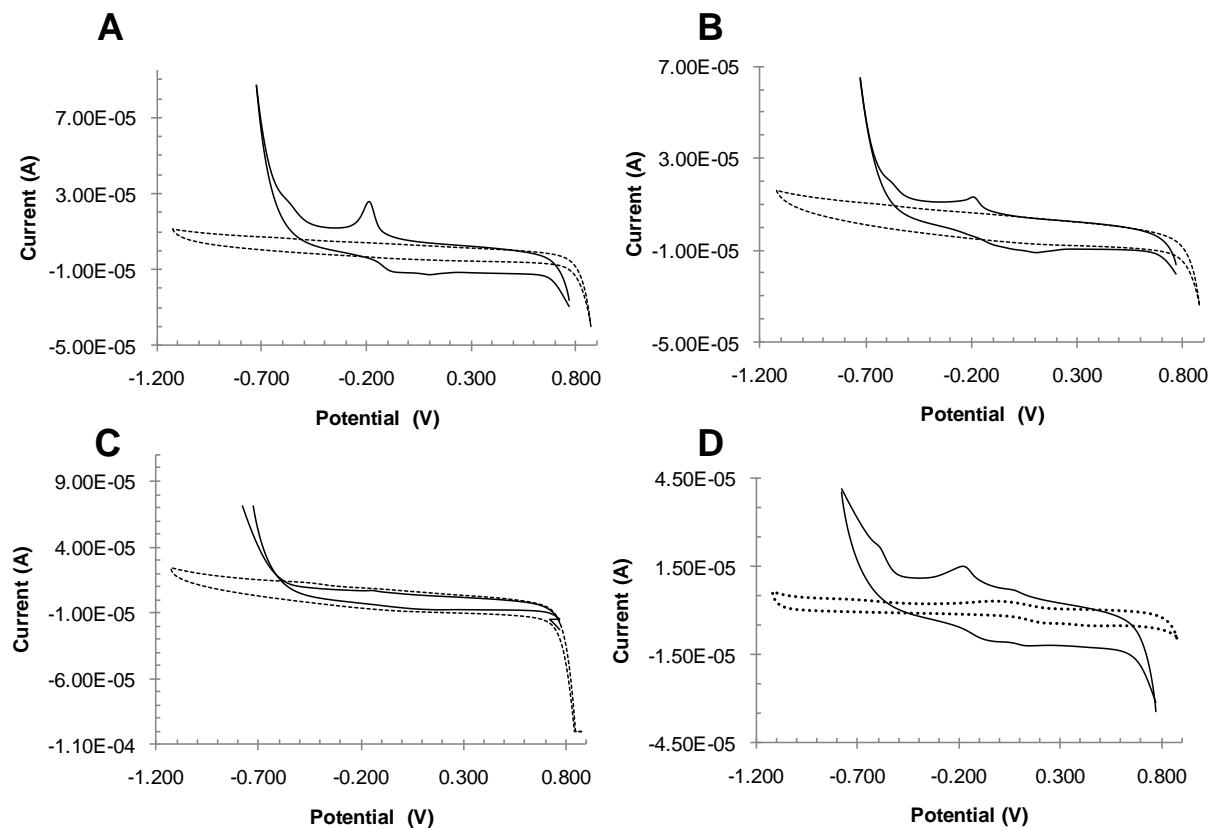
**Fig. S16** Cyclic voltammograms vs. NHE for A) glycine, B) glutamate, C) 4-aminobutyrate, and D) curcumin (380  $\mu$ M, dotted line) and 10 min after addition of CuSO<sub>4</sub> (380  $\mu$ M; solid line) in MOPS buffer (64 mM, pH 7.0) with KNO<sub>3</sub> (64 mM) as a supporting electrolyte.
