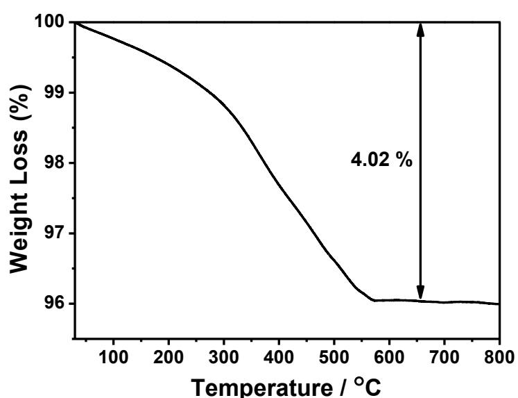
**Fig. S2.** TGA curves of the as-prepared yttrium tungstate precursor.
