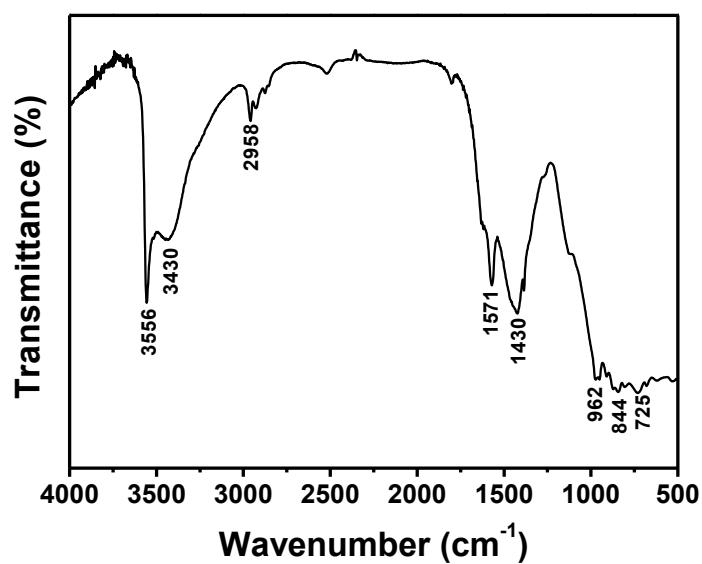
**Fig. S1.** FT-IR spectrum of the as-prepared yttrium tungstate precursor.
