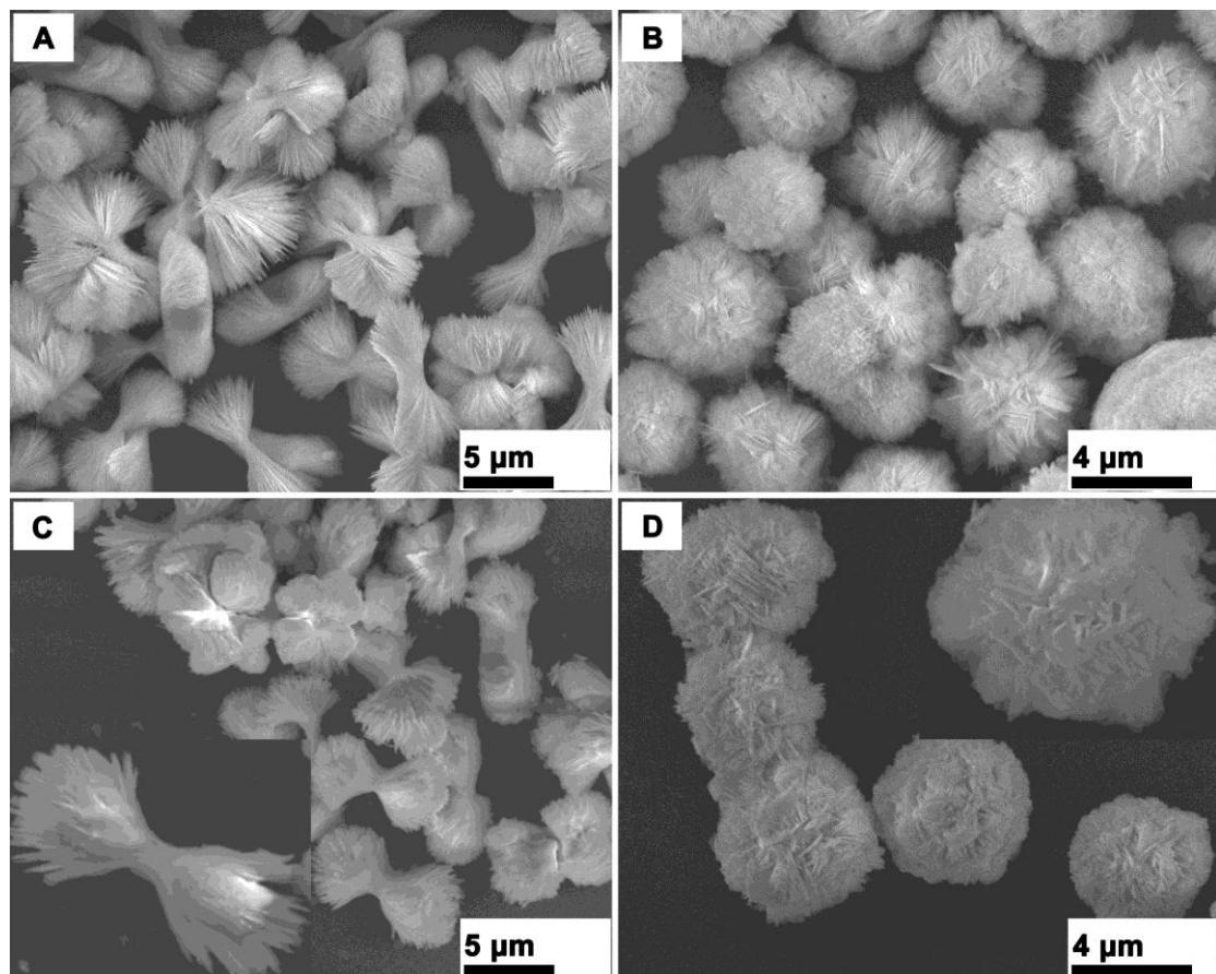
**Fig. S3.** SEM images of the as-prepared yttrium tungstate precursors prepared with (A) 0.5 mmol, (B) 0.75 mmol SDBS, and SEM images of  $\text{Y}_2(\text{WO}_4)_3$  prepared with (C) 0.5 mmol, (D) 0.75 mmol samples after annealed at 800 °C for 2 h.
