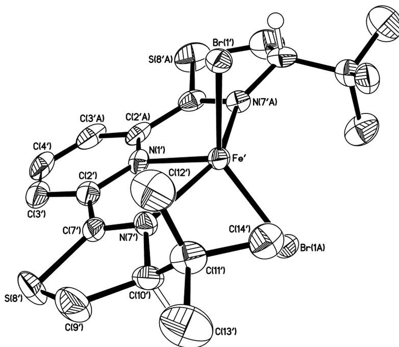
**Fig. S7** The molecular structure of the  $C_2$ -symmetric complex  $[\text{Fe}(\text{L}2)\text{Br}_2]\text{-II}$ , one of the two crystallographically independent complexes present in the crystals of  $[\text{Fe}(\text{L}2)\text{Br}_2]$  (50% probability ellipsoids).
