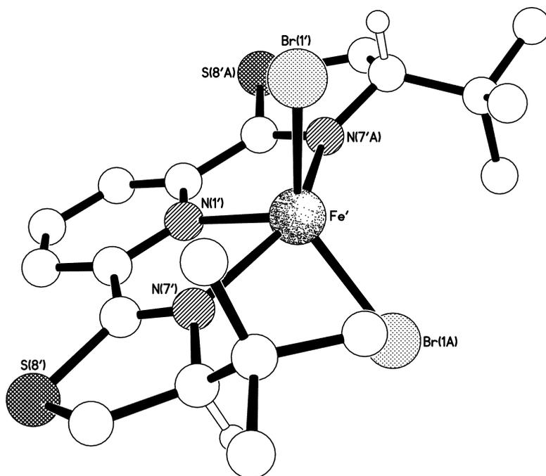
**Fig. S6** The molecular structure of the C<sub>2</sub>-symmetric complex [Fe(L2)Br<sub>2</sub>]-II, one of the two crystallographically independent complexes present in the crystals of [Fe(L2)Br<sub>2</sub>].
