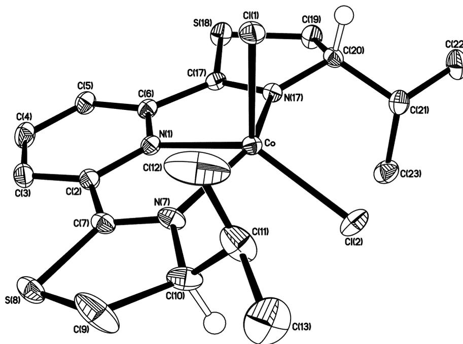
**Fig. S13** The molecular structure of [Co(L3)Cl<sub>2</sub>]-I, one of the two crystallographically independent complexes present in the crystals of [Co(L3)Cl<sub>2</sub>] (30% probability ellipsoids).
