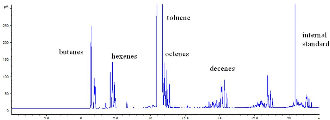
Figure S18. A GC trace of the liquid fraction obtained from the oligomerisation of ethylene by  $[\text{Co}(\text{L}2)\text{Cl}_2]$  with 500 eq. MAO. Internal standard: 2,2,4,4,6,8,8–heptamethylnonane.
