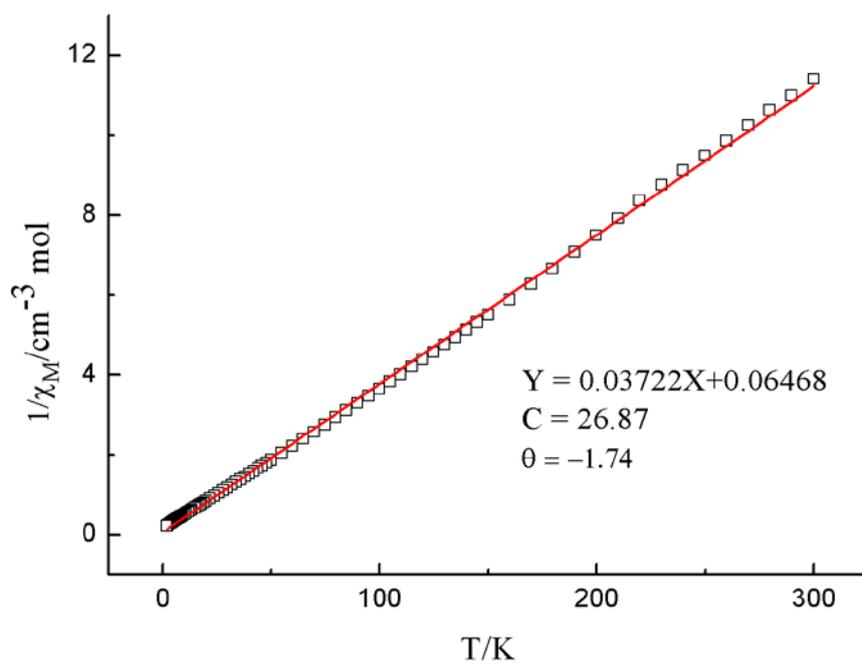
Figure S6. The plots of  $1/\chi_M$  versus  $T$  for compound **6** (Tm) and the linear fit of Curie-Weiss law at 1000 Oe field.
