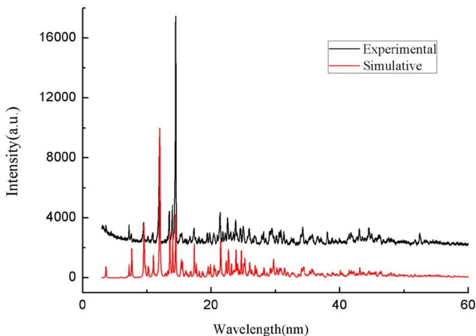
**Figure S13.** The simulative and experiment PXRD spectra of compound **4**.
