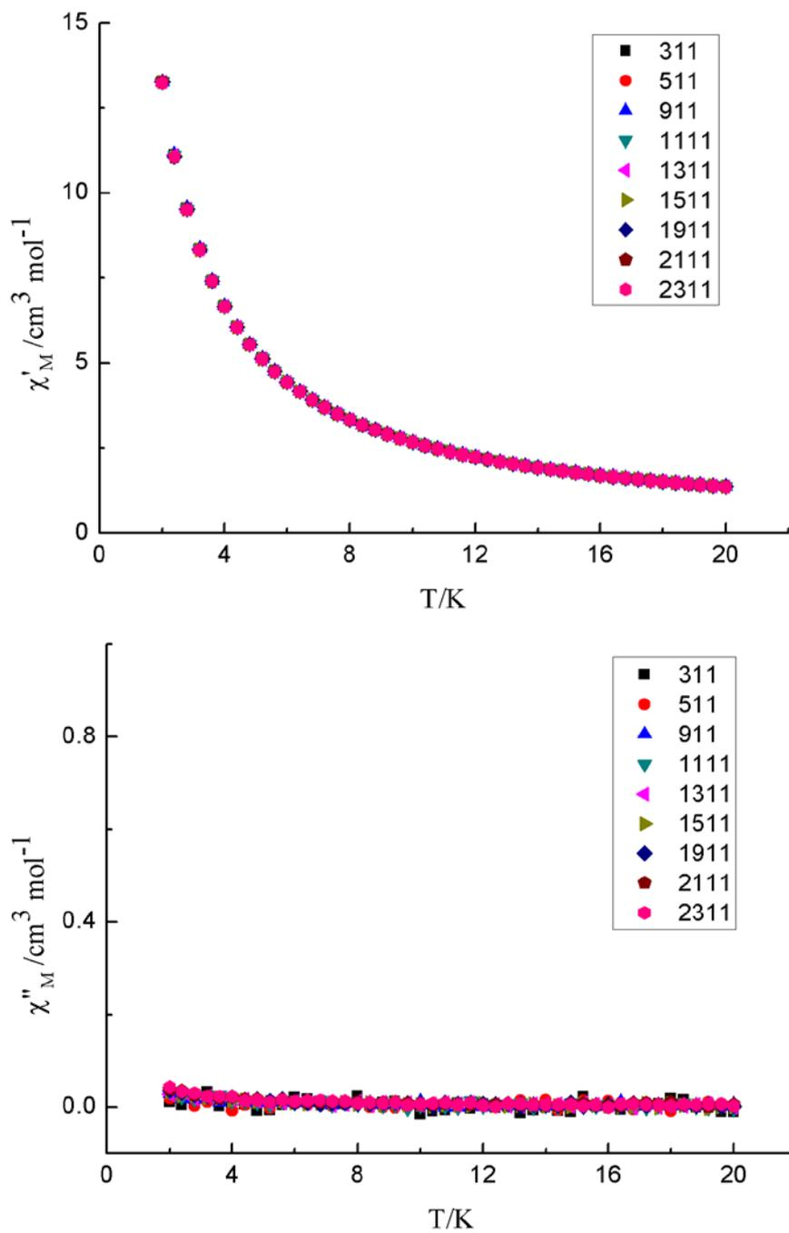
**Figure S8.** Temperature dependence of the in-phase ( $\chi'$ ) and out-of-phase ( $\chi''$ ) AC susceptibilities for **3** (Tb) at the indicated frequencies.
