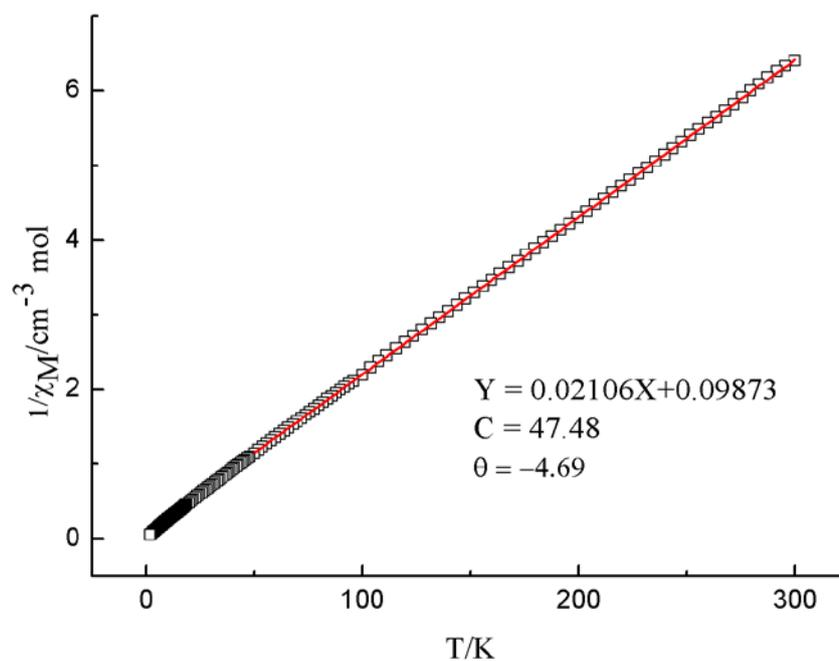
Figure S4. The plots of  $1/\chi_M$  versus  $T$  for compound **4** (Dy) and the linear fit of Curie-Weiss law at 1000 Oe field.
