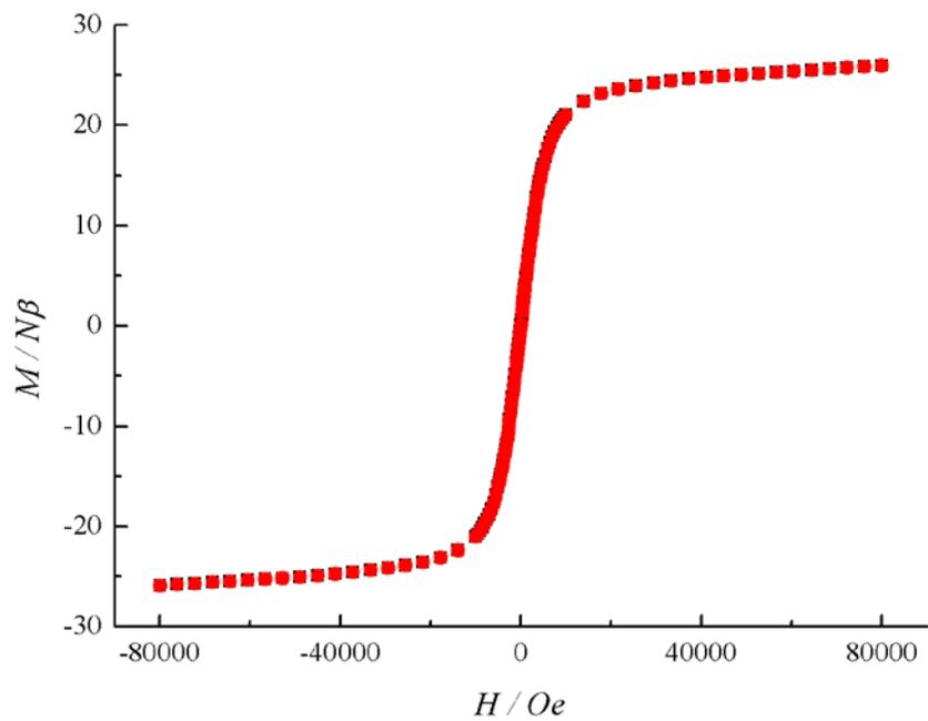
**Figure S12.** The M-H plot of in compound **4**, displaying no magnetic hysteresis loops.
