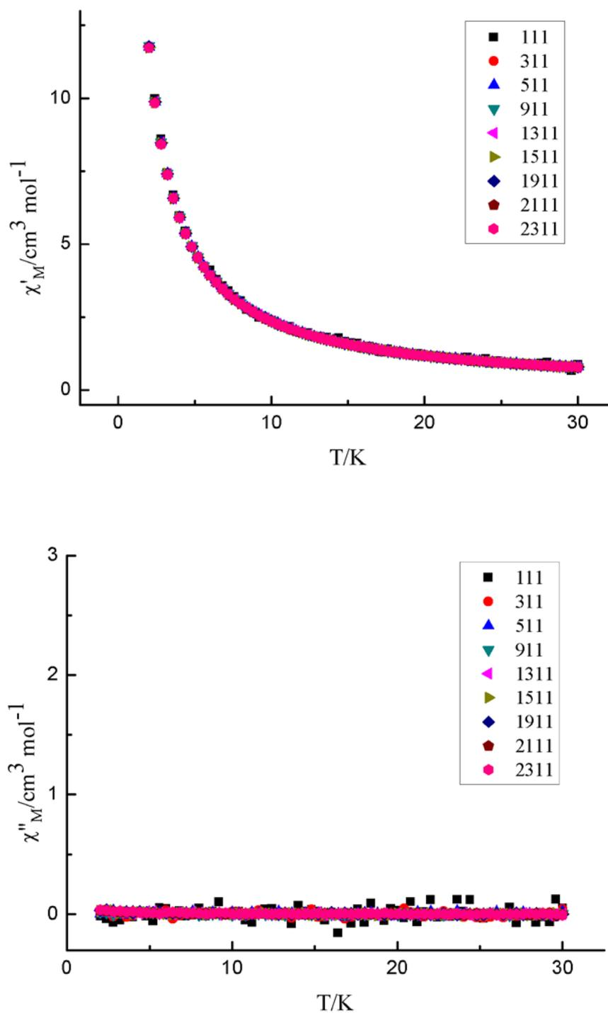
**Figure S7.** Temperature dependence of the in-phase ( $\chi'$ ) and out-of-phase ( $\chi''$ ) AC susceptibilities for **2(Gd)** at the indicated frequencies.
