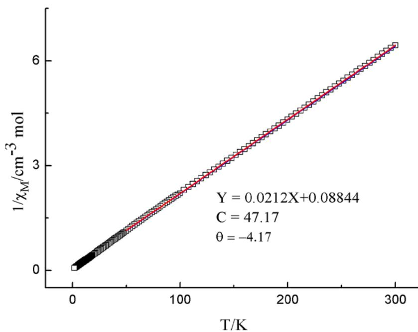
Figure S5. The plots of  $1/\chi_M$  versus  $T$  for compound **5** (Ho) and the linear fit of Curie-Weiss law at 1000 Oe field.
