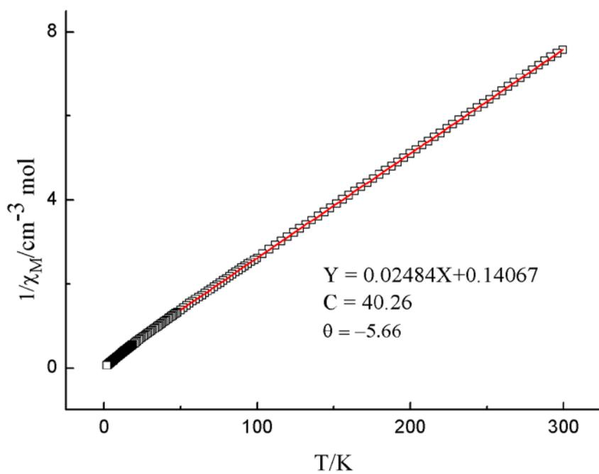
Figure S3. The plots of  $1/\chi_M$  versus  $T$  for compound **3** (Tb) and the linear fit of Curie-Weiss law at 1000 Oe field.
