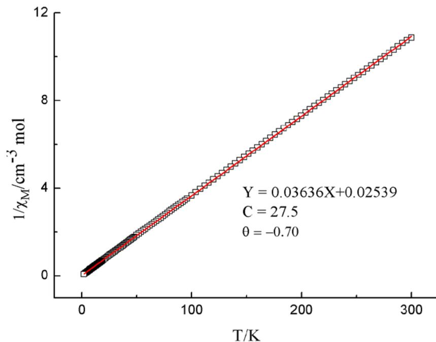
Figure S2. The plots of  $1/\chi_M$  versus  $T$  for compound **2** (Gd) and the linear fit of Curie-Weiss law at 1000 Oe field.
