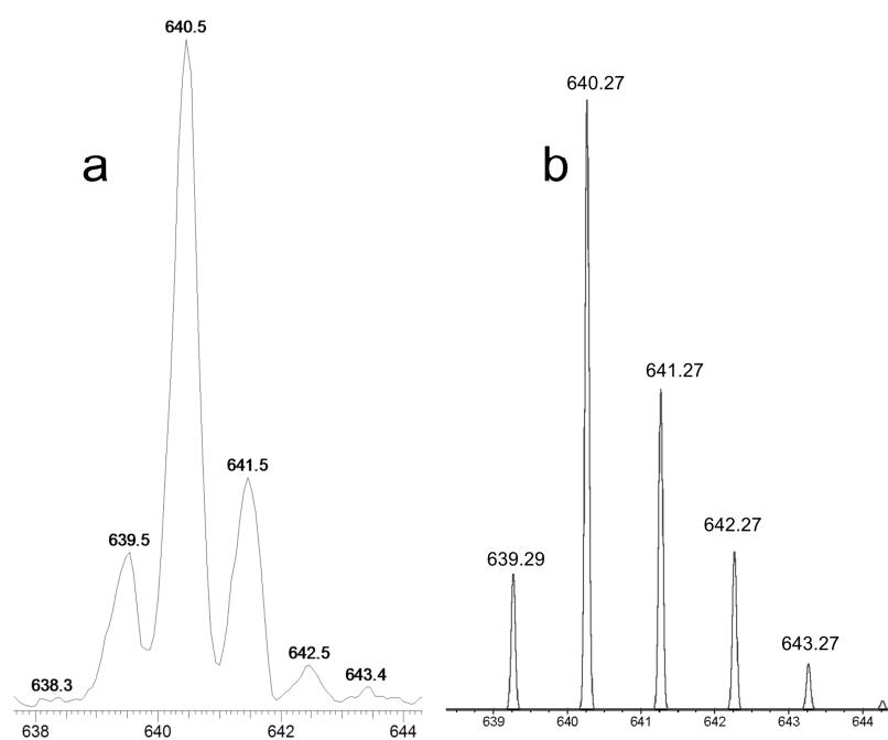
**Figure S2.** (a) Expanded ion cluster at  $m/z$  640.5 from the positive ESI-mass spectrum of an acetonitrile solution of **1** and  $\text{Mg}(\text{ClO}_4)_2$ ; (b) simulated isotopic pattern of  $[\mathbf{1} \cdot \text{Mg}-\text{H}]^+$ .
