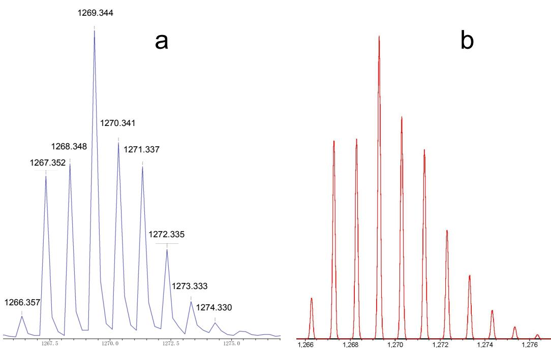
**Figure S4.** (a) Expanded ion cluster at  $m/z$  1269 from the positive MALDI-TOF mass spectrum of an acetonitrile solution of **2** and  $\text{Mg}(\text{ClO}_4)_2$ ; (b) simulated isotopic pattern of  $[2 \cdot 2\text{Mg} \cdot 3\text{ClO}_4]^+$ .
