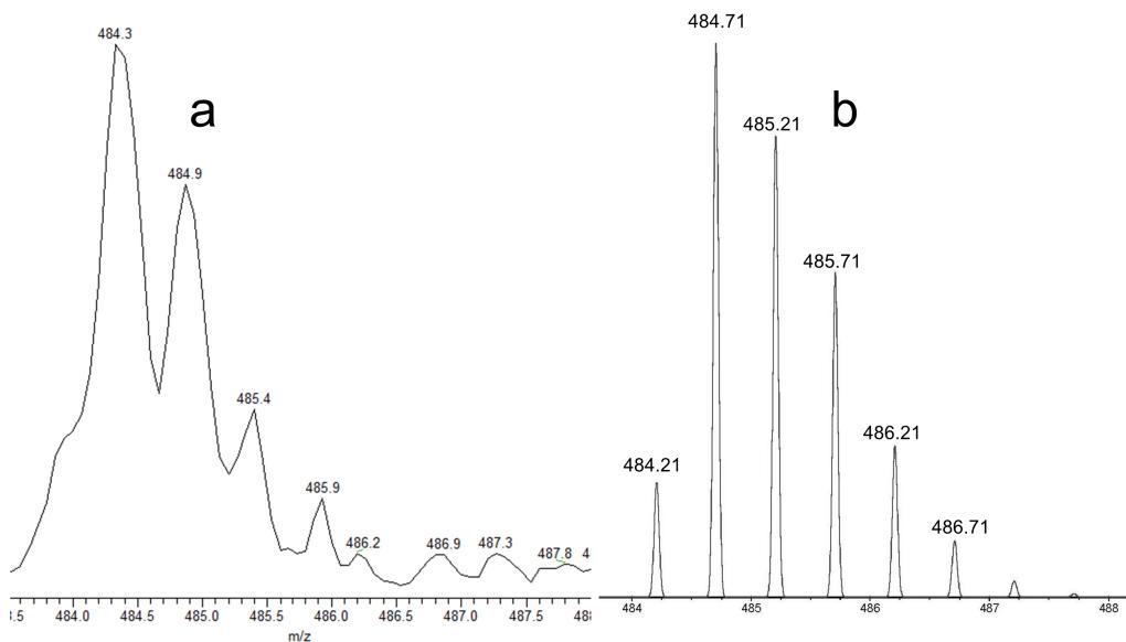
**Figure S3.** (a) Expanded ion cluster at  $m/z$  484 from the positive ESI-mass spectrum of an acetonitrile solution of **2** and  $\text{Mg}(\text{ClO}_4)_2$ ; (b) simulated isotopic pattern of  $[\mathbf{2} \cdot 2\text{Mg}-2\text{H}]^{2+}$ .
