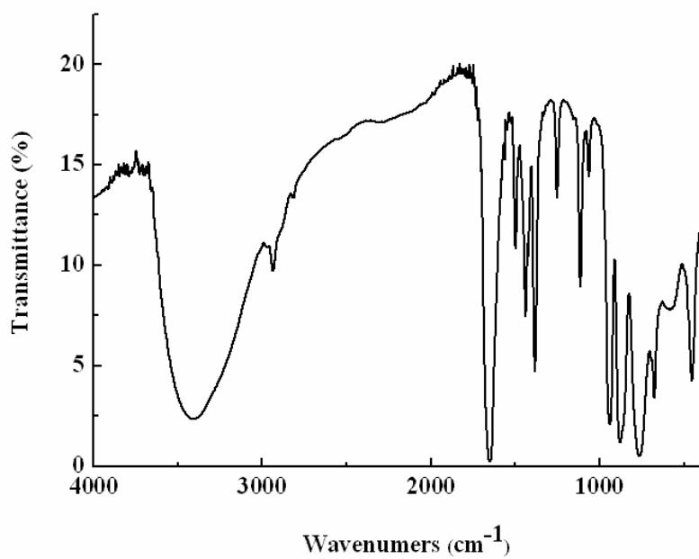
**Fig. S10.** IR spectrum of **La-POM**.
