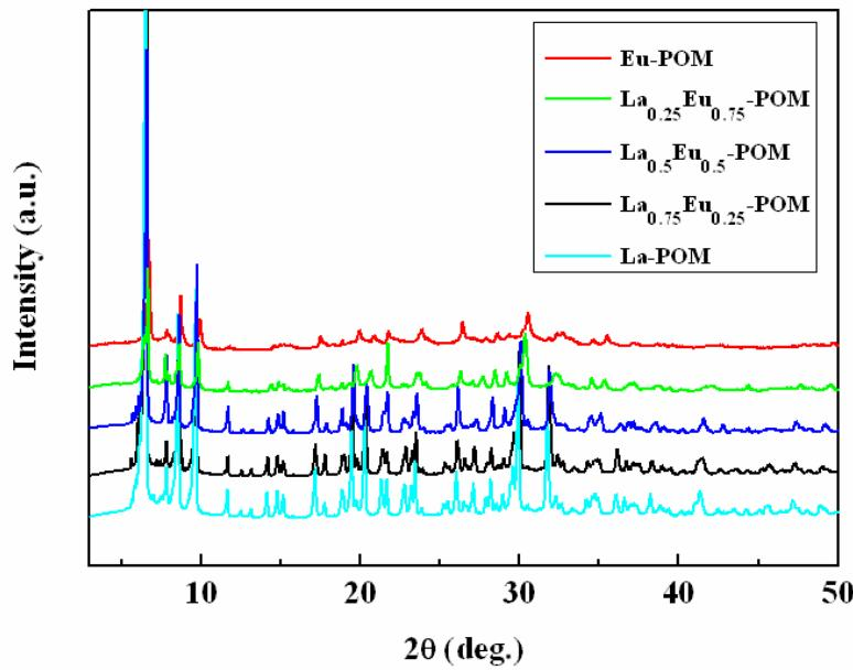
**Fig. S4.** PXRD for  $\text{La}_{1-x}\text{Eu}_x\text{-POM}$ .
