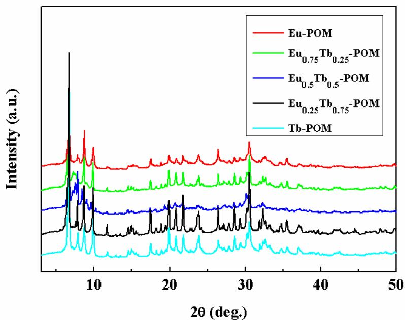
Fig. S6. PXRD for  $\text{Eu}_x\text{Tb}_{1-x}\text{-POM}$ .
