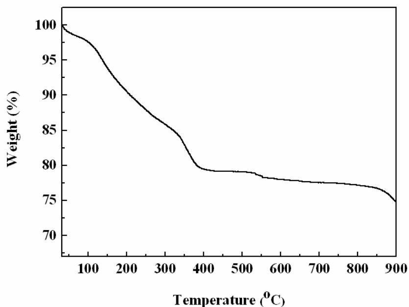
**Fig. S9.** TGA curve for **Tb-POM**.
