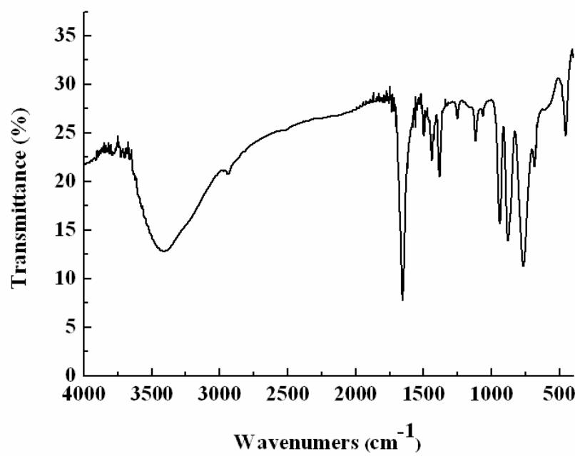
**Fig. S12.** IR spectrum of **Tb-POM**.
