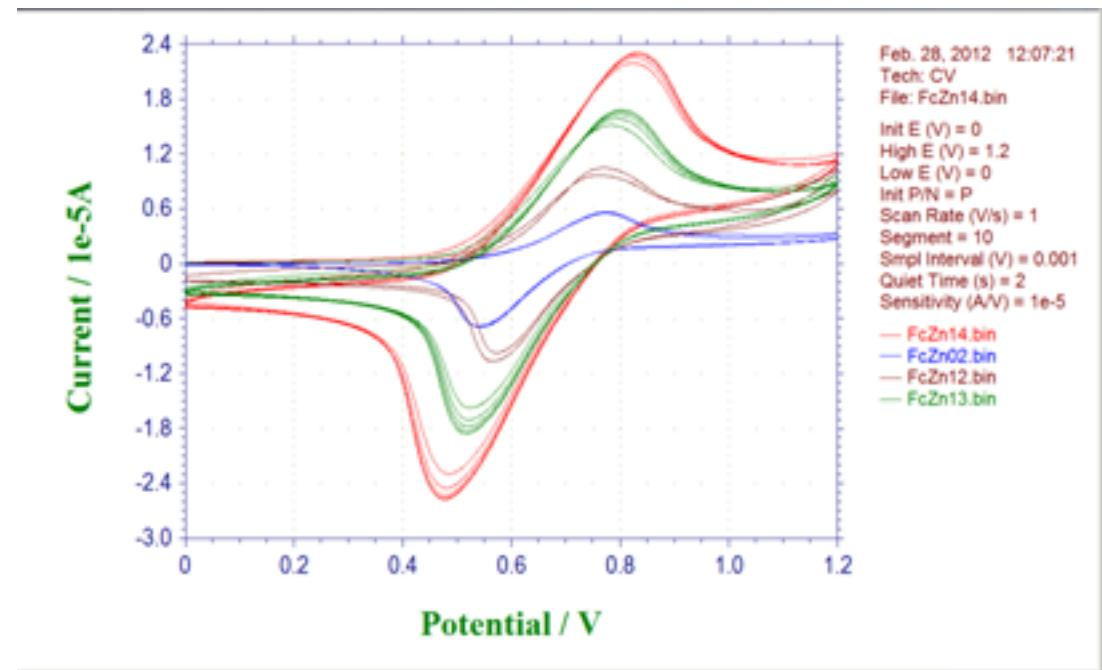
Solution phase voltammetry of 1 mM solution of **3** dissolved in THF containing 0.1 M TBAPF<sub>6</sub> using a 3 mm diameter platinum working electrode. The scan rates are 0.05, 0.2, 0.5 and 1.0 Vs<sup>-1</sup>.
