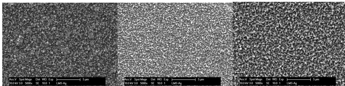
Figure S16: Silver deposits from  $[\text{Ag}(\text{MeIm})(\text{BuIm})][\text{Tf}_2\text{N}]$  on an Au working electrode at 90 °C for different current densities: 1  $\text{A dm}^{-2}$  (left), 5  $\text{A dm}^{-2}$  (centre), and 25  $\text{A dm}^{-2}$  (right). The theoretical thickness is 1  $\mu\text{m}$ .
