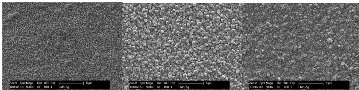
Figure S14: Silver deposits from  $[\text{Ag}(\text{BuIm})_2][\text{Tf}_2\text{N}]$  on an Au working electrode at 90 °C for different current densities: 1  $\text{A dm}^{-2}$  (left), 5  $\text{A dm}^{-2}$  (centre), and 25  $\text{A dm}^{-2}$  (right). The theoretical thickness is 1  $\mu\text{m}$ .
