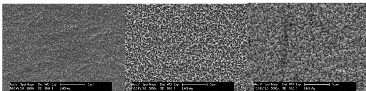
Figure S15: Silver deposits from  $[\text{Ag}(\text{EtIm})(\text{BuIm})][\text{Tf}_2\text{N}]$  on an Au working electrode at 90 °C for different current densities: 1  $\text{A dm}^{-2}$  (left), 5  $\text{A dm}^{-2}$  (centre), and 25  $\text{A dm}^{-2}$  (right). The theoretical thickness is 1  $\mu\text{m}$ .
