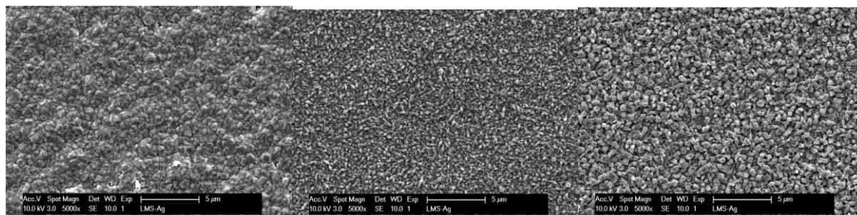
Figure S17: Silver deposits from  $[\text{Ag}(\text{MeIm})(\text{EtIm})][\text{Tf}_2\text{N}]$  on an Au working electrode at 90 °C for different current densities: 1  $\text{A dm}^{-2}$  (left), 5  $\text{A dm}^{-2}$  (centre), and 25  $\text{A dm}^{-2}$  (right). The theoretical thickness is 1  $\mu\text{m}$ .
