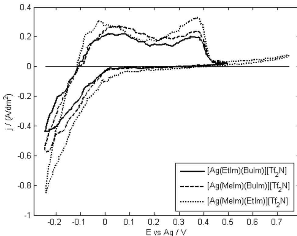
Figure S13: Cyclic voltammogram of  $[\text{Ag}(\text{MeIm})(\text{EtIm})][\text{Tf}_2\text{N}]$  (dotted line),  $[\text{Ag}(\text{MeIm})(\text{BuIm})][\text{Tf}_2\text{N}]$  (dashed line) and  $[\text{Ag}(\text{EtIm})(\text{BuIm})][\text{Tf}_2\text{N}]$  (solid line).
