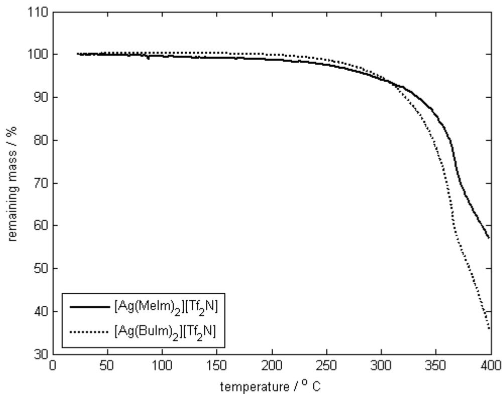
Figure S9: TGA of [Ag(MeIm)<sub>2</sub>][Tf<sub>2</sub>N] (solid line) and [Ag(BuIm)<sub>2</sub>][Tf<sub>2</sub>N] (dotted line).
