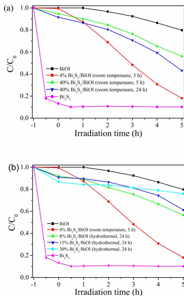
**Fig. S7.** Photocatalytic activities of (a) Bi<sub>2</sub>S<sub>3</sub>/BiOI with different ratios prepared at room temperature and (b)
