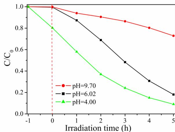
**Fig. S6.** The effect of pH values on photocatalytic activity of 4% Bi<sub>2</sub>S<sub>3</sub>/BiOI photocatalyst under visible light.
