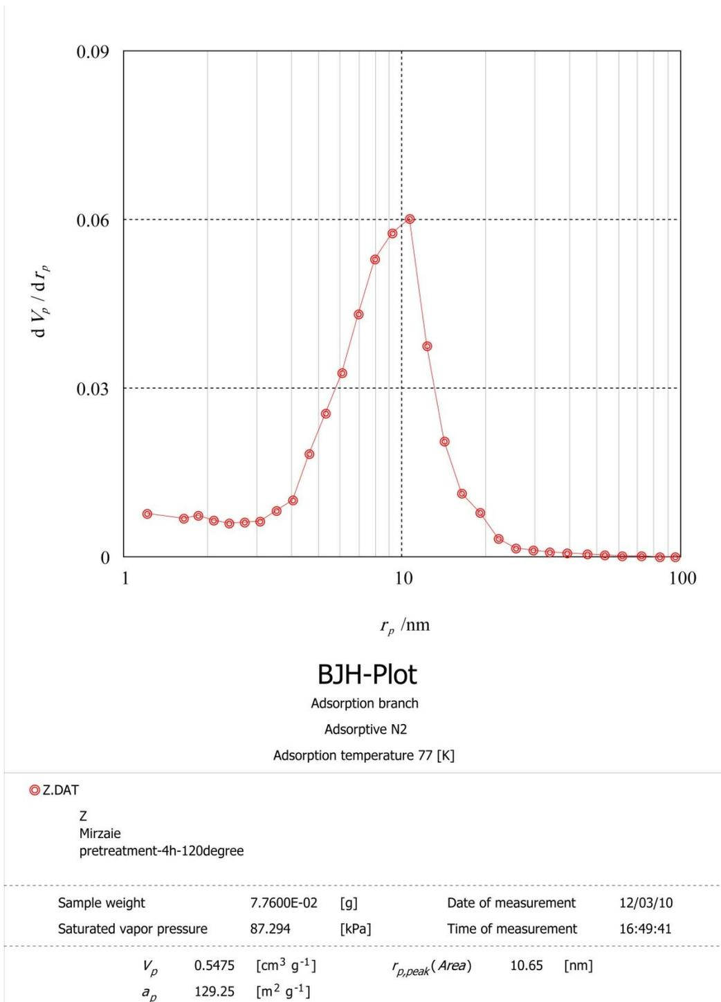
Fig. S3. BJH diagram for Faujasite zeolite
