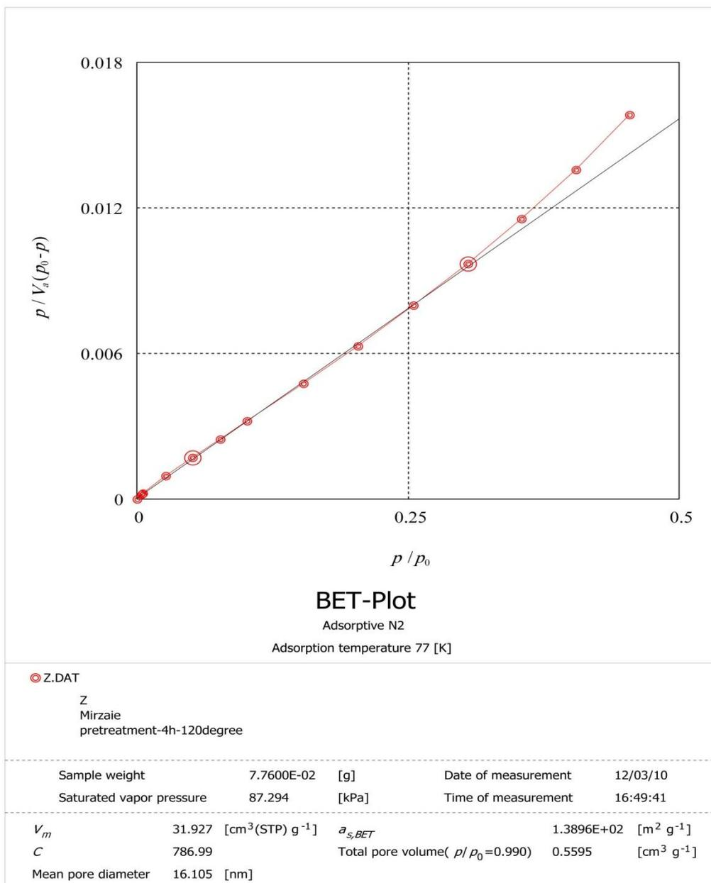
Fig. S2. BET diagram for Faujasite zeolite
