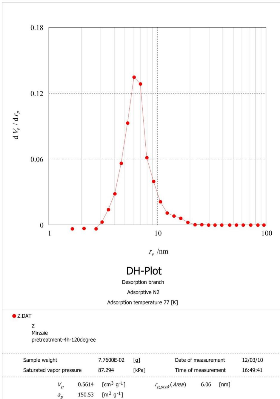
Fig. S4. DH diagram for Faujasite zeolite
