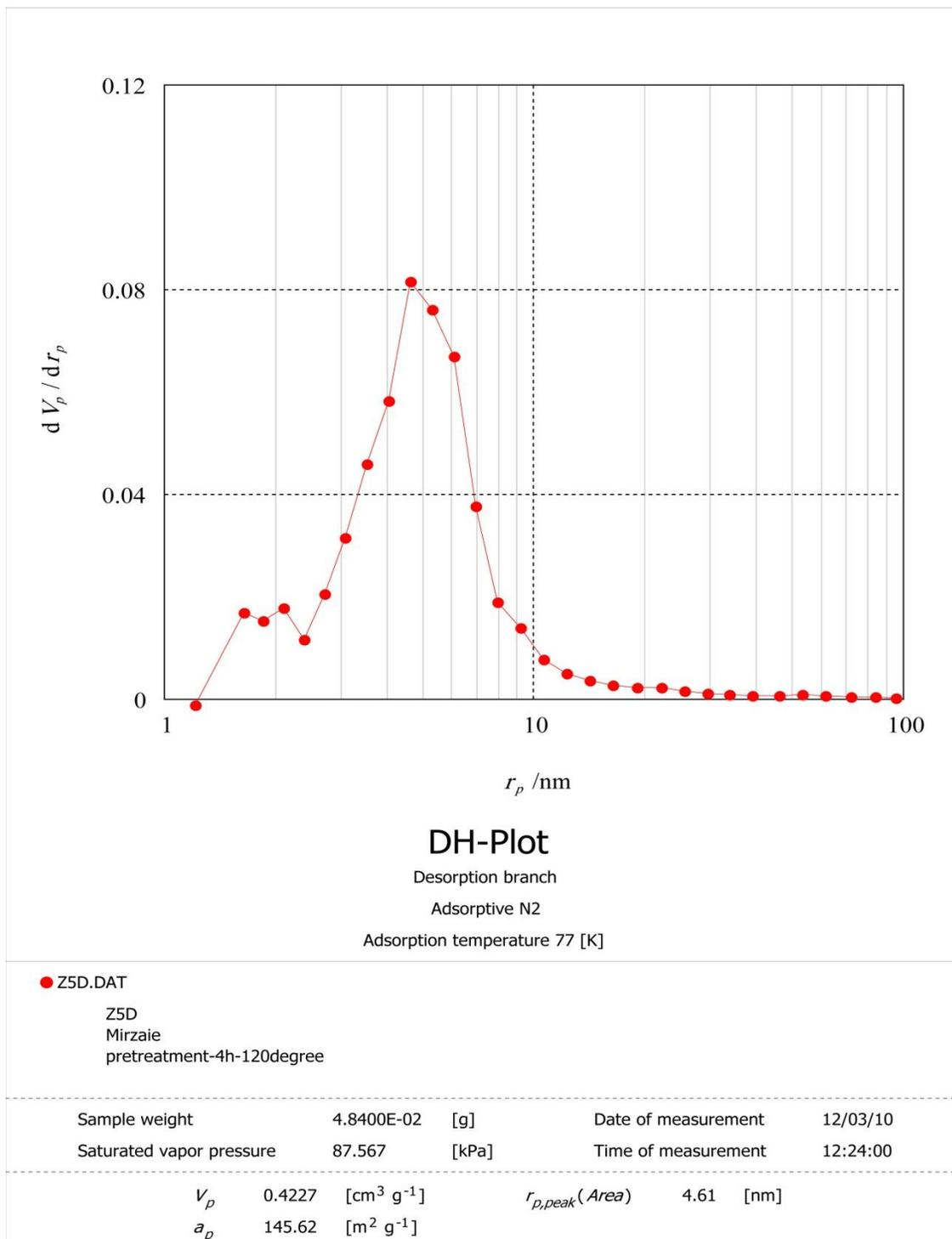
Fig. S8. DH diagram for manganese oxide within Faujasite zeolite
