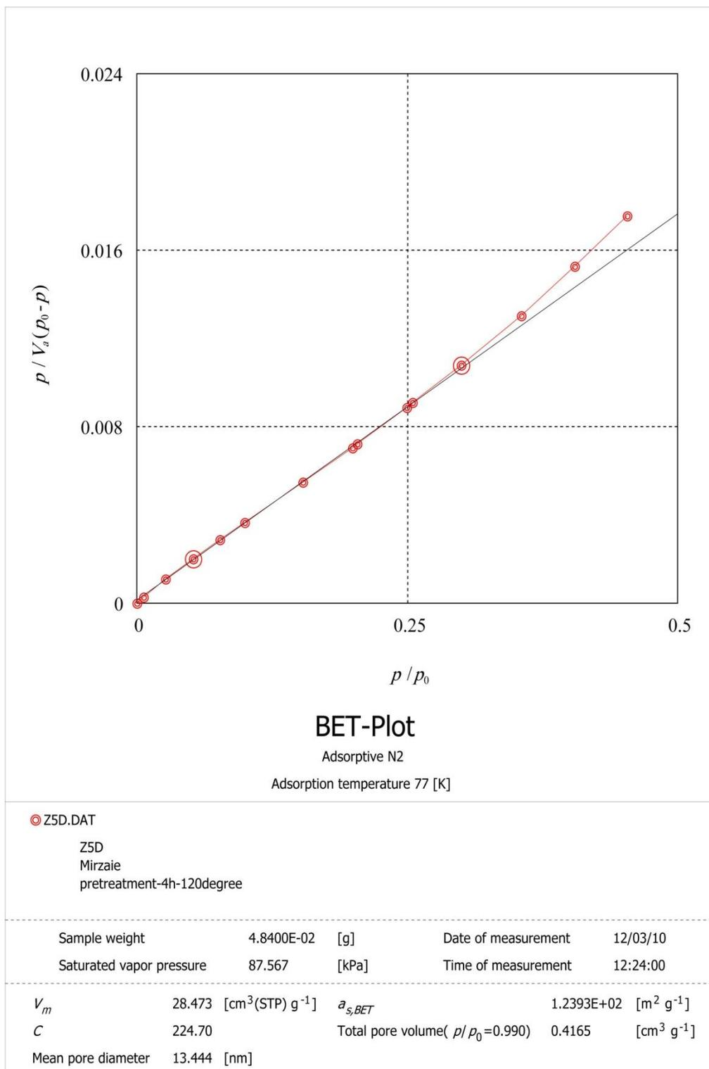
Fig. S6. BET diagram for manganese oxide within Faujasite zeolite
