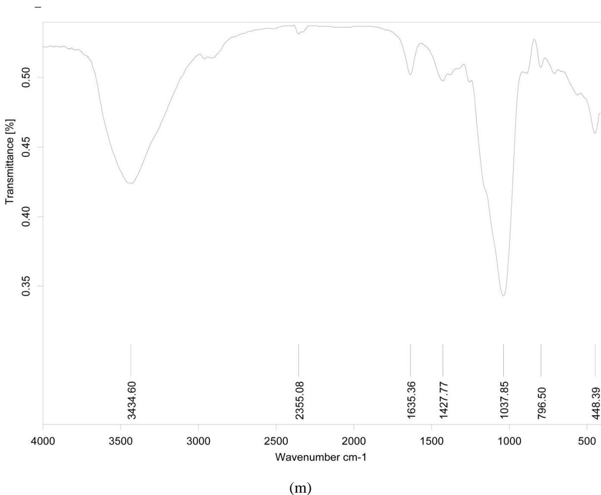
Fig. S10. IR spectra of the Manganese Oxides within Faujasite zeolite for Mn/Zeolite different ratios which that amount of zeolite constant. Contents of manganese in zeolite: a=0.1g, b=0.2g, c=0.3g, d=0.4g, e=0.5g, f=1g, g=2g, h=3g, i=4g, j=5g, k=7g, l=10g, m=Z5D (20g). In all IR spectra: 3420-3440, 1640, 1020-1030  $\text{cm}^{-1}$  are assigned to OH stretching,  $\text{H}_2\text{O}$  and the Si-O-(Al)Si vibrations.
