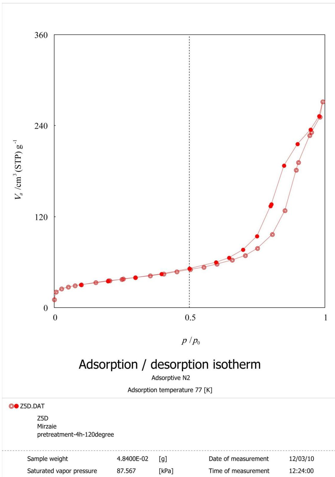
Fig. S9. Adsorption / Desorption Isotherm diagram for manganese oxide within Faujasite zeolite
