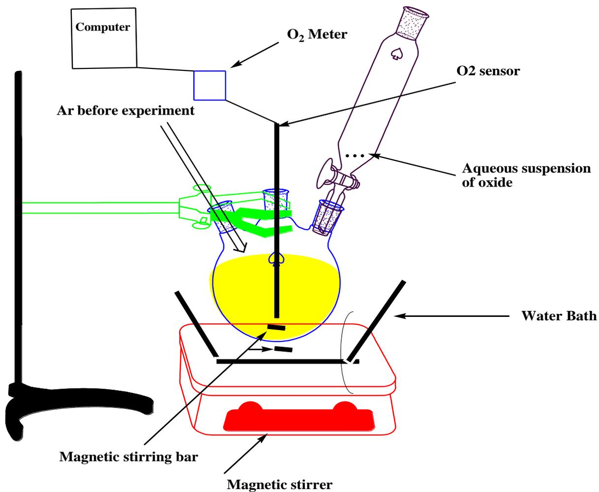
Fig. S1. The reactor set-up for oxygen evolution experiment from aqueous solution in the presence  $(\text{NH}_4)_2\text{Ce}(\text{NO}_3)_6$  (Ce(IV)) and manganese oxide within Faujasite zeolite.
