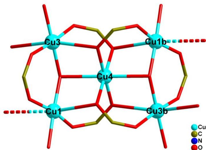
**Fig. S2** The pentanuclear copper(II) core in type II pentanuclear copper(II) cluster. Symmetry code:  $b, 1-x, 1-y, -1-z$ . Selected distances and angles are  $\text{Cu1}\cdots\text{Cu4}$  3.0816(5),  $\text{Cu3}\cdots\text{Cu4}$  3.1149(5),  $\text{Cu1}\cdots\text{Cu3}$  3.4640(8) and  $\text{Cu1}\cdots\text{Cu3b}$  5.1379(7) Å;  $\text{Cu1-Cu3-Cu1b}$  89.34 and  $\text{Cu3-Cu1-Cu3b}$  90.66°.
