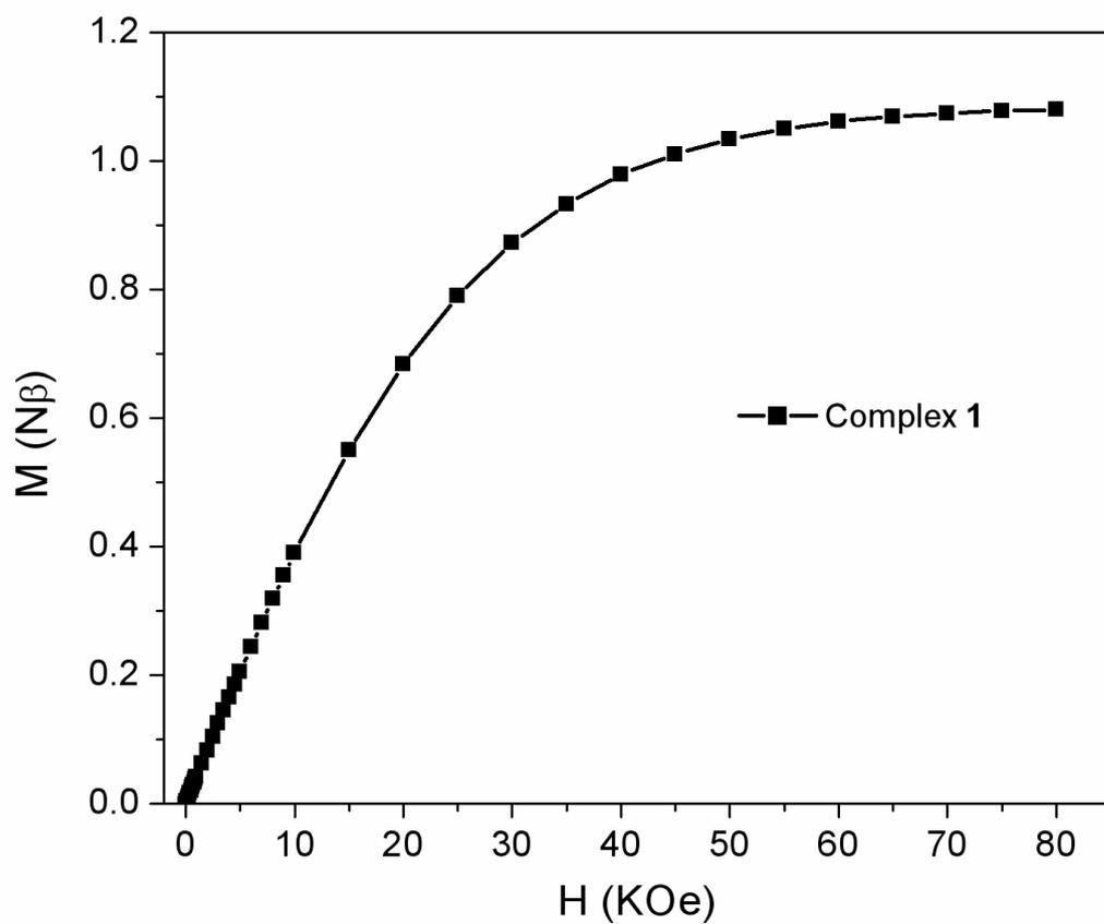
Fig. S4 The isothermal field-dependent magnetization plots for **1** at 2 K.
