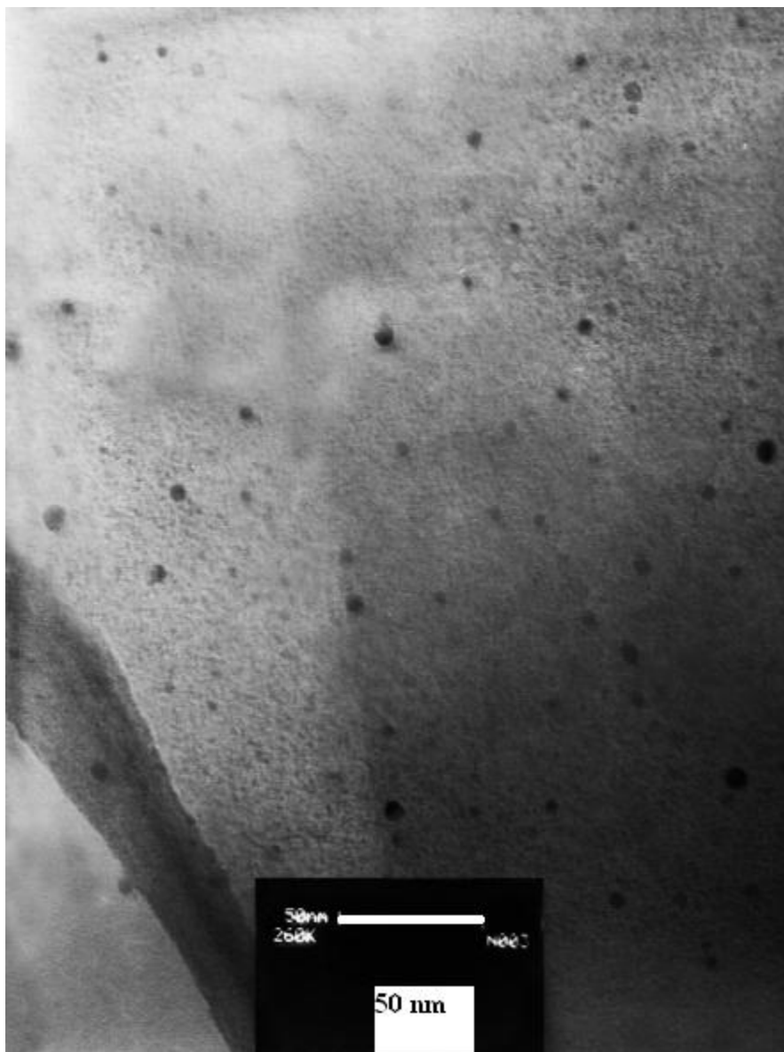
Fig. S7 TEM image of the centrifuged brown solid resulted from reacting of [(\text{bpy})_2\text{Mn}^{\text{III}}(\mu\text{-O})_2\text{Mn}^{\text{IV}}(\text{bpy})_2](\text{ClO}_4)_3 with Ce(IV).
