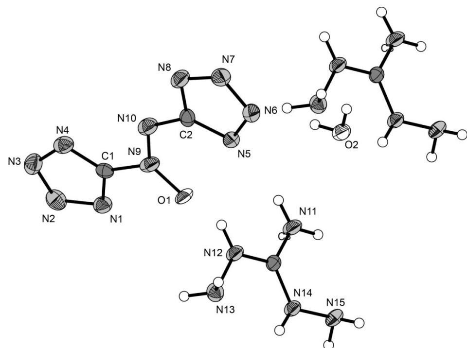
**Figure S2.** Molecular structure of bis(diaminoguanidinium) 5,5'-azoxybistetrazolate monohydrate (**5**). atom-labelling scheme and bond-distances (Å) with standard deviations. Thermal ellipsoids represent the 50 % probability level and hydrogen atoms are shown as small spheres of arbitrary radius.
