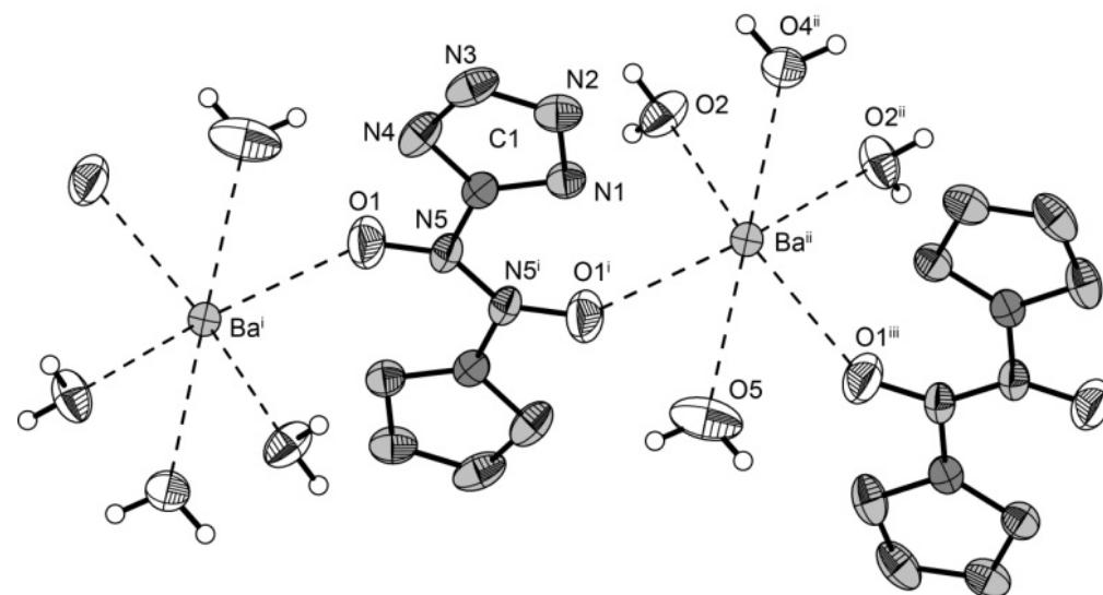
**Figure S1.** View on the formation of chains in the structure of barium 5,5'-azoxybistetrazolate tetrahydrate (**2**). Thermal ellipsoids represent the 50 % probability level and hydrogen atoms are shown as small spheres of arbitrary radius. Symmetry codes: (i) -x, 1-y, -z; (ii) x, 0.5-y, z; (iii) -x, -0.5+y, -z.
