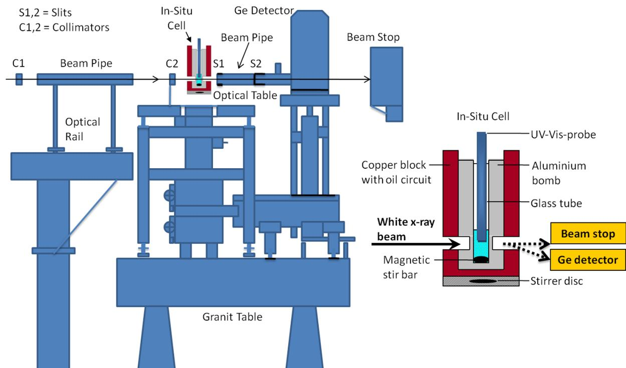
**Figure S3:** Detailed experimental setup of *in-situ* EDXRD reaction cell at the F3 beamline at HASYLAB, Hamburg, Germany.
