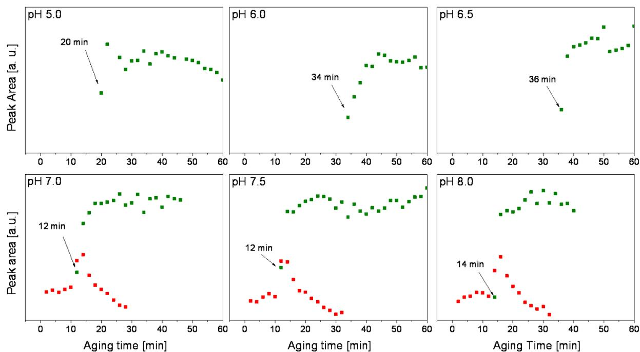
**Figure S7:** Integral intensity of selected EDXRD peaks of detected phases vs. aging time in  $\text{Na}_2\text{CO}_3$  at  $T = 333 \text{ K}$  at different pH-values. Zincian malachite  $(\text{Cu,Zn})_2(\text{OH})_2(\text{CO}_3)$  is represented by the  $20\bar{1}$  peak (green), sodium zinc carbonate  $\text{Na}_2\text{Zn}_3(\text{CO}_3)_4 \cdot 3\text{H}_2\text{O}$  is represented by the 222 peak (red).
