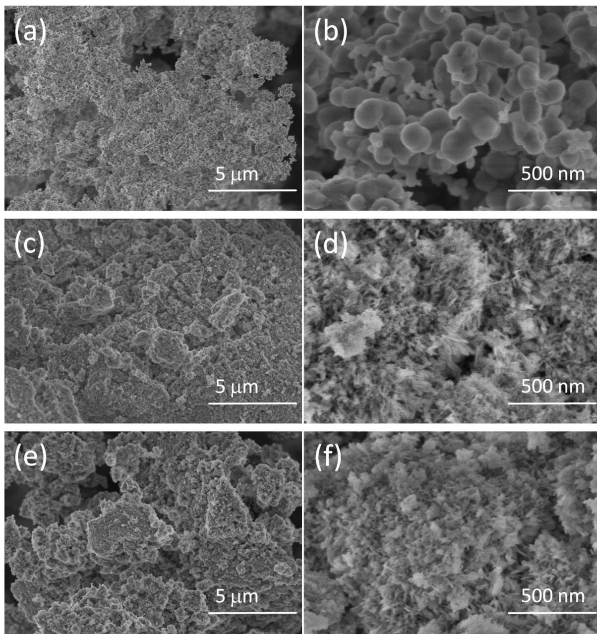
**Figure S5:** SEM images of unaged precursor, ID 0 (a,b) and aged precursors, ID 1 (c,d) and ID 6 (e,f).
