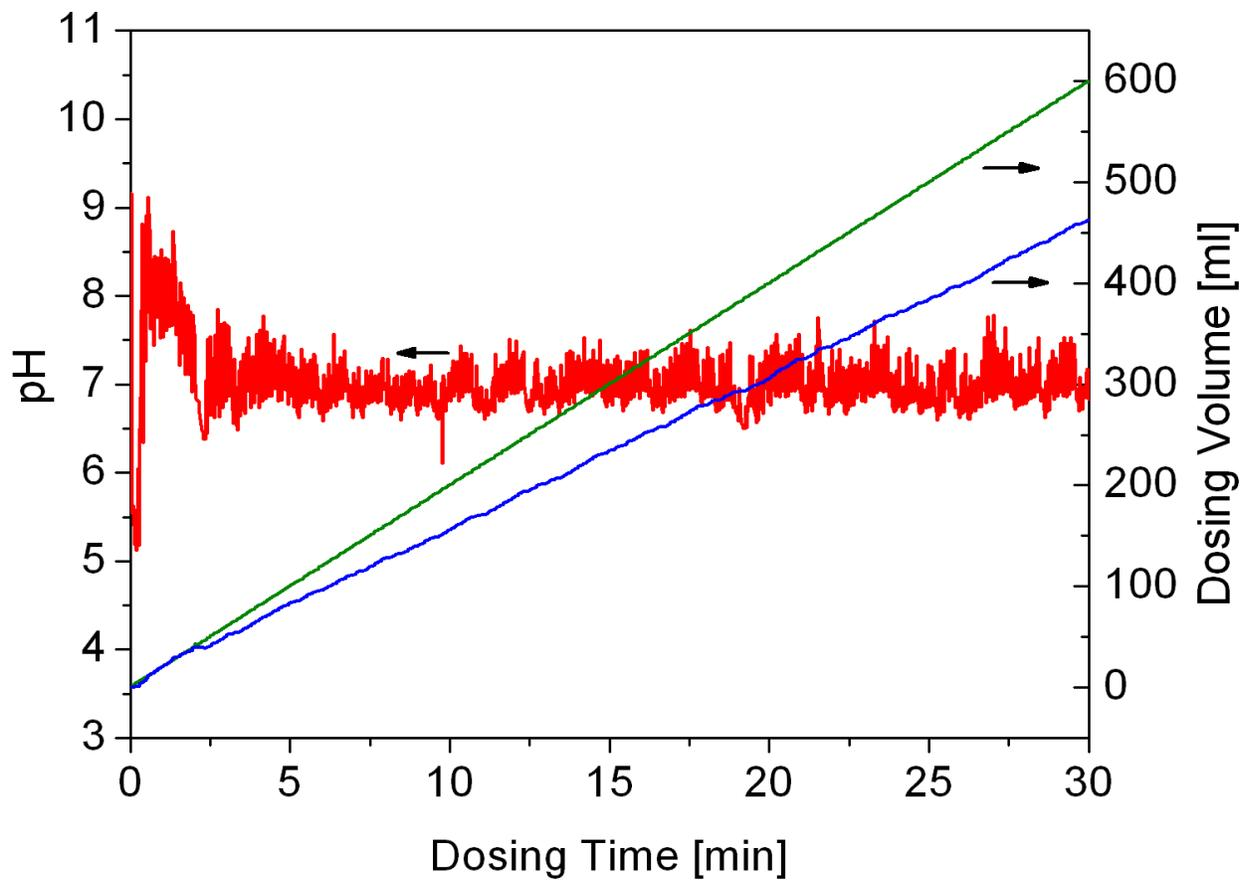
**Figure S1:** Evolution of pH (red curve) with added Cu,Zn solution (green curve) and Na<sub>2</sub>CO<sub>3</sub> solution (blue curve) during co-precipitation of the Cu,Zn (70:30) precursor in the continuous process. The slurry was continuously fed into a spray-dryer.
