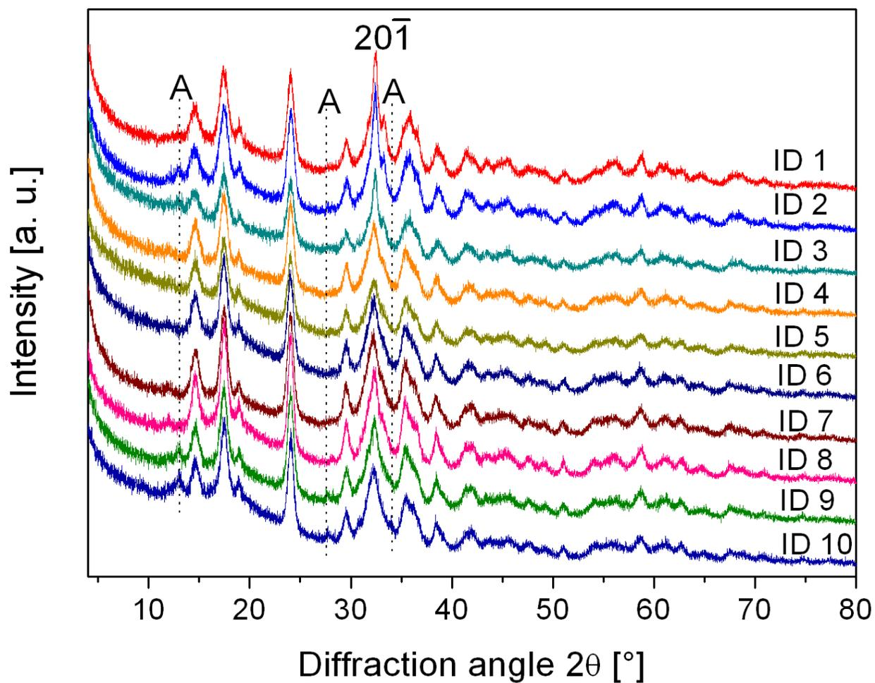
**Figure S4:** *Ex-situ* XRD patterns of all recovered sample (for labeling see Tab. 1). The  $20\bar{1}$  reflection of malachite and the characteristic peaks of aurichalcite are marked. The labeling refers to the entry number of Table 1 in the main article.
