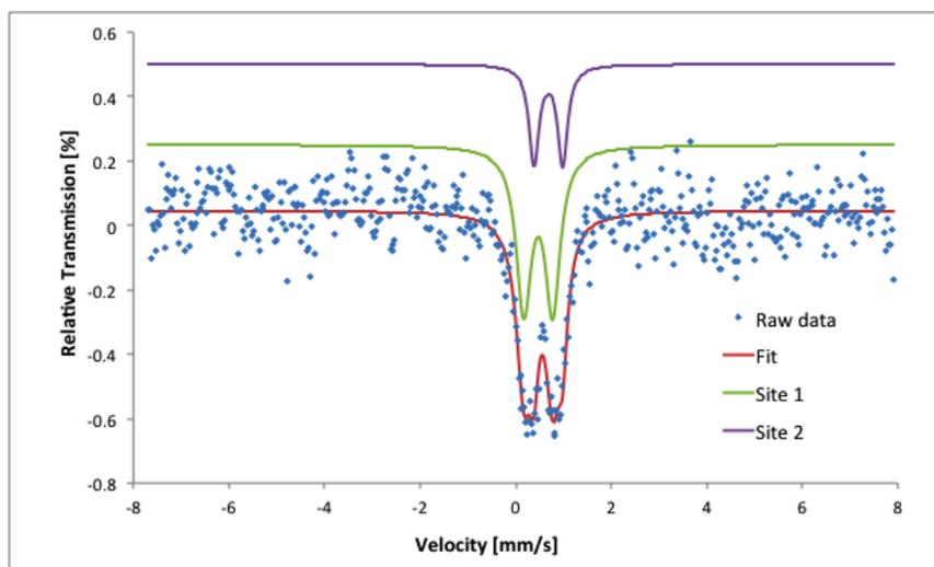
**Figure S1.** Zero-field  $^{57}\text{Fe}$  Mössbauer spectrum of complex **8** recorded at 77 K. Site 1 (71%):  $\delta = 0.472 \pm 0.02$  mm/s,  $\Delta E_q = 0.604 \pm 0.02$  mm/s; Site 2 (29%):  $\delta = 0.684 \pm 0.02$  mm/s,  $\Delta E_q = 0.600 \pm 0.02$  mm/s.
