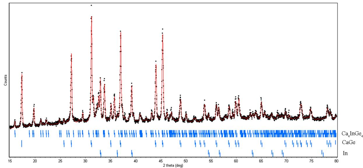
**Figure S1.** Measured and calculated powder X-ray diffraction pattern of  $\text{Ca}_4\text{InGe}_4$ . Peak positions are fitted using three phases:  $\text{Ca}_4\text{InGe}_4$ ,  $\text{CaGe}$ , and elemental In.
