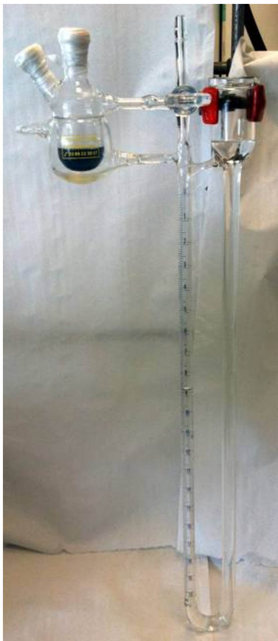
Figure 1. The volumetric glass vessel used in this study. The O 2 galvanometric probe was fixed to the top ground joint via a Teflon adaptor.
