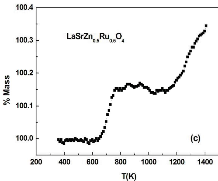
**FIG.S1** Thermogravimetric analysis (TGA) in air (a)  $\text{LaSrCo}_{0.5}\text{Ru}_{0.5}\text{O}_4$ , (b)  $\text{LaSrNi}_{0.5}\text{Ru}_{0.5}\text{O}_4$  and (c)  $\text{LaSrZn}_{0.5}\text{Ru}_{0.5}\text{O}_4$ .
