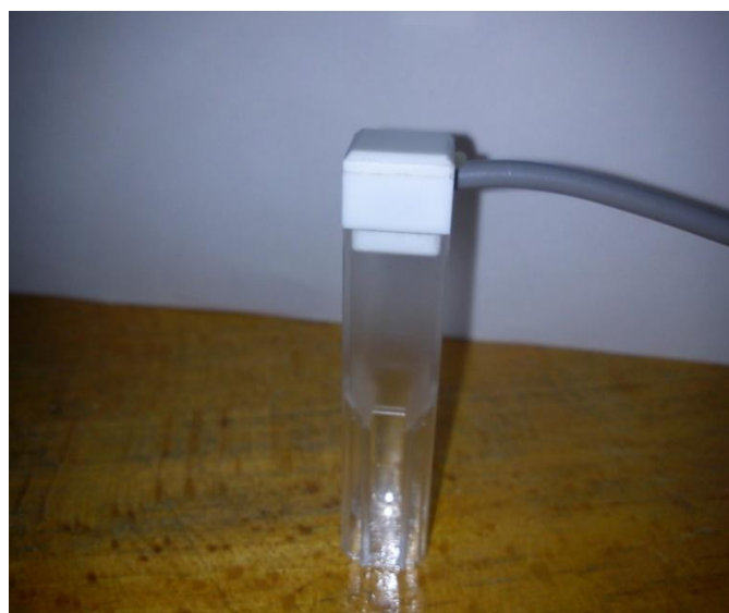
Figure 1 – An LED mounted on a special plastic cap fitted in to a PMMA cuvette.
