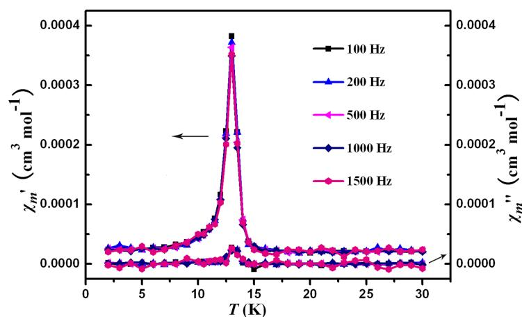
**Figure S5.** The in-phase  $\chi_m'$  and out-of-phase  $\chi_m''$  components of the ac susceptibility of **1** measured at different frequencies (100, 200, 500, 1000, 1500 Hz) in an applied ac field of 3 Oe.
