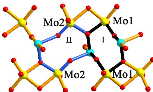
**Figure S7.** View of the magnetic Cu(II) centers bridged by oxygen atoms from two pathways:  $[\text{Mo}_1\text{O}_5]$  and  $[\text{Mo}_2\text{O}_5]$  polyhedra.
