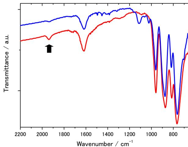
**Figure S1.** IR spectra of (blue line)  $[\text{GeW}_{11}\text{O}_{39}\text{Ru}^{\text{III}}(\text{dmsO})]^{5-}$  (**2**) and (red line)  $[\text{GeW}_{11}\text{O}_{39}\text{Ru}^{\text{III}}(\text{H}_2\text{O})]^{5-}$  (**1**). The black arrow indicates the peaks corresponding to the CO ligand bound to  $\text{Ru}^{\text{II}}$ .
