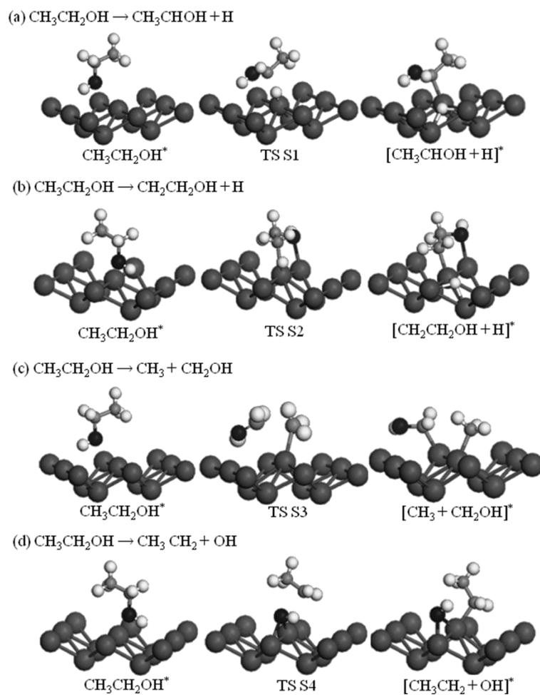
**Fig. S2** Reaction processes for the excluded steps relevant to short-bridge adsorbed *trans*-ethanol decomposition on Pd(110).
