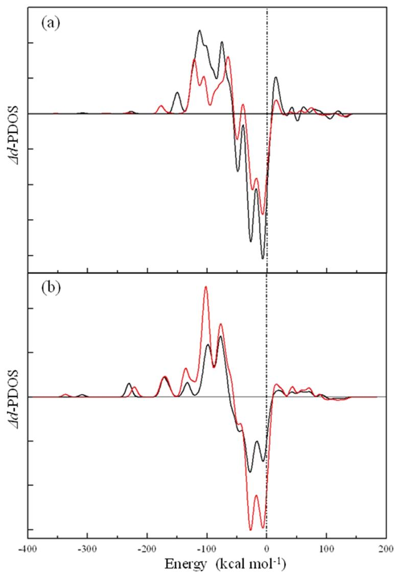
**Fig. S5** Variations of the  $d$ -projected density of states of surface Pd atoms due to bonding with TS complex in the competitive bond scission of  $\text{CH}_3\text{CH}_2\text{OH}$  and  $\text{CH}_3\text{CO}$  on Pd(111). (a) The black and red lines represent the O-H and C <sup>$\alpha$</sup> -H bond scission of ethanol. (b) The black and red lines represent the C-C and C-H bond scission of  $\text{CH}_3\text{CO}$ .
