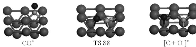
**Fig. S3** Reaction processes for the excluded steps relevant to  $\text{CH}_3\text{CH}_2\text{O}$  decomposition and  $\text{CO}$  dissociation on  $\text{Pd}(110)$ .
