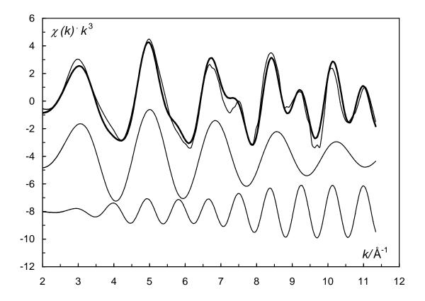
**Figure S3.** The fit and the individual contribution of the different scattering paths of the EXAFS data of colloidal plutonium(IV) oxide, stored for five years. Solid thin line - experimental data, thick line - calculated model function using the parameters given in Table 1. Individual contributions: solid line (offset - -3) - Pu-O single scattering (SS) (offset - -8) and Pu--Pu SS (offset - -7).
