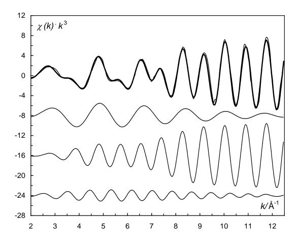
**Figure S2.** The fit and the individual contribution of the different scattering paths of the EXAFS data of colloidal plutonium(IV) oxide, freshly prepared. Solid thin line - experimental data, thick line - calculated model function using the parameters given in Table 1. Individual contributions: solid line (offset - -4) - Pu-O single scattering (SS) (offset - -8) and Pu--Pu SS (offset - -8).
