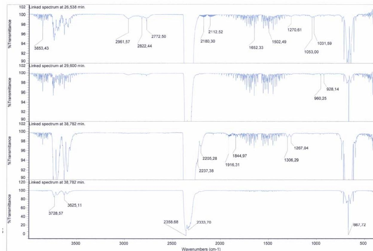
e) Sheet with FT-IR spectra from pure samples of the evolved gases, for identification purposes.
