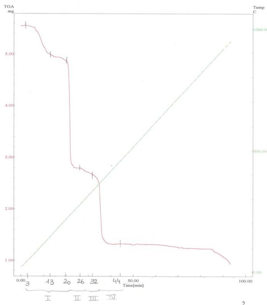
b) The TG-plot of compound **8** with weight loss as a function of the temperature (bottom axis)
